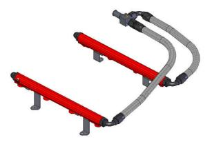
25. Connect one AN-08 90-Degree hose end to the rear of each fuel rail. Plan a route for each of the two lines between the fuel pressure regulator and the fuel rails, measure the two lengths of fuel line needed. See section titled Hose and Fitting Assembly for fuel line assembly instructions. Once the hoses are assembled, **ensure there is no debris in the hose** and install them.
