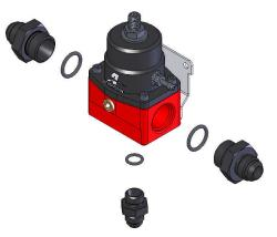
20. Install one ORB-08 o-ring on each of the two p/n 15607 ORB-08/AN-08 cutoff tapered flare fittings.
