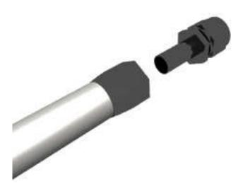
G. Using a properly sized wrench, complete threading the two components together (The maximum allowable gap between the two fitting components is .030 inches).
