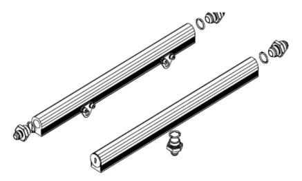
32. Inspect the o-rings on the OEM quick disconnect fitting and replace if necessary. Coat o-rings and the adapter fitting with a light oil and install the 15101 AN-06 Ford quick disconnect adapter fitting on the OEM return fuel line.
