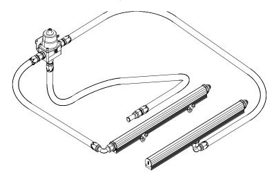
36. Inspect the OEM fuel supply line o-rings and replace if necessary. Place a light coat of oil on the fuel supply line o-rings and the supply line adapter fitting to ease installation. Connect the 15103 AN-08 tee adapter fitting to the OEM quick connect on the fuel supply line.
