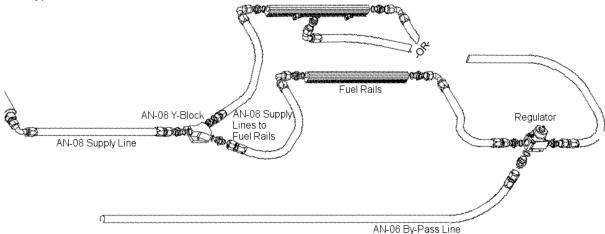
26. If you intend to retain the factory feed and return lines, Aeromotive offers the 14102 fuel rail system, including the 15101 and 15102 fuel line adapters.
