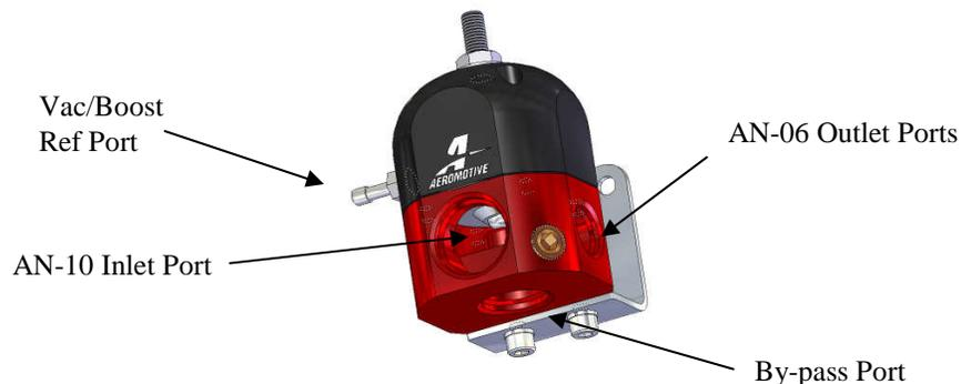
5. Attach the fuel supply line to the AN-10 inlet port located in the front of the regulator using a cutoff AN-10 style fitting (Aeromotive P/N 15608 or equivalent) and o-rings.
