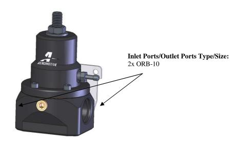
7. Attach the fuel return line to the ORB-10 bypass port located at the bottom of the regulator using a ORB-10 to AN-10 port fitting (Aeromotive P/N 15608 or equivalent) and o-ring.
