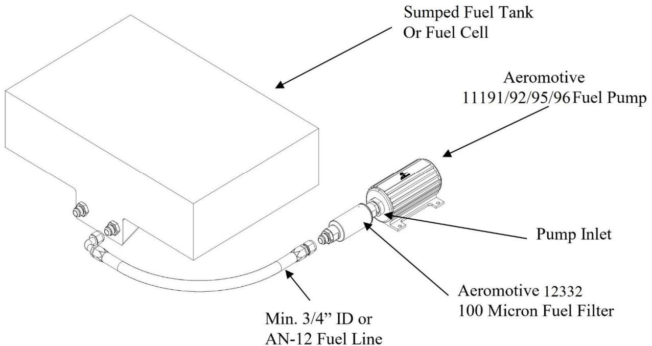
7. Using AN-12 fuel line, connect the fuel pump outlet to a 10 micron post fuel filter (Aeromotive P/N 12339). You can attach the filter directly to the fuel pump utilizing an ORB-10 to AN-12 fitting (Aeromotive P/N 15642) and 2 sealing o-rings (AN-10 o-ring pack Aeromotive P/N 15623, AN-12 o-ring pack Aeromotive P/N 15624). **Make sure you use high pressure (150 psi minimum) fuel line for this connection!**
