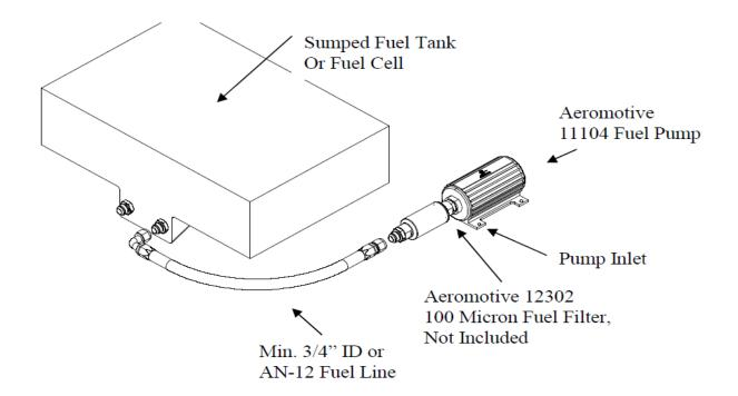
Note: If you would like a fuel shut off valve installed between the fuel tank outlet and the fuel pump. Use Aeromotive part # 12332 shutoff valve fuel filter in place of the 12302 fuel filter.
