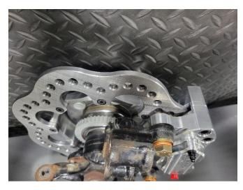
\*Drop the pads into the calipers with the friction side facing the rotor and secure them with the pad retaining bolt and ny-lock nut. Be sure the bolt extends through the locking feature of the nut and tighten until you can barely spin the pad bolt with your fingers. Make sure the brake pads are the only thing touching the rotor! The rotor should be centered in the caliper.
