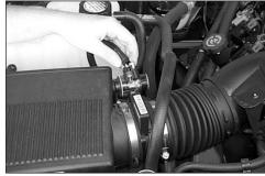
2. Disconnect the mass air sensor electrician connection.
