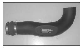
11. Install the silicone hump hose (08176) and hose clamps onto the K&N intake tube as shown.
