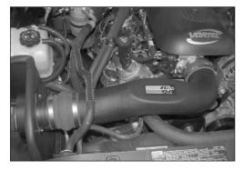
12. Install the K&N intake tube onto the mass air sensor, then secure the other end onto the throttle body as shown.
