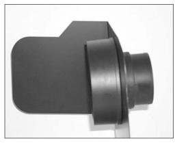
7. Assemble the mass air adapter, heat shield, gaskets and the mass air sensor as shown above.
