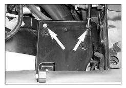
5. Loosen and remove the two air cleaner mounting tray bolts as shown. NOTE: K&N recommends that you do not discard your factory air intake.
