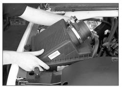
4) Pull firmly upwards to release the air cleaner assembly from the mounting tray grommets, then remove the assembly.
