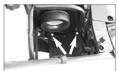
9. Install and mount the heat shield assembly to the air cleaner mounting tray
