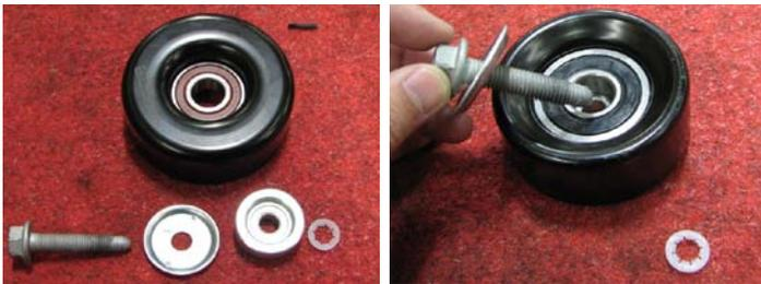
72. Apply Loctite to the threads on both idler pulley bolts. Then use a 15mm socket to install the 76mm idler pulley with the factory hardware to the left idler pulley location. Install the additional idler pulley to the right idler pulley location with the M8 x 20mm bolt and M8 washer from Bag #1. Torque both pulley bolts to 18 ft-lbs. Verify that both pulleys spin freely.
