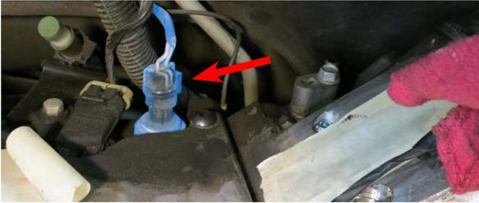
30. Using a 8mm Allen wrench, remove the factory plug towards the front driver side of the block, adjacent to the crank pulley. Apply thread sealant w/ PTFE to the threads of the factory oil pressure sensor and install the sensor in the location of the plug. Torque to 26 ft/lbs (35 Nm).
