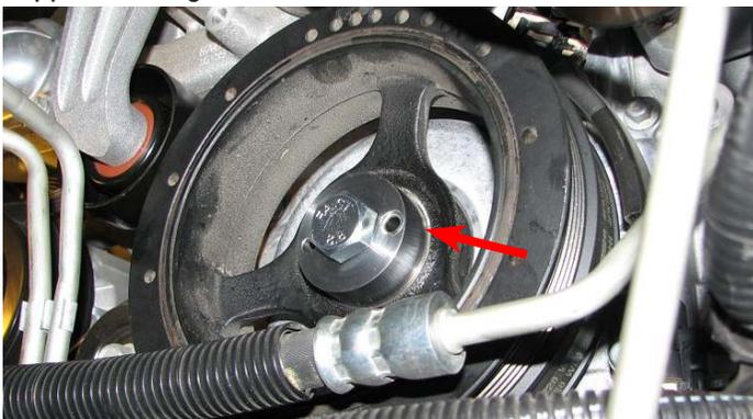
17. Measure 1.7" from the tip of the 15/64" drill bit supplied in Bag #4 and mark the position with a piece of masking tape. Lubricate the drill bit with a small amount of engine oil. Then locate the guide hole with the drilling bushing. Begin drilling using a Right Angle Drill (or equivalent) and the supplied 15/64" drill bit. The drilling process is complete when the tape mark on the bit meets the guide.
