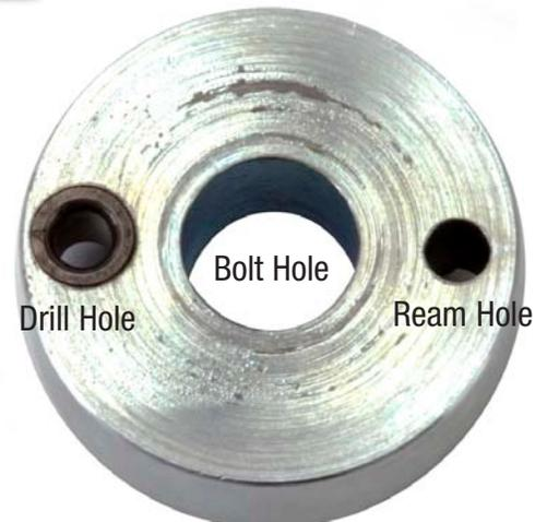
(1x) - Crank Pinning Drill Guide
