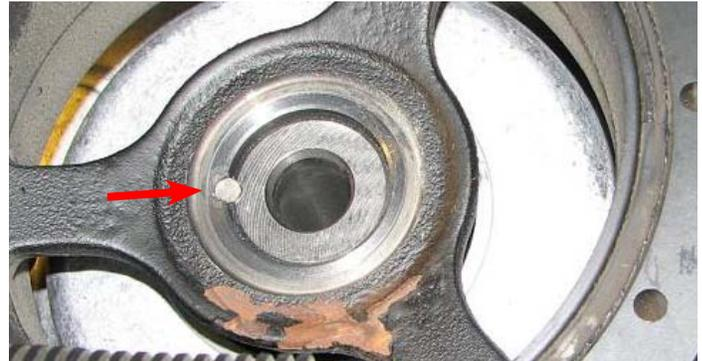
21. Install the crank bolt supplied in Bag #4 and torque it to 37 ft-lbs then rotate it an additional 140°.
