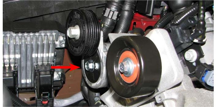
68. Use a 12mm socket and an M8 x 20mm bolt supplied in Bag #1 to secure the ground strap to the back side of the tensioner bracket.
