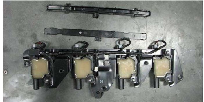
48. Tuck any loose wiring under each coil bracket then use a 10mm socket and the ten stock bolts to install the coil brackets on to each valve cover.
