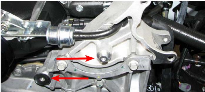
73. Route the serpentine belt (*not included*) using the diagram below. Use a 15mm socket to release tension from the tensioner and re-tension after the belt is routed. Proceed to Step 74.
