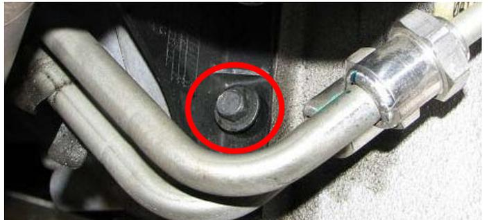
9. Use a 13mm socket to remove the two starter bolts.
