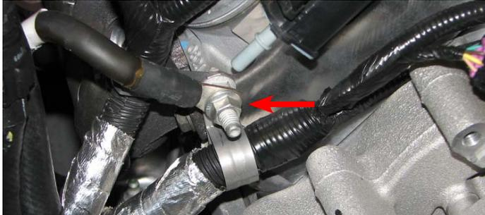
65. Install the supplied tensioner bracket to the water pump using the spacers from bag #6, three M10 x 65mm bolts from bag #1, and blue Loctite. The two short spacers go onto the two provisions on the water pump with two 65mm hex flange bolts, and the long spacer goes on the cylinder head provision with the 65mm socket head bolt.
