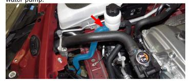
105. Using one (1) 3/4" Hose clamp form Bag #2, secure the surge tank to water pump hose (highlighted blue) to the water pump. Attach convoluted tubing (highlighted red) on the hose where it makes contact with metal or sharp surfaces and secure with zip ties or electrical tape.
