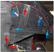
7. Using A 10mm socket, panel puller and Phillips Head Screwdriver, remove the eight (8) bolts, two (2) screws and two (2) push pins securing the under tray.
