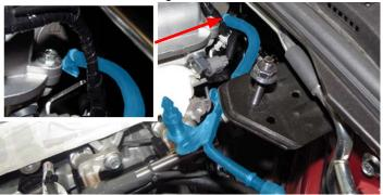
46. Install the provided fuel line by pushing the female end onto the factory quick connect fitting. Tuck the new fuel line against the fire wall as shown.
