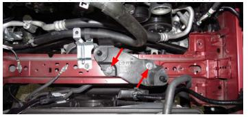
49. Using a 10mm socket, remove the bolt securing the cooling hose bracket to the frame. The bracket can be left attached to the hose. This will make removal/installation of the belt easier.
