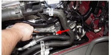
51. Remove the four (4) intake 0-ring gaskets from the factory manifold and trim off the small tab on each gasket.
