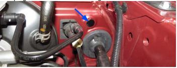
20. Using a 10mm socket, remove the bolt securing the lower portion of the airbox to the frame and remove the airbox. The air inlet tube on the left will remain in place.
