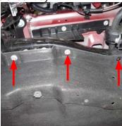
On both driver and passenger sides, disconnect the side marker and fog light harness connectors from the light fixtures. Using a panel puller, remove the anchors securing
