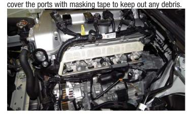
44. Using a 13mm socket, remove the bolt securing the engine hoist bracket to the driver side of the cylinder head. **Optional:** Using the provided M10 x 16mm bolt in Bag #3, transfer the engine hoist bracket to the provision on the passenger side front of the cylinder head.
