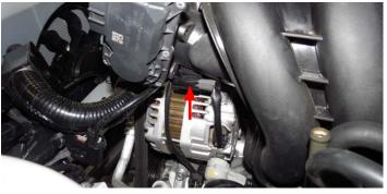
40. Lift up the front of the intake manifold and remove the anchor securing the engine harness to the intake manifold. **NOTE:** *This pin will be located just behind the alternator.*
