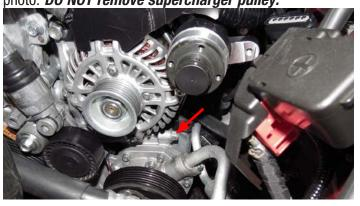
83. Using the 120mm hex head bolt from Bag #1, loosely install the supplied idler bracket onto the A/C compressor. Orient the bracket so the idler boss is facing forward and closest to the A/C pulley.
