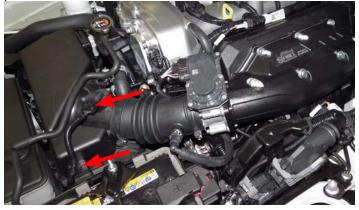
137. Locate the 3' section of hose attached to the supercharger inlet during step 72. Lubricate the brake booster check valve with silicone lube and insert the **tapered end into the hose first**. Push the remaining potion of the check valve into the hose so it sits just below the hose end.
