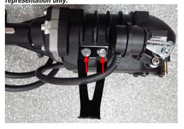
78. Access the lower mounting bracket bolt through the drive side wheel well and tighten the bolt to 16 lb/ft.
