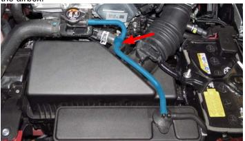
WARNING! Steps 136 to 138 are for installing the brake booster check valve. These steps must be followed correctly or braking performance will be severely compromised.
