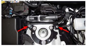
122. Install the EVAP mounting bracket onto the ECM mounting stud closest to the firewall and loosely secure with the factory nut. Attach the EVAP solenoid to the bracket using the factory bolt removed during step 30. Tighten both the nut and bolt.
