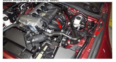
18. If equipped, remove the sound tube and intake tube assembly by disengaging the locking tabs from the fire wall mounting hole. **NOTE:** There are two locking tabs on each side of the sound tube recessed in the fire wall. These tabs can be released by carefully inserting a flat head screwdriver on the sides of the tube to release the tabs.
