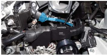
113. Install the throttle body extension harness onto the factory throttle body connector. Tuck the factory end under the MAP sensor and route the harness to the front of the valve cover as shown.
