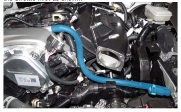
115. Apply silicone lubricant to the provided throttle body 0-ring and install the 0-ring into the groove on the supercharger inlet.
