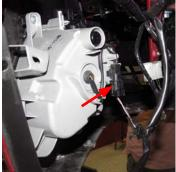
Using a 10mm socket or Phillips Head Screwdriver, remove the two (2) bolts securing the from fascia to the fender (one on each side of the vehicle).
