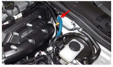
139. Route the EVAP connector on the water pump harness to the EVAP solenoid and connect as shown. Attach the harness to existing harnesses and secure with zip ties or electrical tape.
