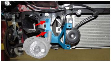
92. Remove the two (2) inside bolts securing the driver side crash beam to the frame. Install the driver side LTR bracket on top of the crash beam mounting points and reinstall the bolts.
