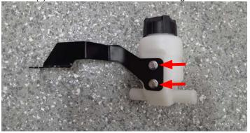
89. Using a 10mm socket, remove the two (2) nuts securing the factory harness connection to the passenger side strut tower. Secure the surge tank bracket to the
