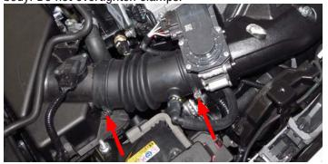
factory intake manifold. Also remove the indicated clamp.
