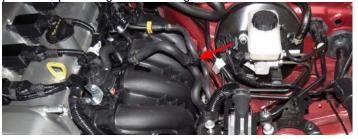
27. Using hose clamp pliers, remove the EVAP hose from the hard line.
