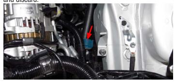
56. Using pliers, bend the top portion of the harness retaining bracket so it is oriented straight up.
