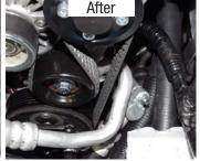
88. Install the surge tank onto the surge tank bracket using the two (2) M6 x 10mm bolts located in Bag #2.
