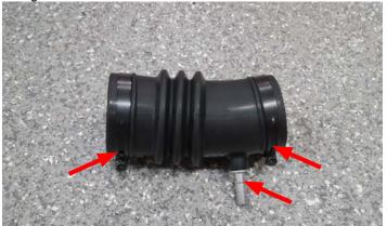
129. Install the new intake tube assembly onto the factory airbox lid in the orientation shown below. Do not tighten the clamp on the lid.
