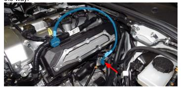
69. Using the one (1) M8 x 20mm bolt from bag #3, loosely install the supercharger support bracket onto the engine block above the drive side engine mount. **NOTE:** *The bracket should be rotated toward the alternator so to rests against the engine mount.*
