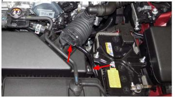
15. Disengage the two (2) clips retaining the airbox lid and loosen the clamp securing the rubber intake tube to the lid. Remove the lid and air filter and set aside.
