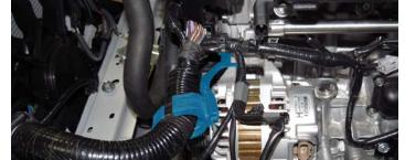
72. Using two (2) 5/8" hose clamps from Bag #2, connect the 2' section of 3/8" hose to the front fitting on the supercharger assembly. This hose will connect to the EVAP solenoid later. Connect the 3' section of hose to the rear fitting. This hose will connect to the brake booster later.
