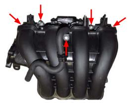
39. Using a panel puller, remove the anchor securing the alternator harness to the intake manifold.
