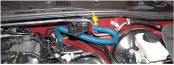
30. Remove the EVAP solenoid from the intake manifold by disconnecting the harness connector from the solenoid and removing the 8mm bolt securing the bracket to the solenoid. Remove the solenoid off the manifold as well as the rubber hose that connects to the manifold.
