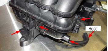
43. Remove the intake manifold and set aside. Using a lint
