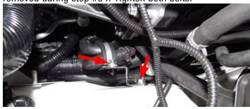
66. Attach convoluted tubing around the hoses installed in steps 57 and 58 in areas that make contact with sharp edges. Secure the convoluted tubing with zip ties or electrical tape.
