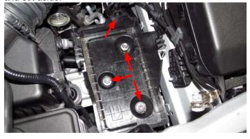
Using a panel puller and Phillips head screwdriver, remove the four (4) push pins and two (2) screws securing the radiator cover to the frame.
