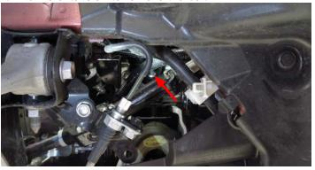
26. Separate the EVAP line and Fuel line by prying apart the plastic clip holding the lines together.
