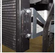
97. Tighten the passenger side radiator shroud bolt left loose in step 95. **TIP:** *This bolt can be reached from the back side of the LTR using a 10mm wrench.*
