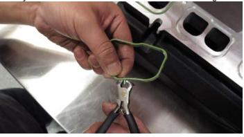
52. Apply silicone lubricant to the modified 0-ring gaskets then insert the gaskets into the supercharger runner as shown.
