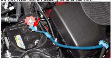
142. Using zip ties, secure all water pump harness wires away from any moving parts or potentially hot surfaces. Secure the water pump fuse holder inside the fuse box next to the battery as shown below and reinstall the lid.
