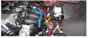
28. Stuff shop rags under the fuel line to catch any spilt fuel and disconnect the line by pulling up on the yellow locking tab.
