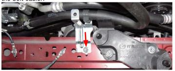
50. Using a 17mm wrench, slowly release the tension on the main drive belt and remove the belt. The wrench should be rotated counter clockwise to compress the tensioner.
