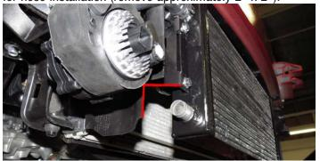
103. Using three (3) 3/4" clamps and one (1) straight connector from Bag #2, install the hose (highlighted blue) from the bottom fitting on the LTR to the hose end labeled "Z". Attach convoluted tubing (highlighted red) on the hose where it makes contact with metal or sharp surfaces and secure with zip ties or electrical tape. **NOTE:** Zip Tie the hose to the two (2) ears on each side of the steering rack to hold it in place.
