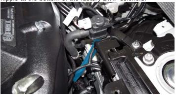
118. Remove the EVAP hose from the factory intake manifold and orient as shown below. Cut the hose as far away from the 90° bend as possible but before the next bend starts as indicated by the red line.
