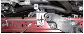
127. Using the factory hardware, reinstall the lower portion of the airbox and insert the provided K&N high flow filter in place of the factory paper filter.
