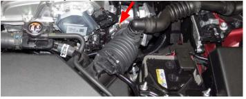
17. If equipped, use a 10mm socket to remove the two (2) bolts securing the sound tube.
