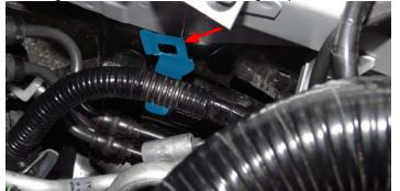
©2018 Edelbrock LLC Part #1554, 15540 57. Position the hose labeled "IC" into the engine bay so that the hose routes under the clutch line (if equipped), engine harness, A/C line and front sway bar.
