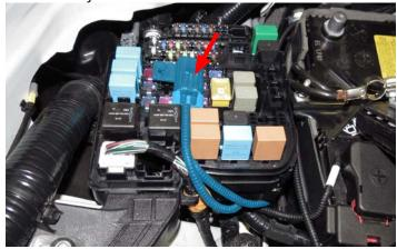
143. Reconnect the four (4) coil harness connections and one (1) fuel pump harness connection at the back of the engine.
