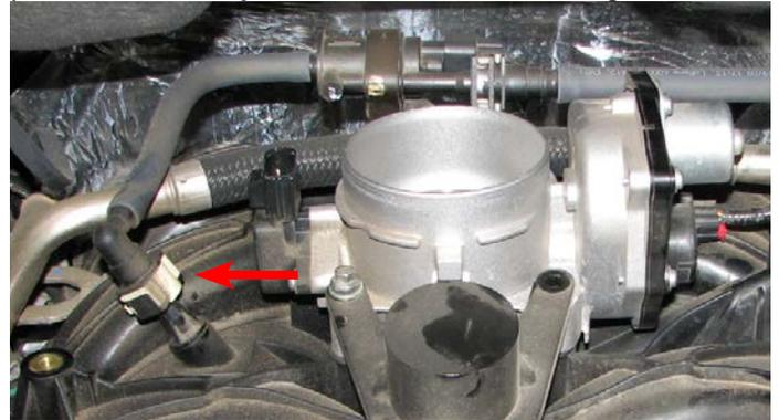
16. Disconnect the fuel inlet hose from the fuel rails by sliding off the lock clip and depressing the blue tab. Use a shop rag to absorb any excess fuel.
