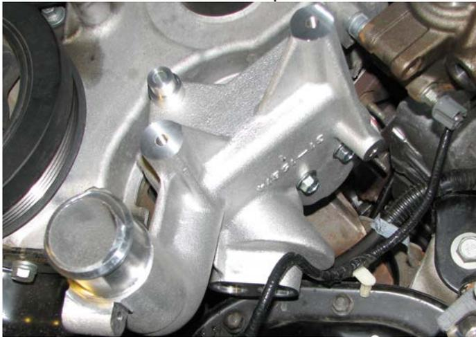
73. Use the (2) M8 x 75mm long bolts from Bag #3 to hold the gasket in place while aligning the flange of the supplied oil filter bracket to the block. Finger tighten these bolts until the bracket is flush to the block
