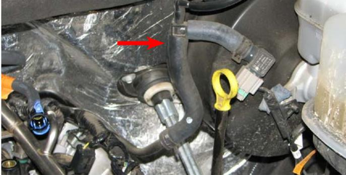
20. Insert a 1/2" drive breaker bar into the square hole of the belt tensioner. Push the breaker bar towards the driver side fender then remove the serpentine belt.
