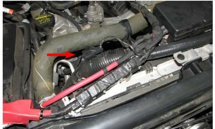
26. Use a 10mm socket and a short extension bar to remove the ten intake manifold bolts then lift and remove the intake manifold.
