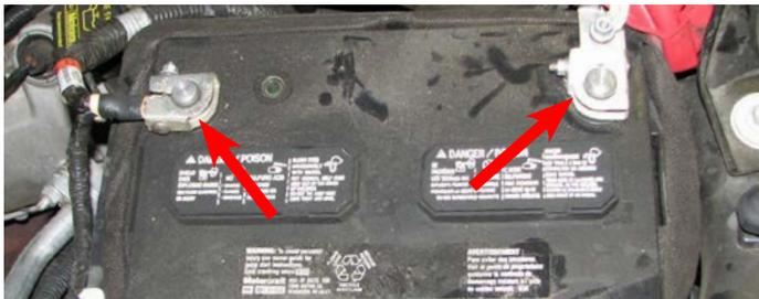
3. Use an 8mm socket to loosen and remove the positive battery terminal clamp, then tuck the wire aside.
