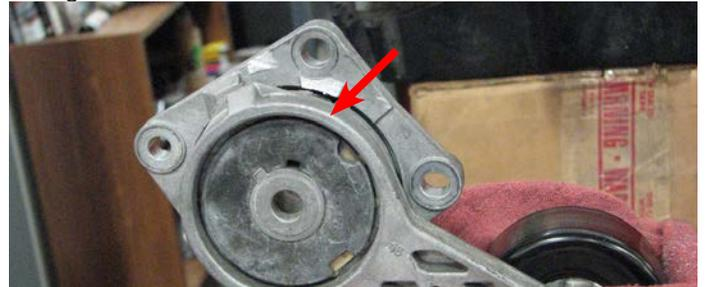
97. Align the two pieces of the tensioner brace so that the bolt holes line up and the script is facing out then install the three M6 x 25mm bolts supplied with the brace.
