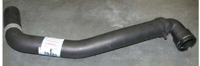
84. Install the lower radiator hose between the oil filter bracket and the radiator. Secure the hose to the bracket with the stock hose clamp then secure the elbow fitting to the radiator by reinserting the stock wire clip.
