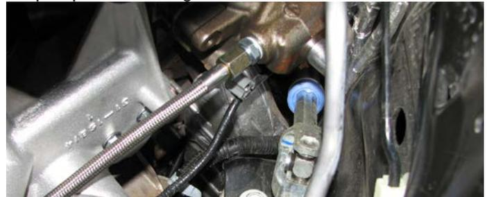
78. Route the power steering hose along the crossmember and back to the power steering rack. Secure it to the crossmember with the stock bolt. Use the supplied wire ties to isolate the hose away from any moving parts.
