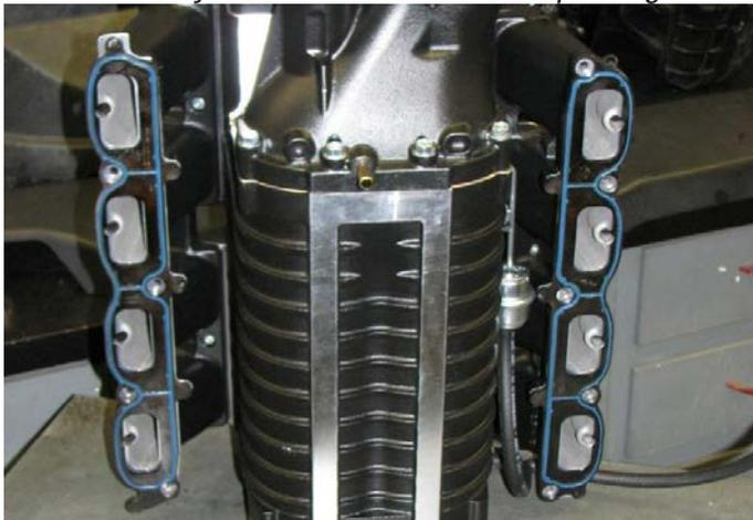
102. Lift the supercharger assembly, with the flange gaskets in place, over the water crossover and onto the engine. Insert the M6 x 30mm manifold bolts supplied in Bag #1 into their provisions to determine when the manifold is properly aligned.
