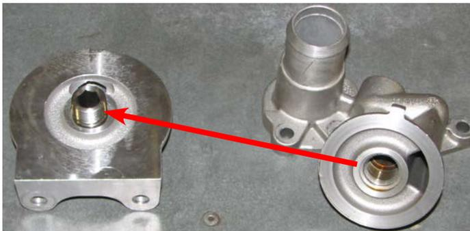
81. 2wd trucks should now install the oil filter on the new bracket, while 4wd trucks should refer to the instructions supplied with the #15834 kit
