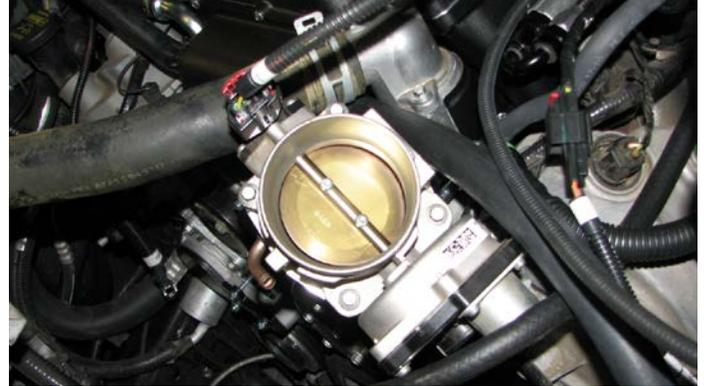
142. Attach the ETC Extension and TPS connectors to the throttle body and connect the other end of the ETC Extension to the stock ETC harness connector.
