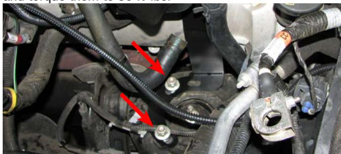
115. Install the Supercharger to Reservoir hose between the intercooler reservoir and the passenger side of the supercharger and secure both ends with the hose clamps supplied in Bag #5.
