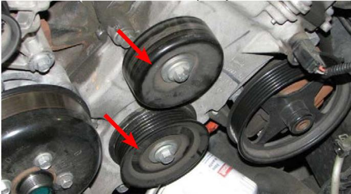
53. Use the stock bolts, in their original locations, to install the supplied idler pulleys on the two, front cover, bosses; the 90mm grooved pulley goes on the top boss, the 76mm smooth pulley goes on the lower boss.
