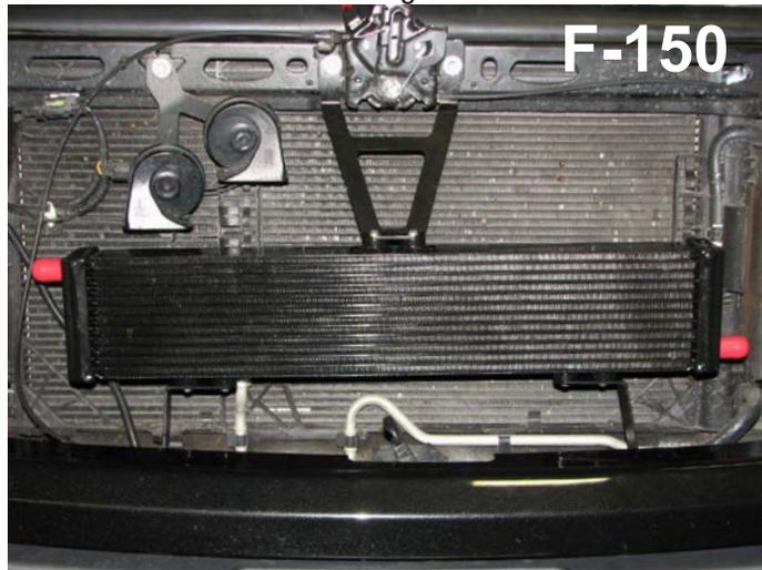
124. Route the Heat Exchanger to Supercharger hose: from the top of the engine bay, down towards the driver side headlight, around the front of the radiator, and attach it to the heat exchanger outlet fitting. Secure the fitting with a hose clamp supplied in Bag #5.
