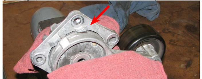
96. Use a grinding wheel or file to ensure that the area that was ground down is smooth and free of burrs.
