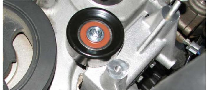
76. Tighten down the four mounting bolts, then tighten the pulley bolt. Verify that the pulley can spin freely once all the filter bracket bolts have been tightened.
