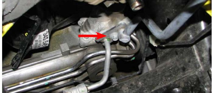
66. The power steering pressure line can now be pulled out of the steering box and removed from the vehicle.
