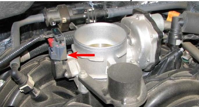
12. Use an 8mm socket to remove the two front throttle body bolts then remove the throttle body weight.
