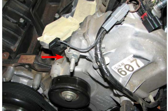
44. Carefully remove the intake gaskets from the intake manifold by pushing the clips out of each hole in the flange
