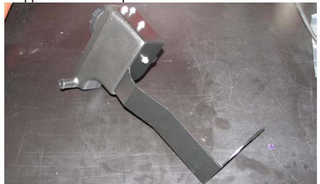
114. Install the intercooler reservoir so that the bracket is on the strut tower studs. Reinstall the strut tower nuts and torque them to 30 ft-lbs.
