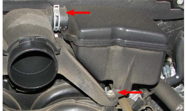
7. Detach the electrical connector from the MAF sensor on the air box cover.
