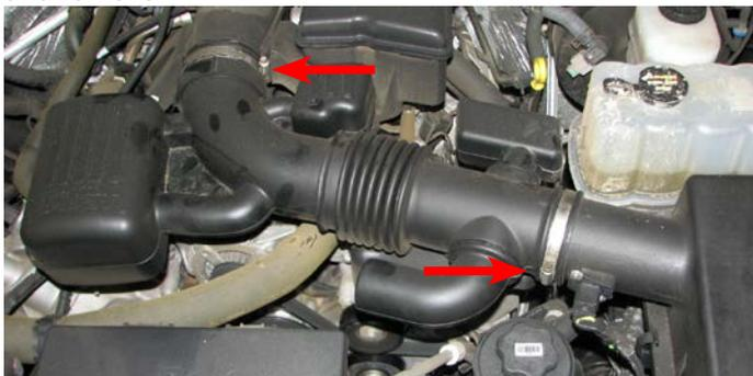
5. Disconnect the PCV tube running between the throttle body elbow and the passenger side valve cover.
