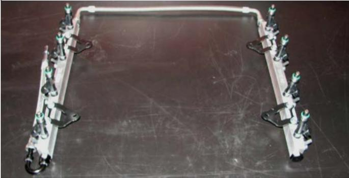
107. Apply a small amount of lube to each injector and insert them into the injector provisions in the fuel rails. Install the fuel crossover line on the two straight fittings and the fuel inlet line on the black inlet fitting.
