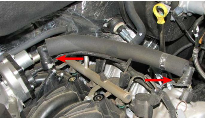
11. Detach the throttle position sensor (TPS) connector from the driver side of the throttle body.
