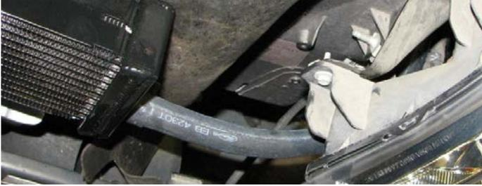
125. Route the molded hose from the bottom of the intercooler reservoir to the water pump inlet. Note the location where it intersects with the passenger side radiator shroud and make a small incision in the shroud. Feed the hose through the incision and attach it to the water pump inlet, securing the fitting with a hose clamp supplied in Bag #5.
