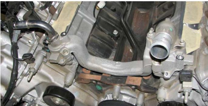
42. Use an 8mm socket to unbolt and remove the water crossover from the engine. Remove the gaskets on each end and retain them, as they will be reused. Then place making tape over each water passage.
