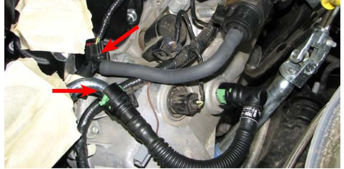
129. Connect the 90° end of the driver side PCV hose to the valve cover fitting. Connect the straight end to: the upper, 90° fitting, behind the throttle body flange, on the air inlet, next to the thermostat housing.
