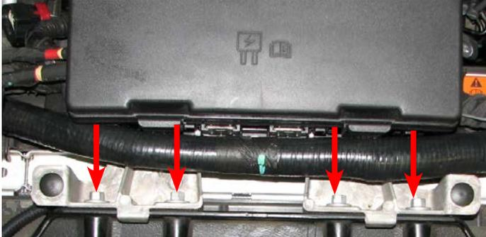
90. Route the alternator wire harness along the top of the radiator, working it below the fuse box support brackets, then plug it into the alternator.
