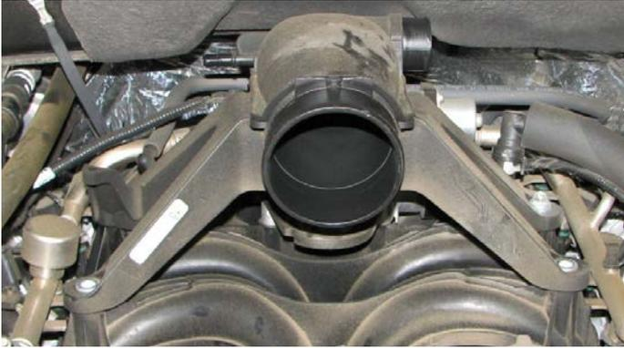
10. Detach and remove the driver side PCV tube from the intake manifold and valve cover.
