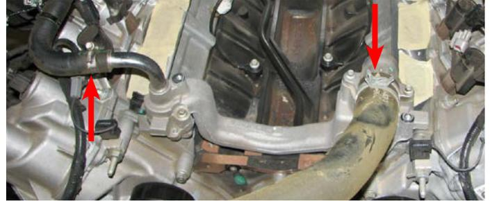
31. Use a screwdriver to remove the clamp that holds the heater hose to the water crossover then pull off the hose.
