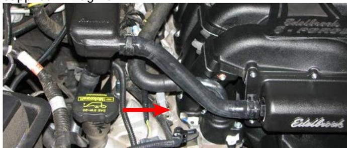
116. Install the water pump into the water pump bracket so that the pump outlet will point up when installed and the pump inlet points toward the passenger side fender. Secure the water pump to the bracket using the strap and the M8 x 30mm bolt supplied in Bag #5.
