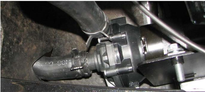
126. Mount the Water Pump to Heat Exchanger hose on the water pump outlet and heat exchanger inlet and secure the fittings with hose clamps supplied in Bag #5.
