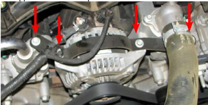
23. Remove the electrical connector from the alternator. Use a 10mm socket to remove the nut retaining the power wire. Remove the power wire and replace the nut.
