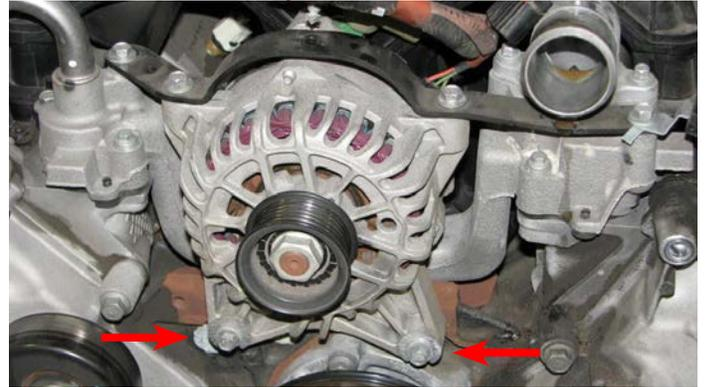
25. Trace the alternator power wire back to the harness connector, on the passenger side of the radiator, and disconnect it then remove the entire power wire harness.
