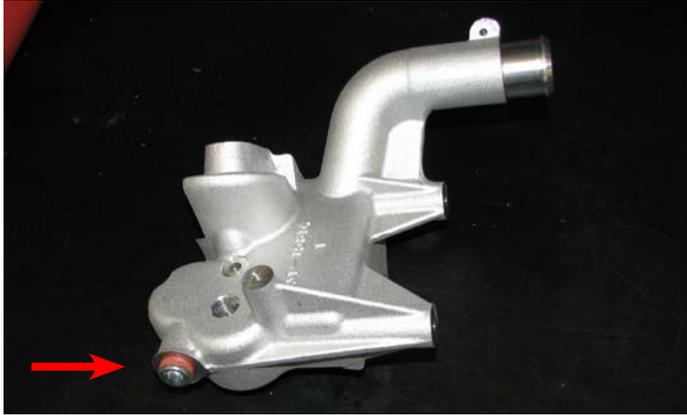
72. Place the oil filter bracket gasket on the flange of the supplied bracket. Once the bracket is close enough, attach the electrical connector to the oil pressure sensor.
