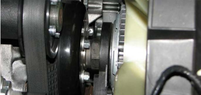
41. Use an 8mm socket to unbolt the thermostat housing and remove it. The housing, thermostat and O-ring will all be reused.
