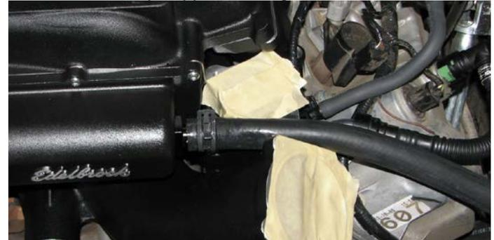
131. Install the stock thermostat, O-ring and housing on the new water crossover and install the stock bolts.
