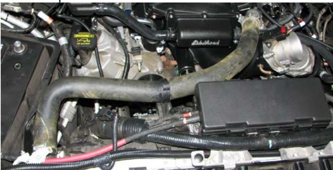
140. Remove the plastic sheet from the supercharger air inlet and install the throttle body O-ring supplied in Bag #1, on to the air inlet flange.
