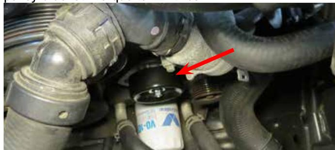
51. Using hose clamp pliers, remove factory coolant bleed hose and discard. Use the factory clamps to install the included hose show below.
