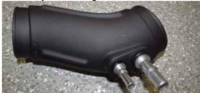
102. Install the inlet tube and air box lid using the supplied boots and clamps as shown below. **Do not over tighten clamps.**
