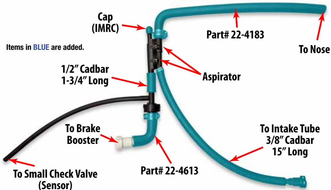
104. For early **2019** models, install the new brake booster hose assembly using the factory clamps to secure the rubber line to the supercharger fitting. Push the two (2) remaining connectors onto their respective fittings to lock them in place. Reconnect the 1/4" hose to the fitting on the line.
