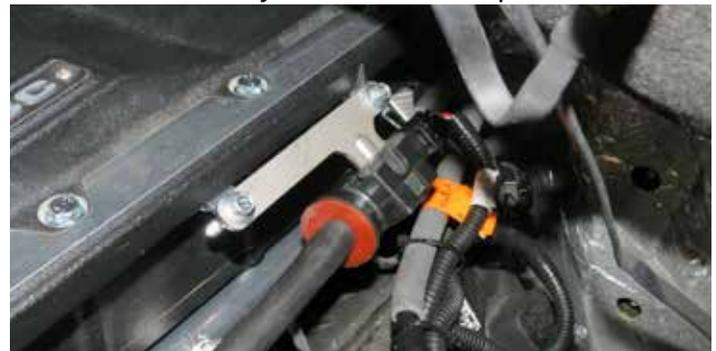
C) Connect the relay harness to the previously installed intercooler water pump and fasten the ground strap to the pump bracket.
