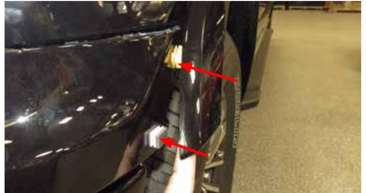
8. Remove plastic bumper cover by pulling outward until panel detaches. Take clips from step 18 out of bumper cover by pressing in the tabs on the inside of the bumper cover.
