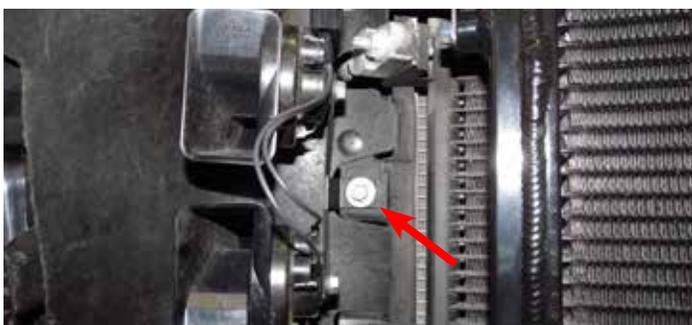
93. Install the intercooler pump harness using steps A-D (harness ends are labeled for your convenience). **Note: All wires should be clear of any moving or potentially hot surfaces. Secure wires in a safe position with wire ties as necessary.**
