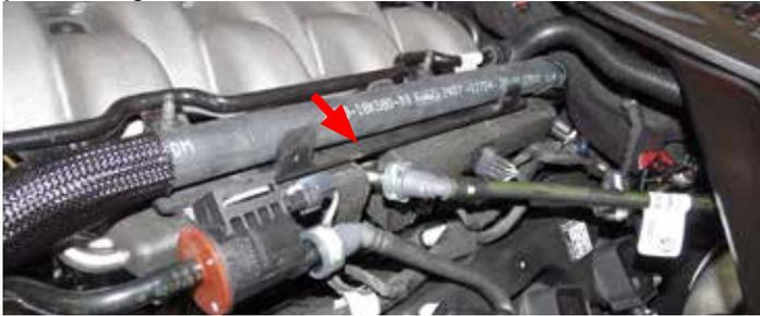
21. Repeating spill protection procedures from step 31, remove the fuel line from the passenger side fuel rail. Use a 3/8" fuel line disconnect tool to remove the line.
