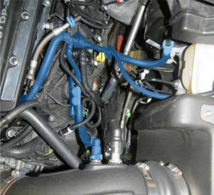
105. Reinstall the factory driver side PCV hose into the inlet tube as shown. Note: Twist the connectors until the hose matches the orientation shown below.
