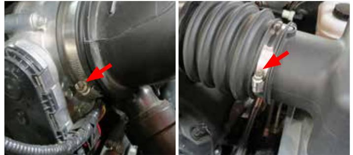
13. Remove the brake aspirator and driver side PCV hose from the back of the intake tube. Remove PCV hose from driver side valve cover and set aside. **TIP:** The brake hose is removed by pushing down the yellow clip and pulling out on connector. The PCV hose is removed by pushing out on the grey tab and pulling the connector out.
