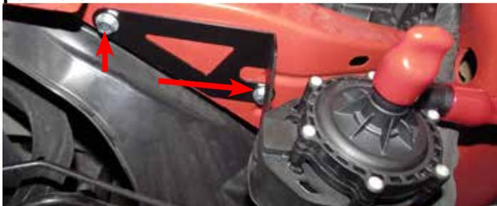
80. Remove the indicated strut tower nut and install intercooler reservoir bracket over stud. Loosely tighten the strut tower nut. Using the supplied M8 x 20mm bolt, washers and nut located in bag #3, fasten the bracket to the hole on the back of the control arm mount. Install intercooler overflow tank on bracket using the supplied M6 x 10mm bolts and align bracket so tank is sitting upright. Tighten all hardware. **Do not overtighten bolts securing tank to bracket.**
