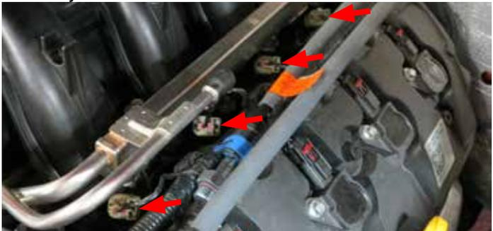
23. Using a 10mm socket, remove four (4) fuel rail bolts (driver side shown). Firmly and evenly lift up on fuel rail from both sides and remove from intake manifold.
