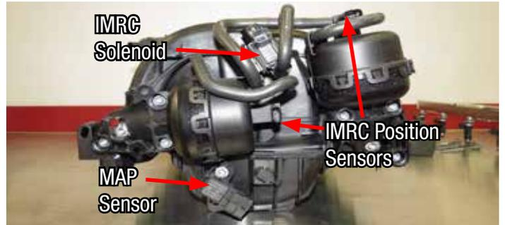
26. Make sure the IMRC harness is completely disconnected from above locations and remove the manifold. Clean the cylinder head surfaces and tape off intake ports so nothing can mistakenly fall into any of the cylinders.
