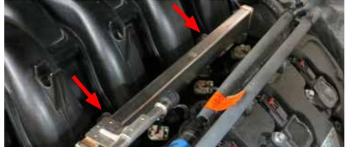
24. Using an 8mm socket, loosen the remaining six (6) intake manifold bolts. Note: Bolts can not be removed from manifold. Loosen enough so threads are disengaged from the cylinder head.
