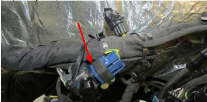
28. Tape up the end of the two (2) IMRC position sensor plugs and secure plugs to the main harness out of the way. These will not be reused.
