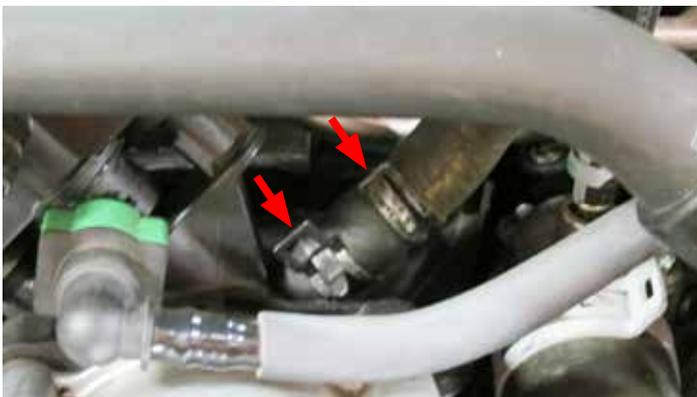
16. Disconnect the evap line from the solenoid by squeezing the green clip together at the bottom and lifting the tab up. Disconnect evap harness by pushing down the black tab and pulling plug out.
