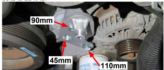
48. Install the supplied tensioner with one (1) M10 x 65mm bolt from bag #2. Leave the tensioner bolt loose until the belt is installed. **NOTE: AC line should be CAREFULLY bent away from the tensioner to allow clearance as shown below.**
