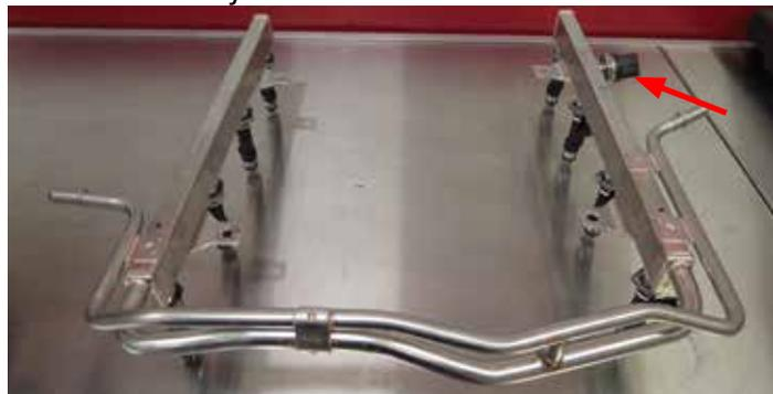
63. Apply fuel resistant thread sealer to the threads of the fuel pressure sensor adapter. Thread the adapter into the supercharger fuel rail until snug. **Ensure not to overtighten and strip threads.** Apply the same thread sealer to the fuel pressure sensor and thread it into the adapter. Prevent the adapter from twisting in further with a second wrench. Optionally continue to twist the sensor once snug until it aligns with fuel rail.
