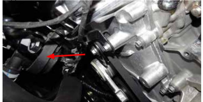
33. Remove the auxiliary water pump bracket from the front of the engine by removing the two (2) bolts and one nut securing it. The second bolt (not shown) is located further down on front of engine.
