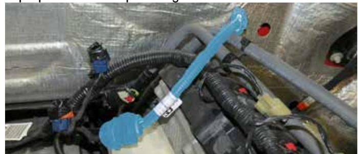
54. Remove the O-ring manifold gaskets from the factory manifold and install them onto the supercharger runners. Apply a small amount of O-ring lubricant to the exposed area of the gaskets. This will help prevent tears during installation of the supercharger.
