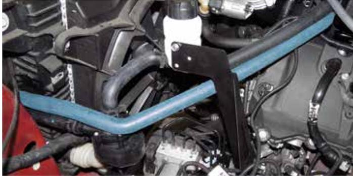
85. Install water pump to LTR hose using the supplied pinch clamps in bag #3 and route through the radiator shroud as shown.
