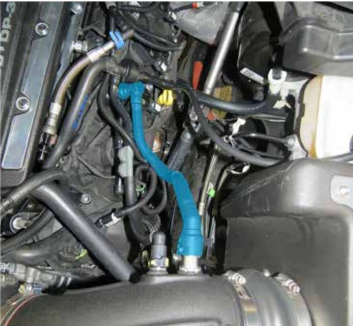
106. For later **2019** models, install the 90° hose and fitting to the brake booster. Connect the long hose on the opposite end of the assembly to the supercharger nose. Connect the hose with the push connector onto the smaller fitting on the intake tube. Reconnect the skinny hose to the brake boost sensor. Connect the remaining PCV hose to the air intake.
