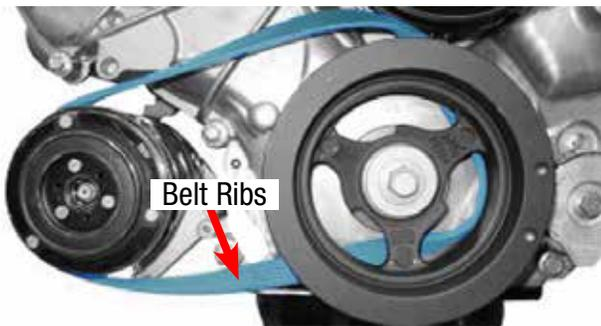
36. Position the A/C compressor belt onto the top of the crankshaft pulley. Using wires ties, securely hold the belt onto the crankshaft pulley at the 12 o'clock position. Do this by feeding the wire ties through the crankshaft pulley spokes, up and over the A/C compressor belt and then securely tighten the wire ties.
