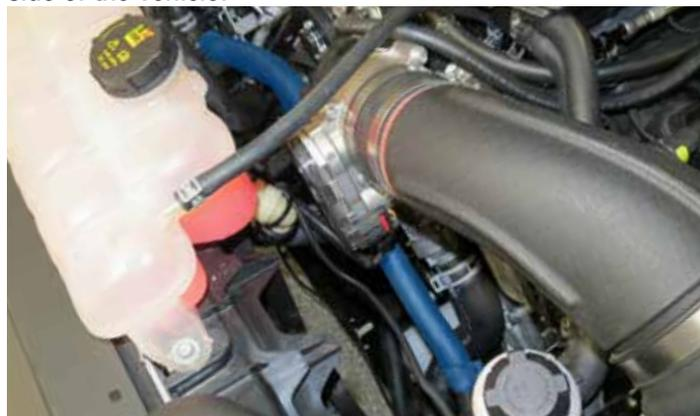
77. Clock the factory auxiliary water pump so the coolant output is pointing towards the radiator. Install the 90° elbow on to the pump outlet and splice together to the rest of the heater hose using the 3/4" straight fitting. Secure with supplied hose clamps.
