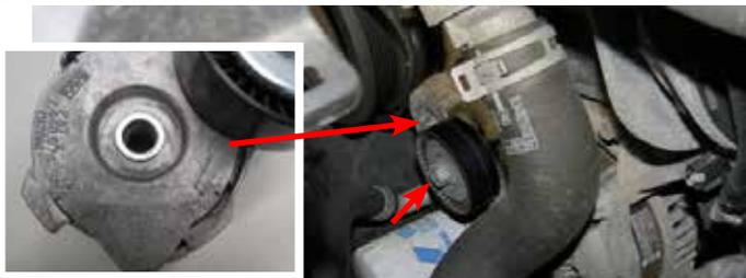
30. Using a 3/8" breaker bar or equivalent, release the tension from the secondary A/C drive tensioner and remove the A/C drive belt and discard.
