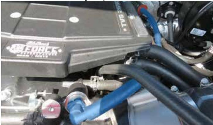
70. Using an 8mm socket, remove the throttle body from the stock manifold and install it onto the supercharger manifold using the supplied O-ring gasket, factory bolts and included extension harness.
