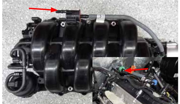
17. Remove the passenger side PCV hose by pushing the grey tabs out and pulling up on the connectors.
