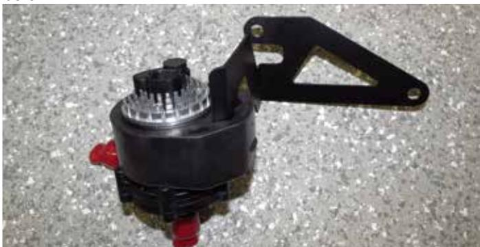
79. Locate the two (2) holes on the driver side air box support and install intercooler pump and bracket assembly using the M8 x 20mm bolt and Nut located in bag #3. **NOTE: The bolt on the left can be loosely installed at this time. The intercooler relay ground wire will connect to this point later.**
