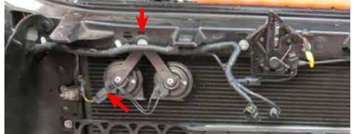
87. Disassemble the horns from the factory bracket and reinstall on the included, new bracket as shown.
