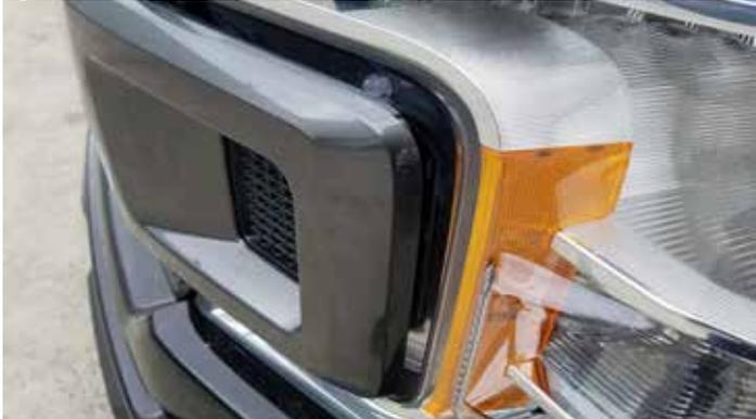
11. Unplug the grille shutter control and ambient temp sensor located in front of the hood latch. Using a panel puller, remove harness from grille. **Remove grille by lifting up and out and set aside.**
