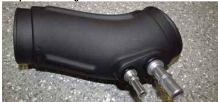
98. Install the inlet tube using the supplied boots and clamps as shown below. **Do not over tighten clamps.**
