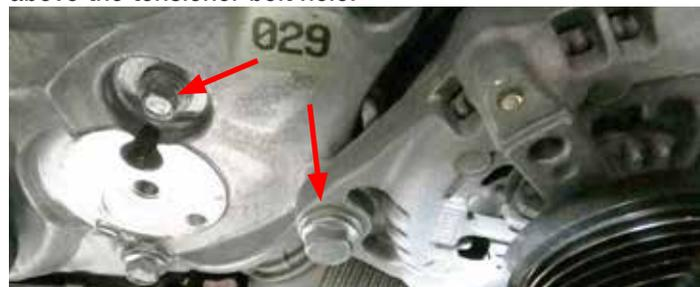
47. Using the bolts supplied in Bag #2, secure the small idler bracket by installing the M10 x 110mm bolt through the ear of the alternator, the M8 x 90mm bolt into the top front cover hole and the M10 x 45mm bolt through the center hole that was used to secure the stock tensioner. Torque M10 x 110mm bolt to 32 ft/lbs and the other two bolts to 22 ft-lb.
