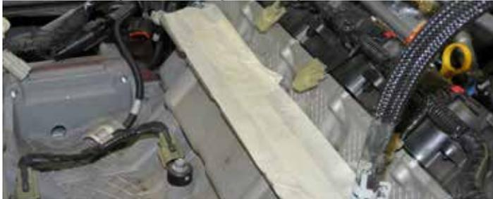
27. Remove the IMRC Solenoid from the manifold. Reconnect to the harness and zip tie out of the way. The solenoid will not be used but **MUST** be plugged in for proper engine operation.
