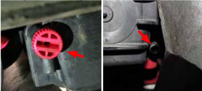
4. Using a panel puller, remove fourteen (14) push pins securing the top radiator shroud. Remove the shroud and set aside.
