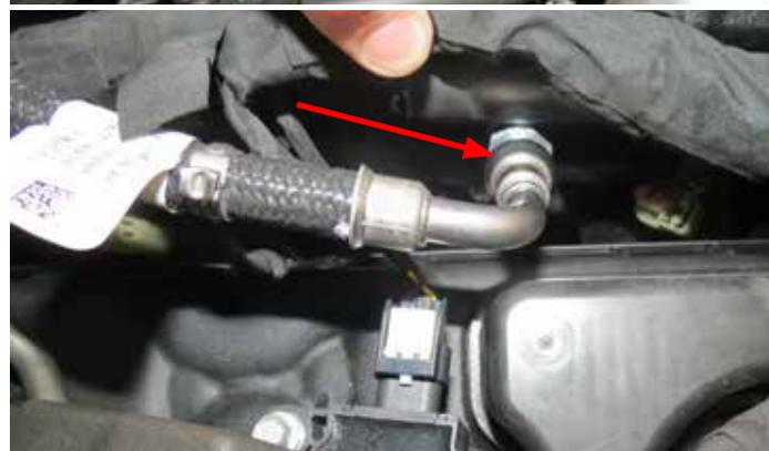
68. Remove the evap solenoid from the factory manifold. Using two (2) M6 x 25mm bolts Install the evap bracket to the supports. Install the solenoid onto the bracket using the factory rubber grommet. **NOTE: These bolts will be need to be removed later when installing the side covers.**
