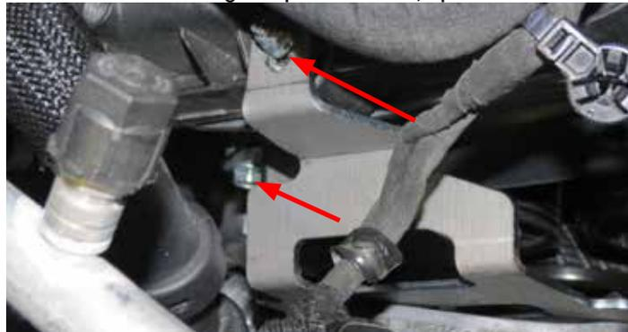
75. Reinsert the pump into the isolator on the newly installed bracket.
