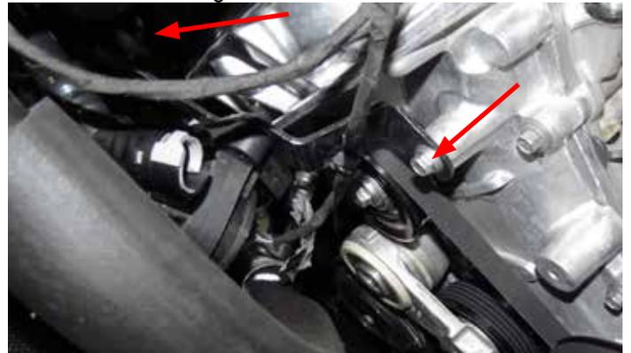
34. Remove rubber support from factory bracket and install into provided bracket as shown.
