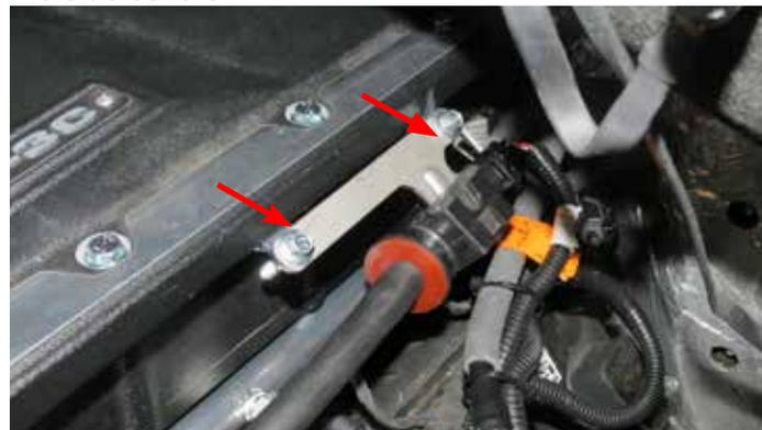
69. Install the provided hose onto the evap solenoid and connect the 90° fitting to the fitting on the supercharger inlet. Connect the factory evap line to the rear of the solenoid.
