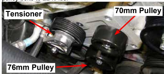
50. Using one (1) M8 x 20mm bolt and one (1) M8 washer from bag #2, install the 65mm pulley to the small idler pulley bracket. Torque to 22 ft-lbs.
