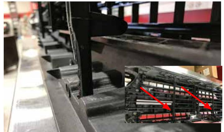
110. Reinstall the grille and radiator cover using the factory hardware and the two, new push pins that secure the air scoop as shows below. **Be sure to reconnect the grill shutter harness.**
