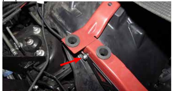
D) Position the relay on the driver side plastic wheel well as shown below. Make sure the wires have some slack and mark the area inside the metal tab attached to the relay. Drill a 1/4" hole on the mark and fasten the relay to the new mounting point using the supplied push pin in bag #3.
