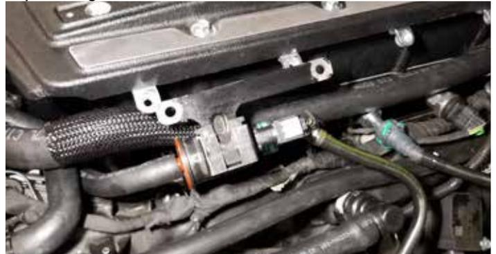
135. As a precaution, slice a 5" length of hose to wrap around the fuel line as pictured. This is to prevent the hose from rubbing on the edge of the coil cover. Secure with zip-ties.
