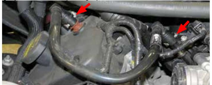
18. Disconnect the throttle body harness by pulling the red locking tab out and push down on the black tab as you pull the plug out.
