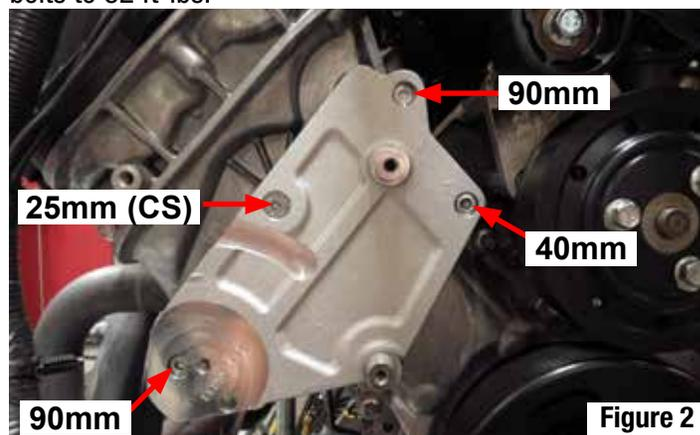
Using a 15mm and 10mm socket, remove the lower bolt securing the alternator and the front cover bolt directly above the tensioner bolt hole.
