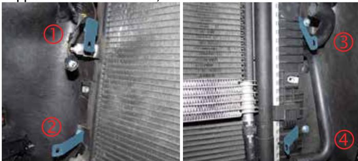
89. Install the LTR onto the brackets using the M6 X 10mm bolts from bag #3. Leave these bolts slightly loose for alignment.
