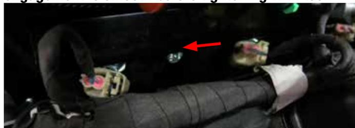
66. Reconnect the fuel injectors and fuel rail pressure sensor. **WARNING: Never attempt to rotate the injectors.**
