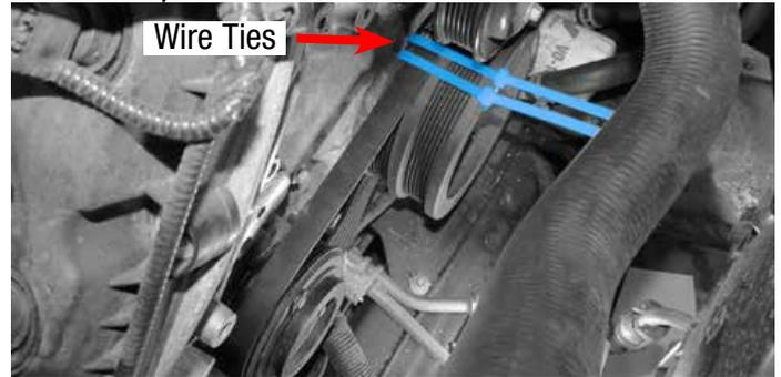
**CAUTION:** It is crucial to maintain the belt alignment with A/C compressor pulley when rotating the crankshaft pulley. This is done by carefully pulling the belt towards the front of the vehicle, with your free hand, while rotating the crankshaft pulley. The belt will have a tendency to skip a groove if not done so; resulting in an unusable belt.
