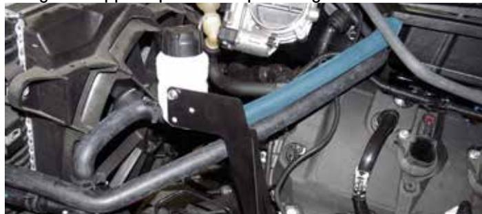
82. Install the surge tank to water pump hose as shown using the supplied pinch clamps in bag #3.
