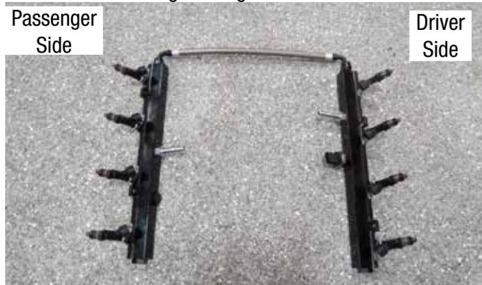
65. Install the fuel rails and secure using four (4) M6 x 16mm bolts from Bag # 1. Bolt holes are located beneath the fuel rail. **Start fuel rail bolts BY HAND first and make sure thread engagement is smooth before tightening with tool.**
