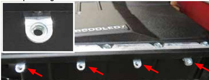
56. For proper bracket alignment, test fit the side covers onto the brackets using eight (8) M6 X 25mm bolts from the side cover kit. While pushing the side covers forward, fully tighten the bracket bolts. Once all brackets are aligned and tightened, remove the side covers.
