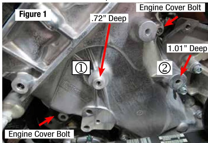
41. Tap hole #1 and #2 with the M10 x 1.5 tap from Bag #2. Remove all metal shavings from engine bay.
