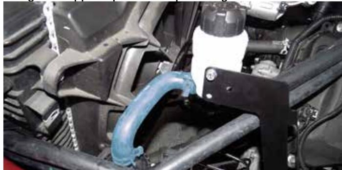
83. Install supercharger to LTR hose using the supplied pinch clamps in bag #3 and route through radiator shroud as shown.
