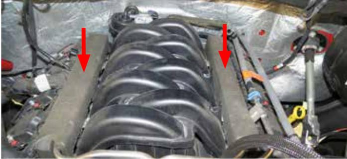
20. With the vehicle **COMPLETELY** cooled. Put rags under the fuel rail fitting and remove the fuel line from the rail. Cap off the fuel rail and fuel line with appropriate cap and plug to prevent spillage. Clean up any spilt fuel before proceeding.
