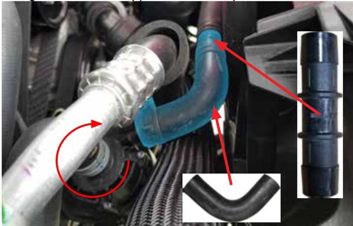
78. Install the intercooler pump damper onto the pump then install pump bracket into damper as shown below.
