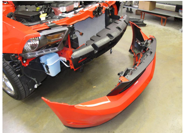
Fig. 1J: Front Fascia Removal
