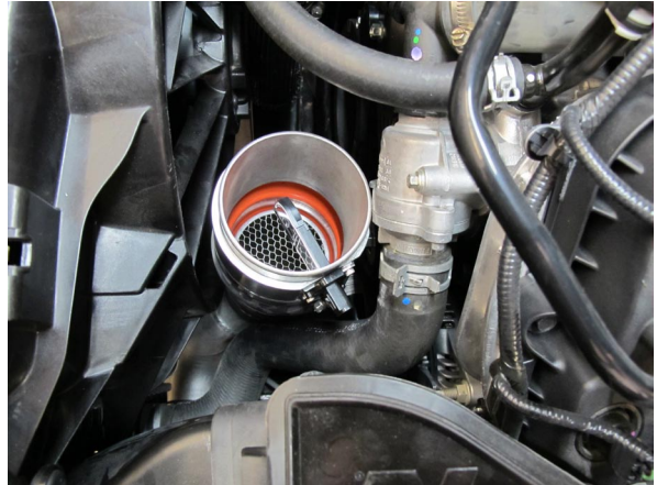
Fig. 7C-5: MAF Location (orientation will vary)
