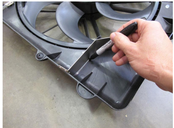
Fig. 3AD: Marking Air Dam Cut Lines
