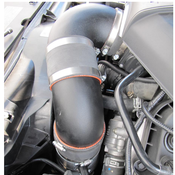
Fig. 7C-7: Cast Elbows, Final Position
