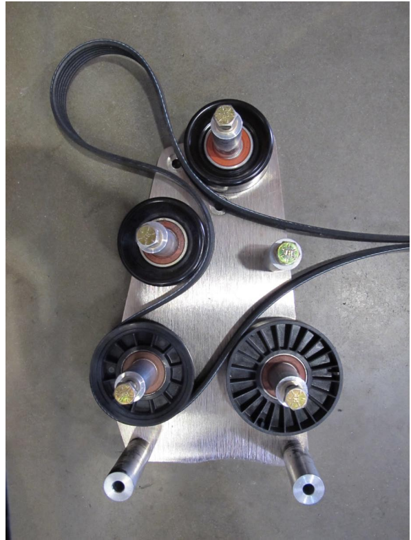
Fig. 4B: Belt Routing (front plate removed for clarity)
