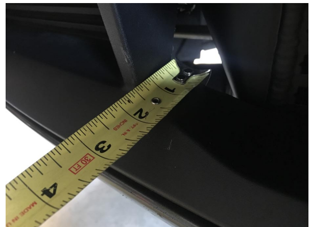
Fig. 12D-5: Bumper Cover, Center; Cut Line Reference
