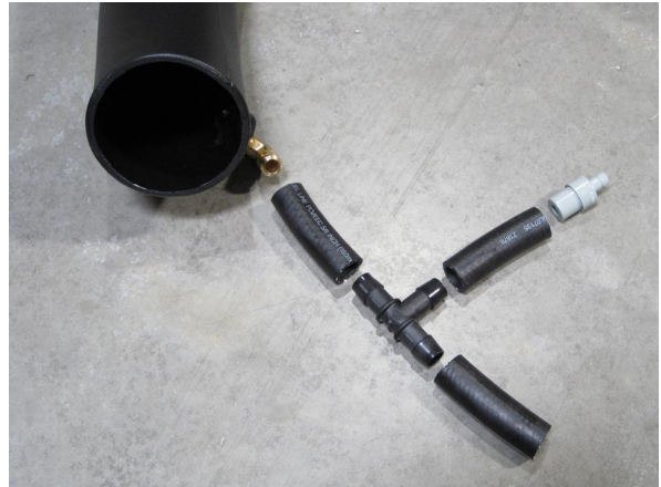
Fig. 11F: (Automatic Transmission Only) Driver Side PCV Hose Modification (Hose Segments Cut for Illustration Only)
