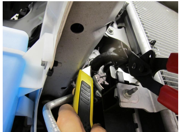
Fig. 2G: Clamping and Cutting A/T Hoses
