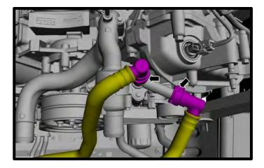
34. (**Dual Alternator**) Remove the (5) bolts from thermostat housing using a 10mm socket.
