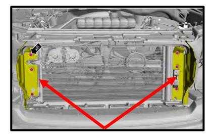
87. Remove the stock horn bracket with horns from the vehicle using a 13mm socket.
