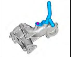
29. (**Single Alternator**) Install the supplied #2-113 oring to the shorter heater tube and install to factory location, secure with stock fastener, torque to 89 lbs-in. Reconnect both factory hoses, secure lower hose with stock clamp. **NOTE:** Some 2022 models, built without the auto start/stop pump. These are equipped with a 55deg fitting (blue arrow). Remove the stock fitting from stock hose, install the supplied 90deg fitting, secure with stock clamp.
