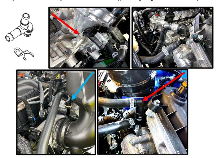
30. (**Single Alternator**) Transfer stock oring from stock water neck to new water neck (clean oring as needed). Apply pipe sealant to threads of 1/8" NPT to 5/16" 45 Deg fitting. Install fitting to water neck, rotate so it ends facing directly towards driver side. Install water neck to motor using stock fasteners (10mm socket), torque to 89 lbs-in.
