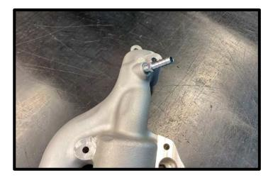
39. **(Dual Alternator)** Install the new thermostat housing assembly to engine using (3) of the factory fasteners, leave hand tight for now.
