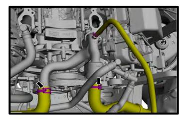
33. (Dual Alternator) Release the (2) coolant lines from the factory LH heater tube.
