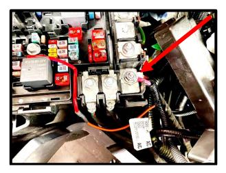
112. Remove the ground bolt from the **RH** side frame, next to the battery using an 8mm socket. Install IC pump relay ground eyelet here. Secure with factory bolt using an 8mm socket.
