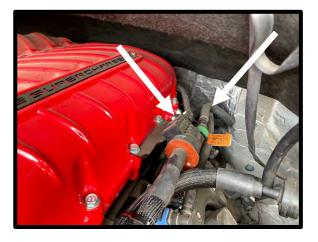
77. Install the supplied 3/8" ID x 13" with 55deg quick connect fitting hose to the EECPV barb fitting and **upper** quick connect fitting on SC inlet. Push until it clicks and locks into place.
