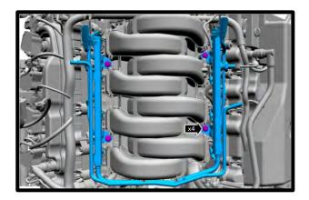
23. Disconnect all 8 fuel injectors from factory injector harness.
