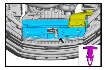
8. Disconnect the factory camera and windshield washer fluid connection from front grill area when applicable.
