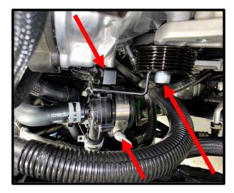
83. Install the supercharger pulley using the supplied (5) 6mm x 14mm SHCS using a 5mm allen socket. Leave hand tight until belt installation.
