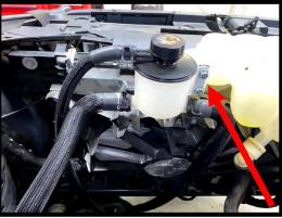
95. Install the ¾" ID x 32" hose (#3103094) and the 3/8" ID 39" (#3103098) rubber hoses to the IC filler neck. Secure with supplied pinch clamps. Connect the ¾" hose to the IC pump inlet fitting, secure with pinch clamp. Secure 3/8" vent hose with zip tie to the ¾" hose. **NOTE: Ensure that this hose cannot kink or rub anything overtime.**
