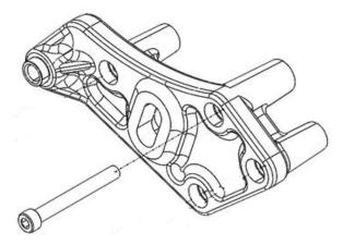
66. Torque the (10) 6mm (10) HHFCS manifold bolts in the following pattern using a 10mm socket. First pass: 88 lbs-in. Second pass: 106 lb-in. **NOTE:** For bolt #10, a ¼" socket with 4"-6" extension, 10mm wobble is the best possible tool to get into this tight area.
