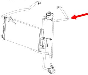
97. Install supplied ¾" ID x 22" hose #3103093 90deg end to heat exchanger top fitting. Route other end to **RH** (**INLET**) intercooler fitting. Secure with supplied constant tension clamps. \***NOTE**: Make sure the hose does not and cannot kink during routing. **DO NOT** lay the hose on the cam sensor wires, this will lead to failure over time.
