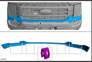
10. Remove the (4) bolts using a 10mm socket and the (2) push pins from the upper side of the grill shell. Remove the (2) lower bolts from the bottom side of the grill shell.
