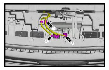
9. Remove the (2 per side) push pins from the lower grill shell in the inner fender area. Pull the lower grill shell section from the vehicle.
