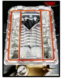
58. Install the supplied pre-formed 65.3" x .103" oring to the top sealing surface of the SC housing. Apply generous amount of grease to help ease the oring into place. **TIP:** To install oring into dove-tail groove, press vertically, vs sliding finger along.
