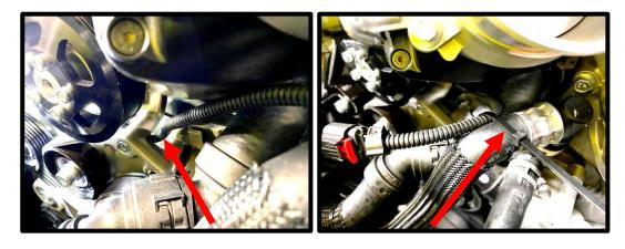
71. Reinstall the water pump pulley using a 10mm socket, torque to 14 lbs-ft.
