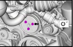
47. Using a 10mm socket, remove the (3) factory fasteners from the timing chain to head cover and (1) from water pump (for new idler plate).
