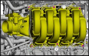
21. Use compressed air and remove any direct or foreign material from cylinder head, block and surrounding area of the fuel rail and injectors. Remove the intake manifold from the engine. To do so, remove the (5) wire harness push pin supports from the back of the intake manifold and disconnect the 4-way MAP sensor connector.
