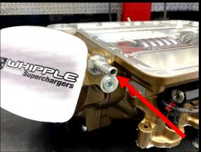
78. Install the stock PCV hose to the **RH** side valve cover. Connect other end to the supercharger inlet 15.82mm quick connect fitting. \*Note: This requires you to rotate the fittings for proper fitment. Push until it clicks and locks into place.
