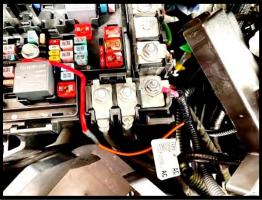
114. Install the fuse box cover, ensure the turn-on wire is clear of cover.
