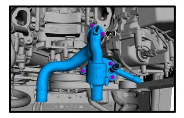
35. (Dual Alternator) Visually inspect factory orings from thermostat housing. Transfer to new thermostat housing.
