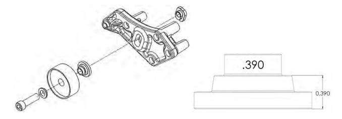
81. Install the supplied (1) grooved idler pulley #36326 to the idler plate using the (1) idler step washer and (1) ½"-13 x 2" SHCS. Install the supplied circulating pump bracket under ½" bolt head, secure other end to front engine timing cover using stock bolt. Torque idler pulley bolt to 30 lbs-ft. using a 3/8" allen socket. Use light amount of anti-seize on threads. **NOTE: Some models are built without these pumps, if so, discard this bracket.**
