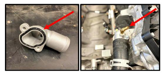
31. (**Single Alternator**) Reinstall water neck hose to new water neck. Using needle nose pliers, reinstall and rotate the factory pinch clamp at the water neck towards the driver side for future clearance of the SC. **NOTE:** Image shows clamp with SC installed to illustrate max clearance.
