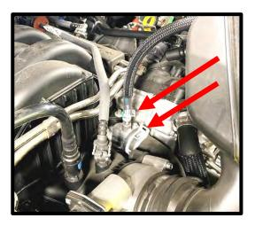
28. **(Single Alternator)** Disconnect the driver side heater tube quick connect fitting by squeezing and lifting away. Remove the heater tube overflow hose using a pinch clamp tool. Using an 8mm socket on the 1 factory bolt, remove the heater tube.
