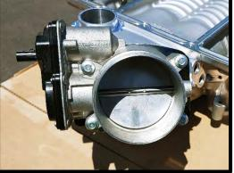
99. (Stage 2 Whipple 132mm Crusher throttle body) Install throttle body to supercharger inlet, use the supplied gasket between TB adapter and SC inlet. Secure with the supplied (3) 6mm x 25mm SHCS and (1) 6mm x 50mm SHCS using a 5mm allen socket. Torque to 89 lbs-in on first pass, 139 lbs-in on second pass.
