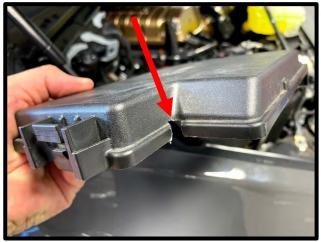
110. Locate the stock hole in the battery box as shown below. Use the supplied plastic push pin to secure the intercooler relay and fuse holder to the battery box. Route power and ground around box to fuse box area.
