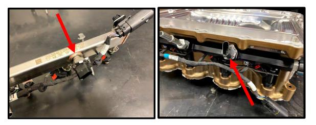
50. Install the supplied (1) #2-906 Viton oring to the (1 of 2) 45mm long 9.49mm inlet fitting to fuel rail. Apply light amount of grease to oring for ease of installation, install to rail.
