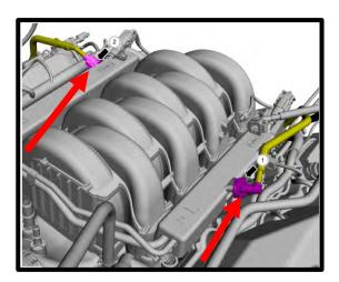
18. Remove fuel rail foam insulation, these will not be reused.
