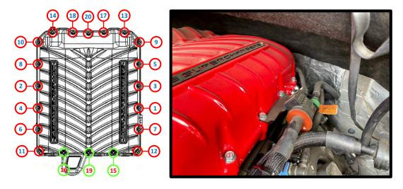
74. Connect the factory high pressure **RH** side rail fitting to the DI pump factory hose, press until it clicks and locks in place. *NOTE: THIS FUEL LINE HAS A CHECK VALVE, NEVER FLIP ORIENTATION FROM STOCK DIRECTION.*
