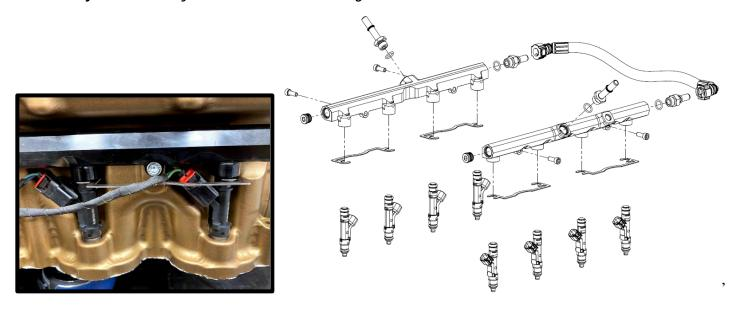
54. Apply generous amount of grease to the injector orings for ease of installation. Install the fuel injectors (*Stage 1 uses stock injectors*, *Stage 1R and 2 uses supplied injectors*), rails and lock bracket to the intake manifold, secure with the (4) 6mm x 16mm SHCS using a 5mm allen socket and use **Blue Loctite** #243. Torque to 90 lbs-in.
