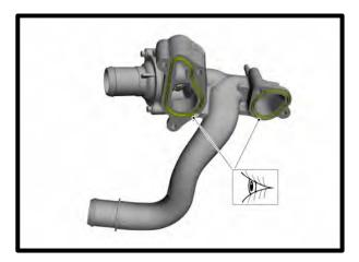
36. **(Dual Alternator)** Remove the **(**2**)** fasteners from the coolant inlet connector, remove inlet connector, thermostat oring and thermostat. Inspect oring, replace if necessary.
