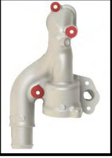
40. **(Dual Alternator)** Install the supplied #2-113 oring to new coolant tube. Install tube to thermostat housing. Secure coolant tube using the (2) 6mm x 50mm HHFCS bolts supplied. Torque all (5) thermostat housing bolts to 89 lbs-in.
