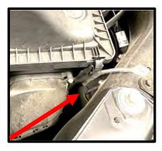
103. Install the supplied lower airbox into factory (2) hole locations. Using the supplied (2) 1.1" L x .30" W plastic push pins, secure front of snorkel to factory location.
