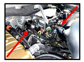
109. Remove the stock fuse box cover located near **RH** firewall. Using small file or cutters, make notch the box as shown for the power wire.
