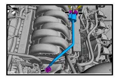
17. Carefully remove the factory fuel line by releasing the safety lock, then squeezing the connector and pulling back. The fuel system may still have pressure, use protective eyewear and multiple rags to catch any possible fuel leak.
