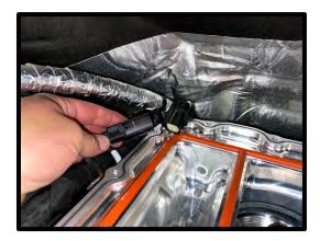
70. Install the supplied electronic throttle pigtail to the factory electrical connector. Route under front idler plate front support for proper safety from belt. Push until it locks in place, then lock the safety lock. Route to **LH** side of vehicle for later connection to throttle body. **TIP:** When pressing together, hold the wires vs connector to ensure the wires do not come loose during connection.
