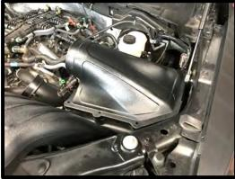
105. Install the (1) supplied 13/16" to ½" rubber grommet into the supercharger inlet tube. Install the supplied ½" to 15.82mm quick connect fitting.
