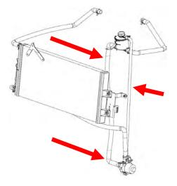
96. Install the ¾" ID x 12" rubber hose (#3103092) from the **LH (OUTLET)** IC fitting to the IC filler neck. Secure both ends with supplied pinch clamps. This goes under the air inlet tube. **NOTE: NEVER SWITCH THE INTERCOOLER ROUTING, BANK 2 IS ALWAYS THE OUTLET!**
