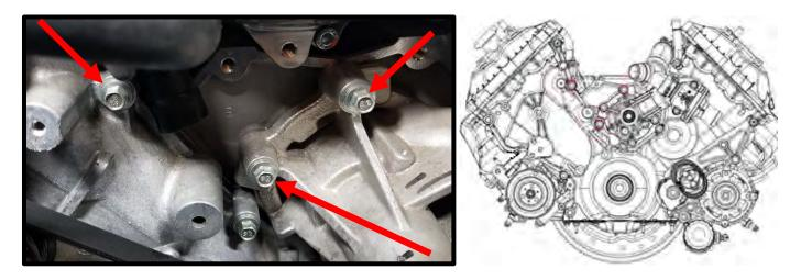
48. Use the supplied (3) 8mm x 90mm SHCS to secure the idler plate to the engine. Using a 6mm allen, torque to 22 lbs-ft.
