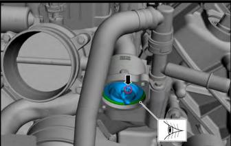
37. **(Dual Alternator)** Install the factory thermostat and thermostat oring to new housing. Install coolant inlet using the factory (2) bolts. Torque to 89 lbs-in.
