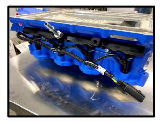
55. Install the supplied ¼" ID bypass actuator to the bypass nipple and ¼" 90deg nipple on SC inlet. **CAUTION:** Do not open/close bypass actuator by hand. This may damage actuator internally. It only moves properly with equal vacuum/boost at the actuator reference port.
