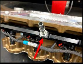
52. Install the supplied (2) #2-906 orings to the (2) inlet/outlet fittings. Install these (2) fittings into rear side of fuel rails. Apply light amount of grease to oring for ease of installation. Using a ¾" wrench (or ¾" deep socket) on both the front and rear fittings, tighten both.
