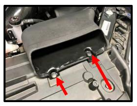
104. Install the supplied panel filter to the airbox lower. Install the upper airbox to the top of the filter. Secure the top to bottom using the supplied (6) 6mm x 16mm BHCS. Torque to 50 in-lbs. \*Caution: Over torqueing can result in pulling an insert out of plastic box.
