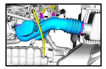
14. Using a 13mm socket, remove the (1) factory fastener securing airbox to the fender. Using a panel pulley or flat head screw driver, remove the (2) push-pins from the factory air snorkel. Remove airbox from vehicle.
