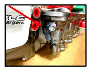
60. Install the supplied TMAP pigtail to the 3-Bar TMAP supplied, wrap up to SC inlet as this will get connected to stock harness later.
