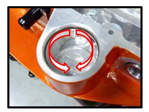
73. Apply generous amount of grease to the (1) #2-230 Viton bypass oring. Install the supercharger lid to the supercharger housing by carefully placing the bypass down. Secure the SC lid using the (17) 6mm x 30mm HHFCS and (3) 6mm x 90mm HHFCS (*marked green*) using the following pattern. Slide the EECPV bracket under bolts 3 and 5 from image (bank 2). Torque to 90 lbs-in using an 10mm socket.
