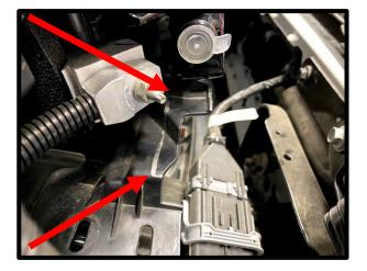
92. Install the supplied pump mount bracket frame opening on **LH** side. Slide J-nut through opening on frame. Secure bracket to J-nut using supplied (1) 6mm x 30mm HHFCS. Install pump clamp to bracket using the supplied (2) 6mm x 10mm HHFCS bolts. Mount pump in clamp using the 1" wide rubber strip around pump, secure clamp. **NOTE:** Outlet fitting should be facing straight up, inlet should be facing center of vehicle.
