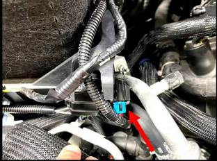
111. Using a 10mm socket, remove the nut on the power stud, located on the positive stud under fuse box cover. Install the IC pump relay power eyelet (red wire) to the power stud on the battery positive (+) stud. Use a 10mm socket to secure stock and IC power wire.
