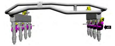
24. **(Stage 1)** Remove the (8) safety clips from injectors. Remove the injectors from fuel rail. Remove the top and bottom orings from stock injectors. Use Berryman B-12 Carburetor cleaner to clean orings or soak orings for a couple hours in a cleaner such as 409 or similar. If orings have any cuts or damage, replace prior to installing. Once clean, reinstall orings to stock fuel injectors.
