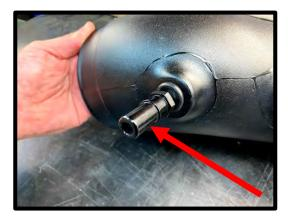
106. (Whipple 132mm Crusher throttle body) Install the supplied 5" ID x 2 1/2" silicone hose over air inlet tube and airbox lid. Install the 4 3/4" x 3" silicone hose over throttle body. Install the air inlet tube between the filter and throttle body. Slide silicone hose over throttle body. Secure all ends with the supplied (4) #80 hose clamps.
