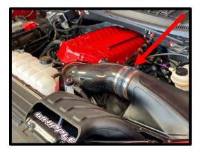
107. (Stock throttle body installations) Install the supplied 5" ID x 2 1/2" silicone hose over air inlet tube and airbox lid. Install the supplied reducer silicone hose over air inlet tube and stock throttle body. Connect the other end to the stock throttle body. Secure all ends with the supplied hose clamps (2) #80, (1) #64 and (1) #56 on throttle body.
