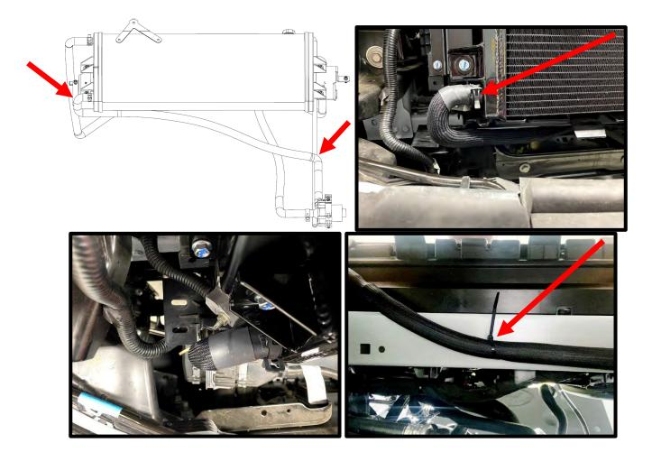
94. Using a 10mm socket, remove the stock coolant reservoir **LH** side bolt. Install the IC filler tee bracket under the coolant reservoir mounting tab. Reinstall factory bolt. Secure filler tee to the bracket using the (2) 6mm x 14mm HHFCS (10mm allen socket).
