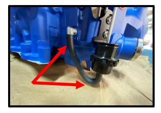
56. Install the (3) supplied 6AN viton orings (#906) to the (1) -6 ORB to 9.89mm, the (1) -6 ORB to 15.82mm and (1) -6 ORB plug supplied from bag WBG-FORD-009. Bank 1 side, install (1) 15.82mm fitting to port using a 7/8" deep socket. Bank 2 side, install the 9.89mm fitting in the top port using a 11/16" deep socket or wrench. Bank 2 side, install (1) 6 ORB plug to the lower port using a 6mm allen socket.
