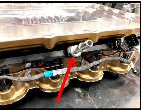
51. Install the supplied (1) #2-906 Viton oring to the (1 of 2) 45mm long 9.49mm outlet fitting. Apply light amount of grease to oring for ease of installation, install to rail.
