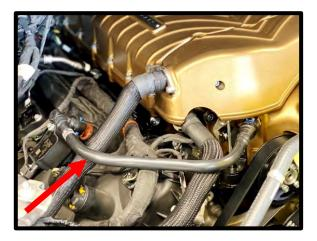
79. Connect the coolant vent line to new 5/16" 45deg barb fitting at water neck using stock clamp. Failure to do this will result in possible leak.
