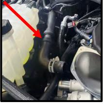
42. **(Dual Alternator)** Reconnect factory quick connect fittings to new coolant tubes. **NOTE:** Some model F150's switched the top fitting from the 90deg to a 55deg (blue arrow). Replace the 45 deg fitting with the supplied 90deg fitting.
