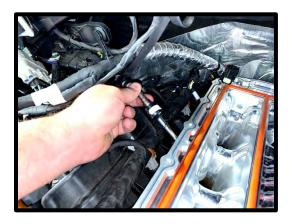
75. Connect the factory fuel inlet line to the driver side fuel fitting, press until it clicks and locks in place. Connect factory fuel psi sensor connector to sensor, press safety lock until it clicks into place.
