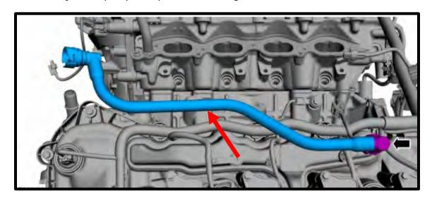
13. Disconnect the (1 or 2) quick connect fittings from air inlet tube. Using a 9/32" nut driver, loosen the factory hose clamp securing the air inlet tube to the throttle body and airbox. Carefully cut the electric tape securing the ETC wires to the throttle body. Disconnect the electronic throttle electrical connector by pushing up on the safety lock and then squeezing the connector and pulling away.
