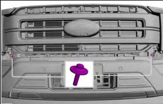
11. Remove the (4) pin-type retainer. Pull up and disengage the locating pins along the top of the grill. Pull forward on center of the grill to remove.
