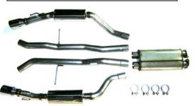
Note: anti-seize should be applied to all fastener threads, pipe slip joints and mating surfaces of ball /socket connections.
