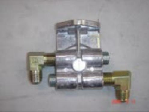
116. Install adapter onto engine and tighten
