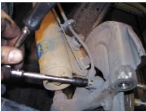
13.Loosen lower ball joint 15/16 nut (both left and right) until there is a 1/8 inch gap with the nut maintaining full thread engagement.
