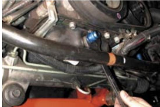
61. Install main turbine inlet pipe. From underneath, raise pipe up and bolt to passenger side exhaust manifold using factory nuts.
