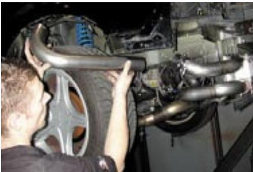
100. Install 4" turbo inlet pipe, Massair meter, and filter onto turbo inlet. Make sure that the flow is correct and the air filter is secured to the end of the meter. Leave clamps loose until final intercooler pipe fitment.
