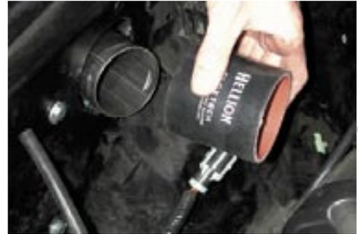
99. Install intercooler pipe #3 and silicone hose.
