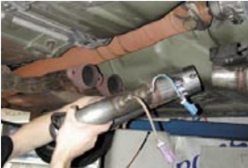
75. Bolt Y-pipe to mufflers.
