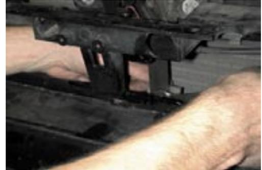
94. To mount Power Steering cooler, either bend power steering cooling line to reach front tab on intercooler, OR Cut 3/8" PS feed and return lines. Install supplied line and splices to extend cooler to reach front of intercooler.
