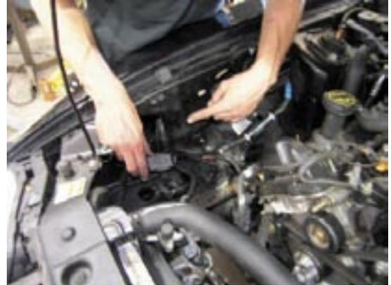
43. If necessary, Unbolt AC line from block, Remove stud that originally held AC line.
