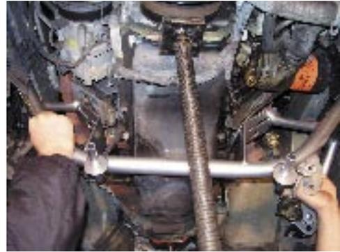
25. Install bushings and sleeves into tubular A-arms, making sure that the short sleeve is in front, and the long sleeve in back
