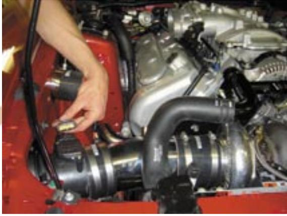
102. Install intercooler pipe #4 and 2.5" by Oval silicone hose adaptor to throttle body.
