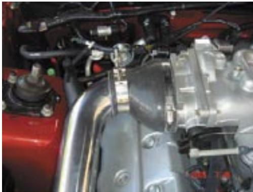
103. Bolt Blow Off Valve to Stub off of inlet tube. Install blow off valve outlet to stub on the 4-inch tube inlet, using 1 3/8 silicone hose and supplied clamps.
