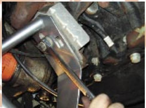
28. Install grease boots on lower ball joints
