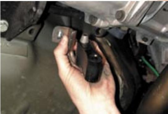
70. Install dog bone rubber hanger to bracket. Use lubricant for easy installation.
