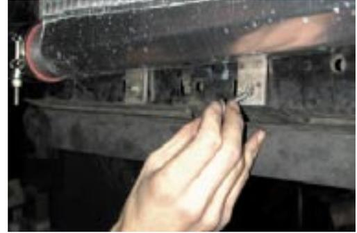
93. Install intercooler support strap, hang strap from hood latch and secure with supplied 5/16" hardware.
