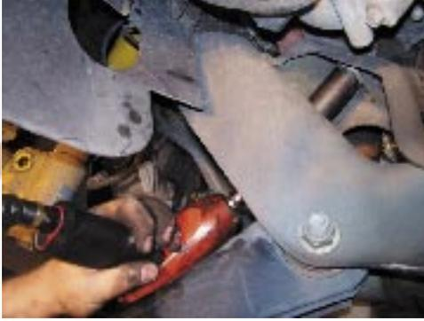
18. Support engine and transmission with appropriate upper support tool or support from beneath.
