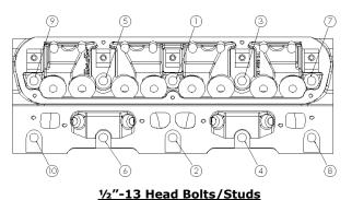
Stage 1: 40 ft.-lbs. Stage 2: 70 ft.-lbs. Stage 3 *Bolts*: 100 ft.-lbs. Stage 3 *Studs*: 110 ft.-lbs.
