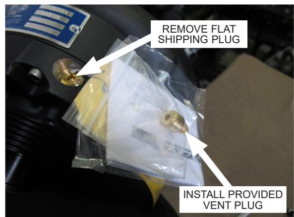
Fig. 3-F: Remove shipping plug and install vent plug
