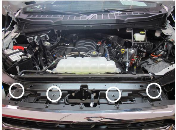
Fig. 1-P: Remove upper grill screws
