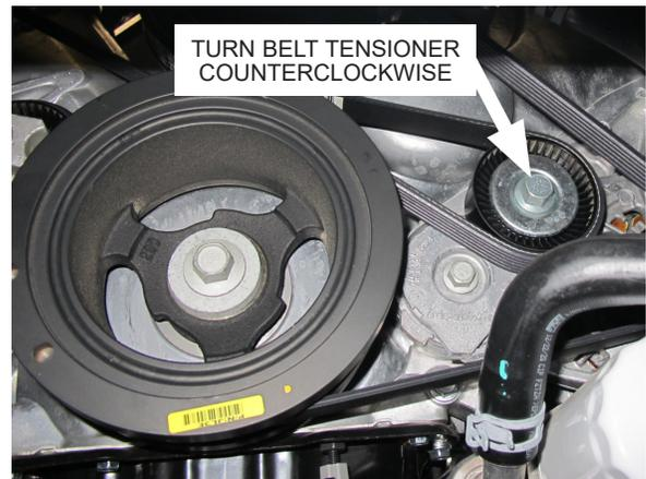
Fig. 1-E: Remove OEM serpentine belt
