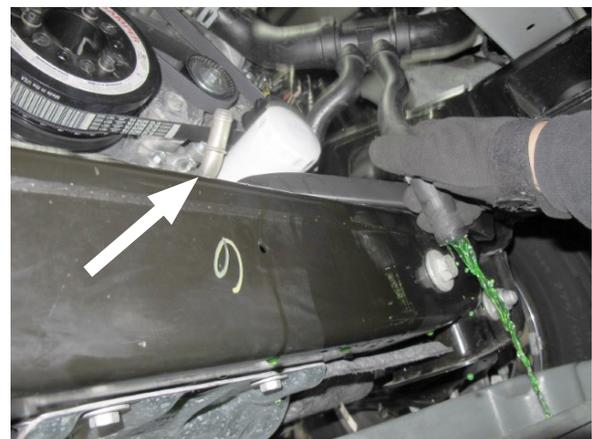
Fig. 1-F: Remove cap and drain coolant
