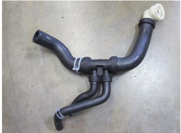
Fig. 1-G: Remove coolant hose assembly
