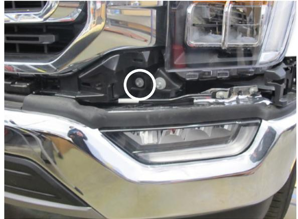
Fig. 1-S: Remove grill lower screws
