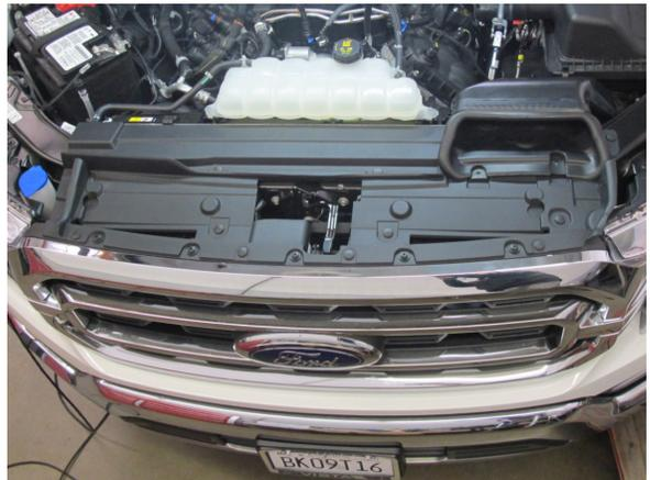
Fig. 9-H: Reinstall radiator support cover
