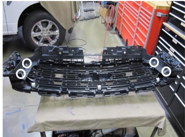
Fig. 2-E: Reattach shutter housing to grill
