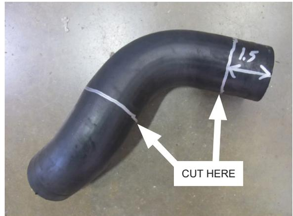
Fig. 2-G: Mark and cut coolant hose
