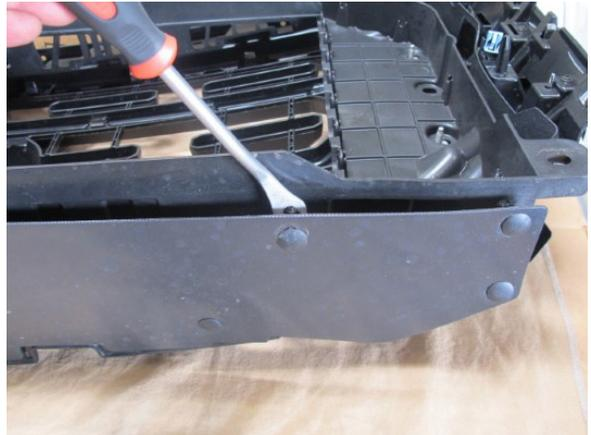
Fig. 1-V: Remove grill lower flap
