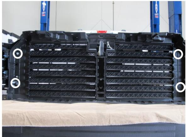
Fig. 1-W: Remove grill nuts
