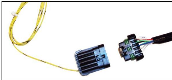
Figure 19 IGN (Shown with Tach Out Adapter Harness)
