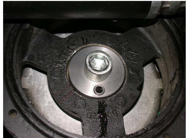
Fig. 3-a (Supplied Drill Guide Tool)
