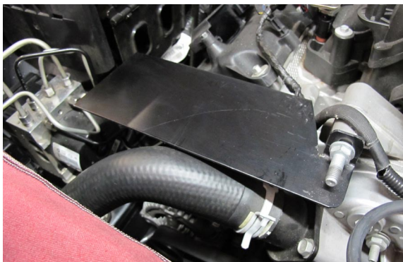
Fig. 8-e (CAC Support Bracket, Installed)
