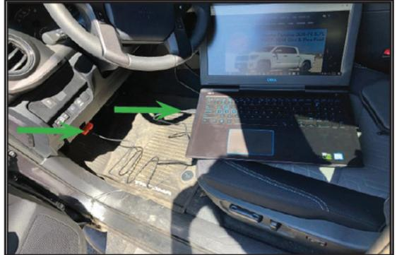
18. Turn the ignition switch to the on position (**Engine off**). On Tacoma's / Tundra's with a push button start **DO NOT** depress the brake pedal and push the start button **twice**. Click on Flash ECU icon shown with the arrow.
