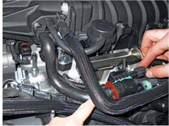
9. Install the connector to the EECPV. Install the purge line (with green connector) to the EECPV. Zip tie the EECPV to the engine harness.
