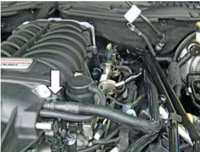
7. Connect the booster hose (1318-9D0692) to the supercharger and secure it with one (1) clamp (7329K11, found in 1318-TVSHWKD).
