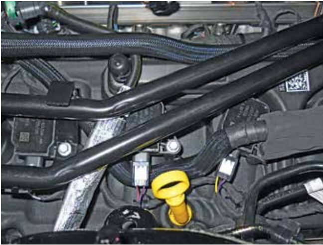
7. Connect the booster hose (1318-9D0692) to the supercharger and secure it with one (1) clamp (7329K11, found in 1318-TVSHWKD).
