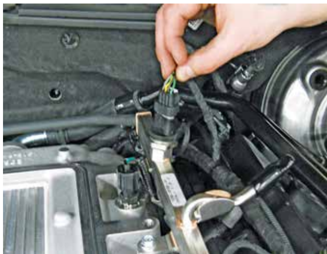
15. Plug in the connector to the fuel pressure sensor on the fuel rail.
