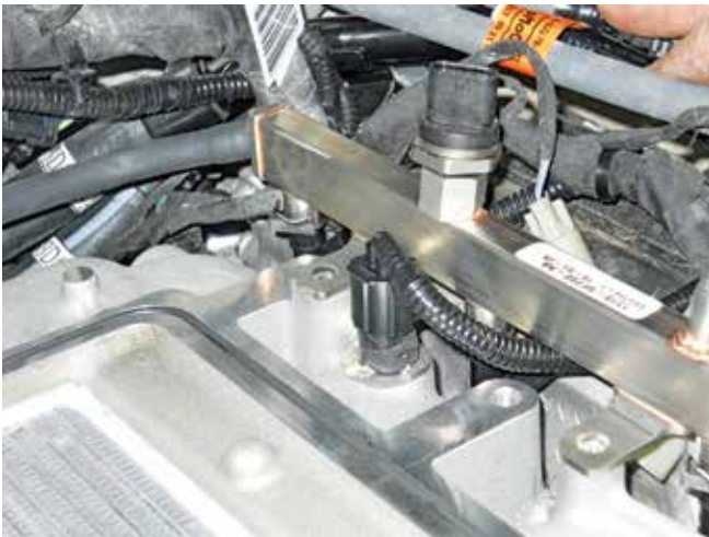
12. Lubricate the lower fuel injector O-rings with petroleum jelly or engine oil. Install the fuel rail and injectors into the intake manifold. Be sure each injector is properly seated into the intake manifold. Install three (3) previously removed fuel rail mounting bolts into three (3) of the four (4) fuel rail mounting locations (positions 1, 3 and 5 in the figure).
