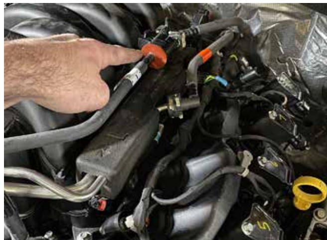
12. Disconnect the VMV (evaporative emission canister purge valve) tube and electrical connector. Remove the VMV tube retainer from the fuel rail and fuel supply line.
