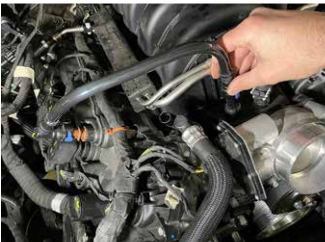
11. Disconnect the throttle body electrical connector as shown. (Pull the red locking tab back; press the black release tab to disengage the lock.) Remove the four (4) throttle body mounting bolts with a 8 mm socket and set the throttle body and fasteners aside for later.
