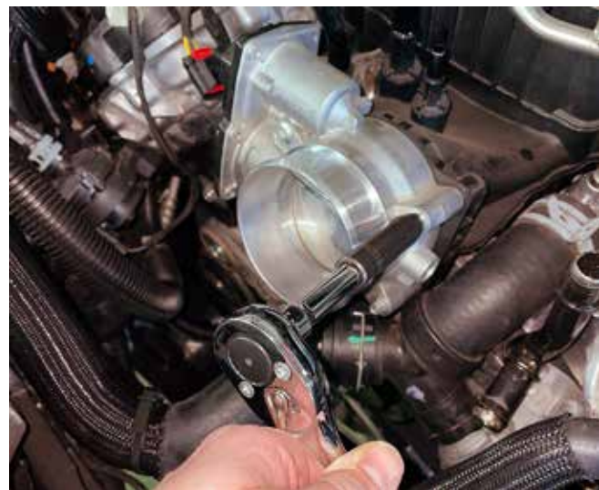
12. Disconnect the VMV (evaporative emission canister purge valve) tube and electrical connector. Remove the VMV tube retainer from the fuel rail and fuel supply line.
