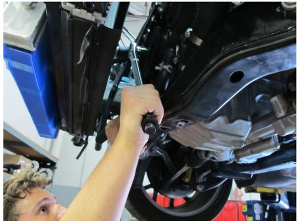
Fig. 5-B: Remove crank bolt
