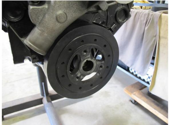
Fig. 1-D: Remove crank pulley and/or accessories from harmonic balancer
