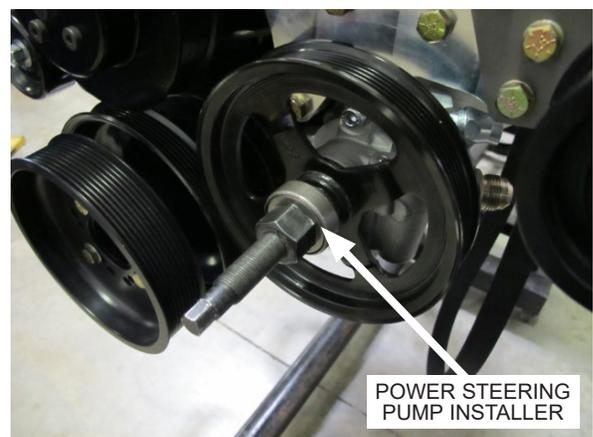
Fig. C: Power steering pump pulley installer tool
