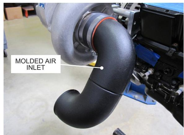
Fig. 8-C: Install molded air inlet to supercharger inlet
