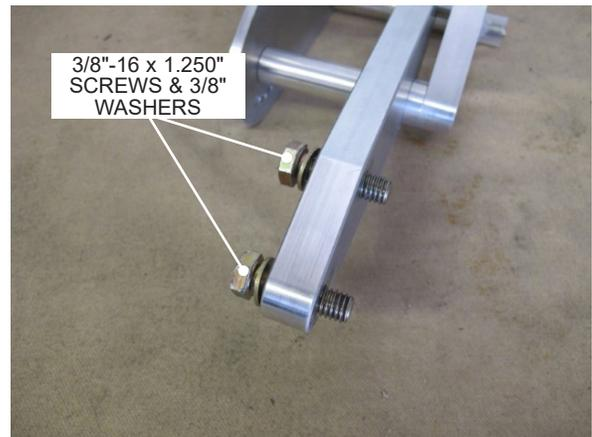
Fig. 4-E: Remove hardware
