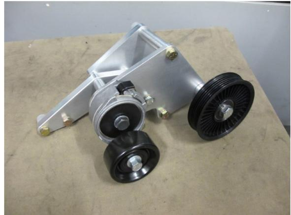
Fig. 3-B: Ribbed idler pulley (Vehicles without A/C only)
