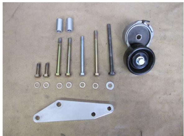
Fig. 4-I: Components to be reused
