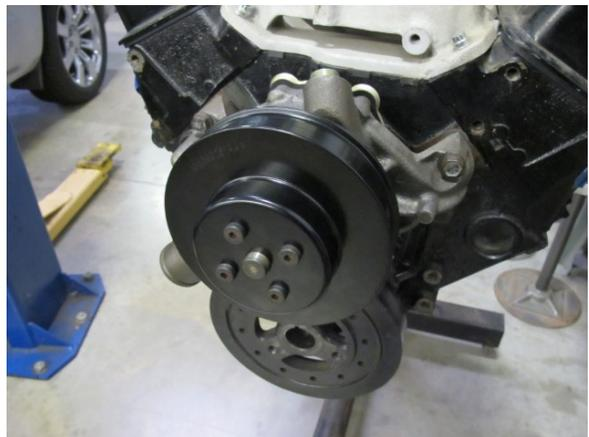
Fig. 1-C: Install water pump pulley
