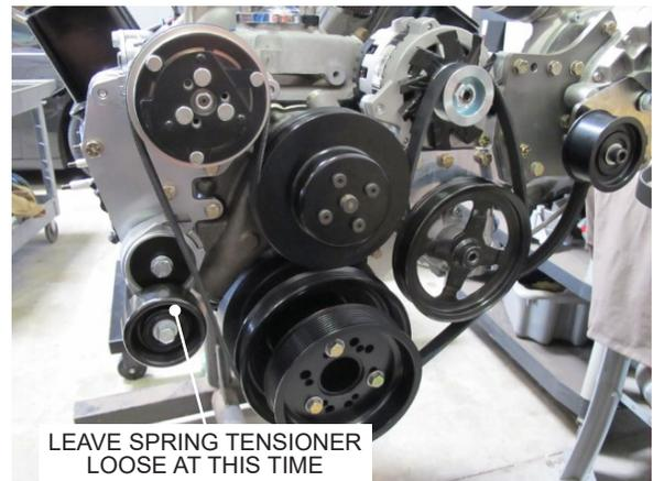
Fig. 5-H: Install accessory drive belt
