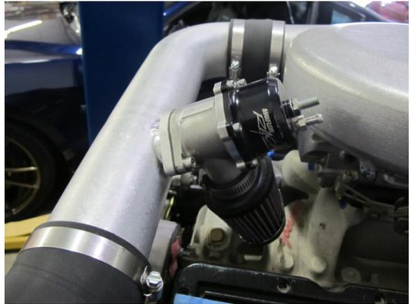
Fig. 7-J: Install bypass
