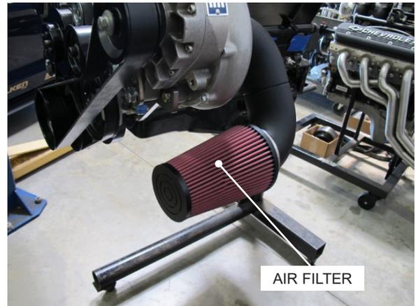
Fig. 8-D: Install air filter to molded inlet
