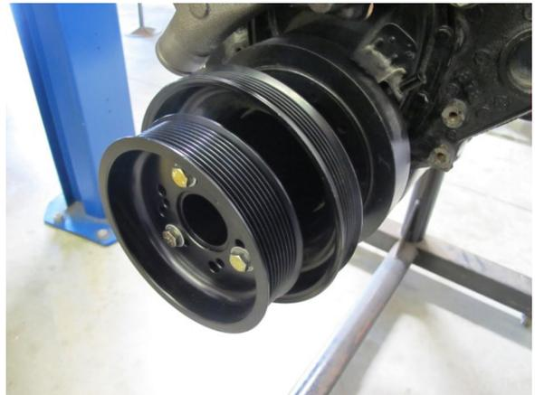
Fig. 5-E: Install belt drive assembly with accessory pulley to harmonic balancer
