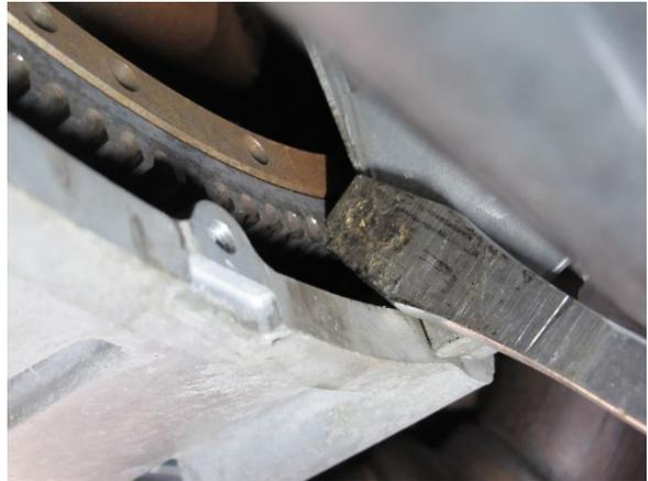
Fig. 5-A: Keep the engine from rotating
