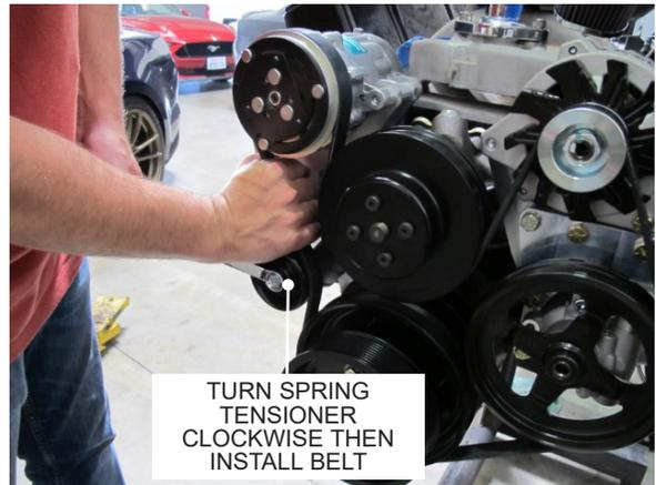
Fig. 5-J: Tension accessory drive belt
