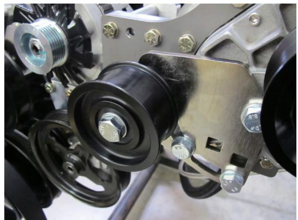
Fig. 6-C: Install flanged idler pulley
