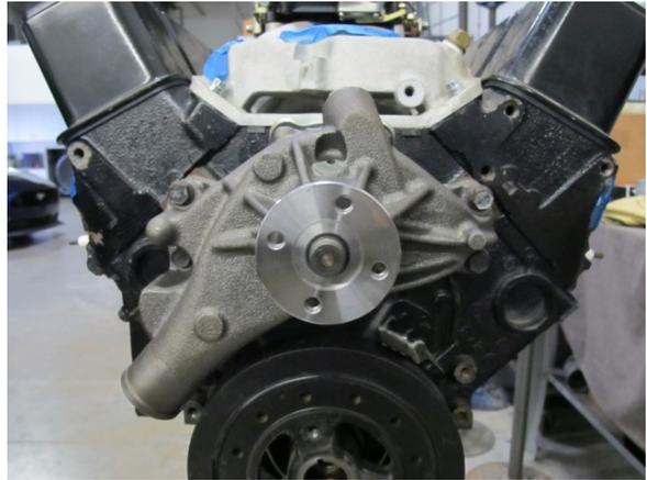
Fig. 1-B: Install water pump
