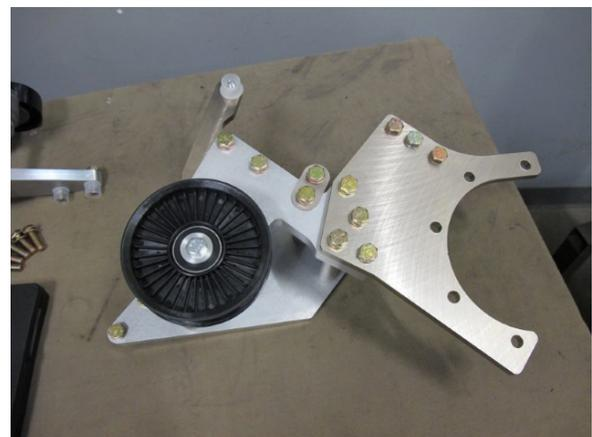
Fig. 2-C: Supercharger mounting bracket assembly
