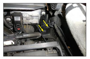
92. Gather the bracket shown below and install it at the two threaded studs and tighten in place with the original nuts.
