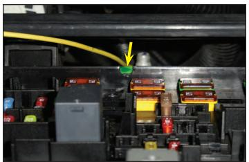
101. Notch the positive terminal cover to allow the yellow trigger wire some clearance.
