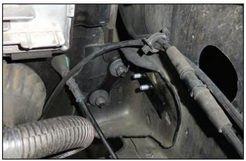
93. Gather the provided intercooler pump harness and install the provided 15A fuse. Reinstall the cover once you are done.
