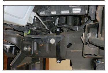
81. Install the coolant pump with the two provided Adel clamps and two M8 nuts at the yellow arrow locations. Ensure that the pump output barb is facing the direction of the green arrow. Ensure that the lower Adel clamp is about 1/2 inch from the bottom as shown. Be careful not to over tighten the M8 nuts, this can cause the Adel clamps to bend.
