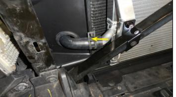
89. Install the provided 29" mesh over the provided 3/4" hose that is 27" long as shown.
