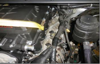
144. Gather the M6x35mm bolts and apply Loctite 242 to them as shown below. Install the driver's side front bolt first. Use a magnetic telescoping pick up tool to install the 8 supercharger mounting bolts as shown here.
