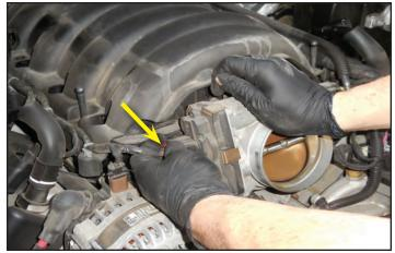
21. Pull the four "tree" tab wire loom mounting anchors from the holes in the right, and left side of the intake manifold.
