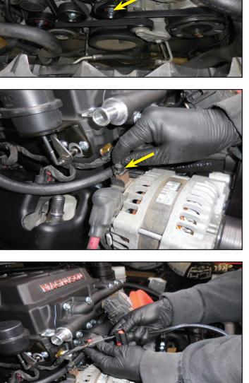
173. Plug the ETC wire extension from the last step into the throttle body and secure with the locking mechanism.
