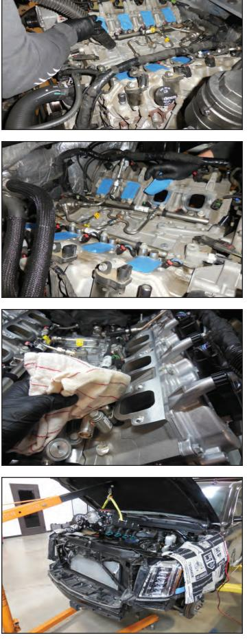
141. Remove the two bolts (shown with yellow arrows), if you haven't already done so, holding the plastic ramp that directs the electrical harness shown in the green highlighted area. Also cut the two cable ties shown with red arrows)
