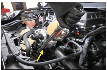
169. Use a strap wrench to hold the supercharger pulley in place while you torque it to 108 in-lbs using a 10mm socket wrench.
