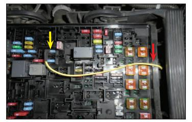
105. You will need to use needle nose pliers to push the fuse down tight into its location. Make sure the fuse is sitting evenly and not crooked.
