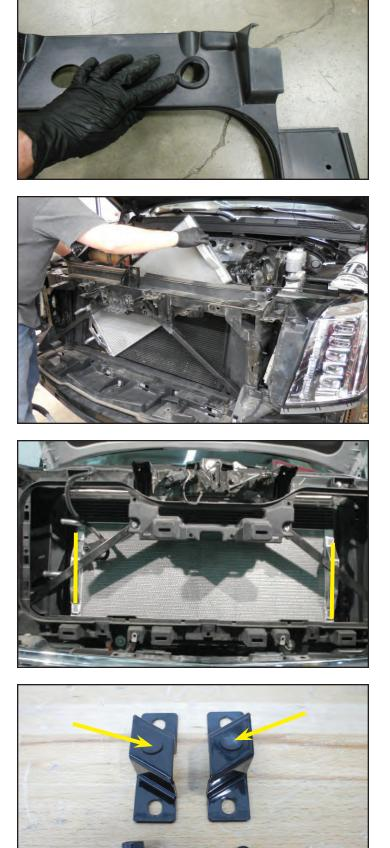
69. Attach the mounting brackets to the LTR mounting flange using the supplied bolts and a 12mm wrench. Do not tighten until you have aligned the LTR to be level, cross checking against the existing horizontal lines of the A/C condenser. Secure in place when you've got
