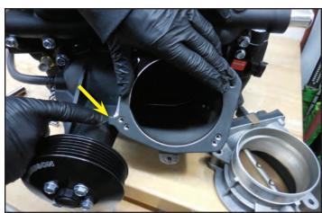
133. Rotate the throttle body so that it fits on the upper right most hole as shown, then line up all the other holes while you hold the gasket in place.
