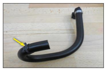
157. Install the connector from the hose assembly in the last step onto the PCV valve. You should hear a click to indicate the connector is locked. Pull up to make sure the lock is engaged.
