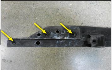
57. Pull up on the upper radiator shroud to unsnap it from the retaining slots, set aside for later re-install.
