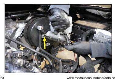
73. Replace the nuts incorporating the reservoir assembly. Torque to 25 ft-lbs. Verify your torque wrench settings.
