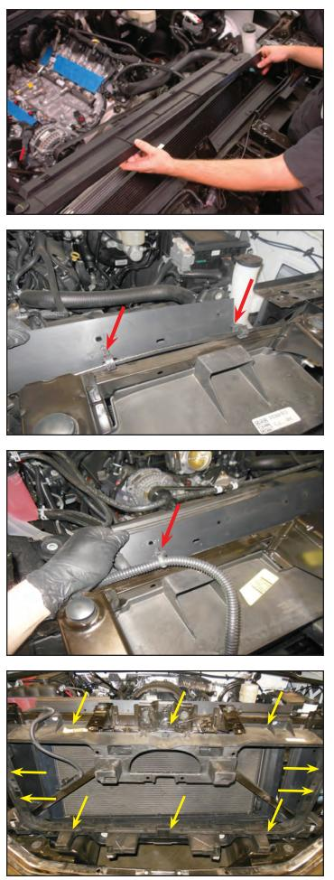
61. Here you can see the three lower locations after the rivets have been removed.
