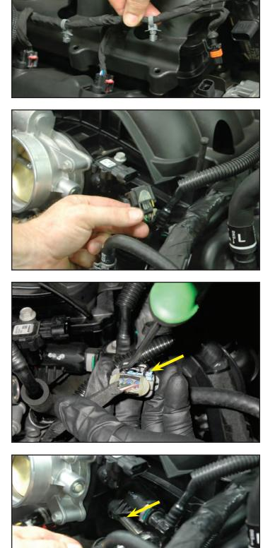
25. With the EVAP Solenoid free you can now remove the electrical connection by pulling back, then pressing the release tab and unplugging.
