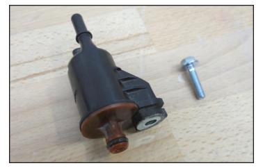
161. Install the EVAP solenoid in the location shown and secure it with the M6x25mm bolt at the yellow arrow. Plug in the electrical connection at the red arrow and the hose connection at the blue arrow.
