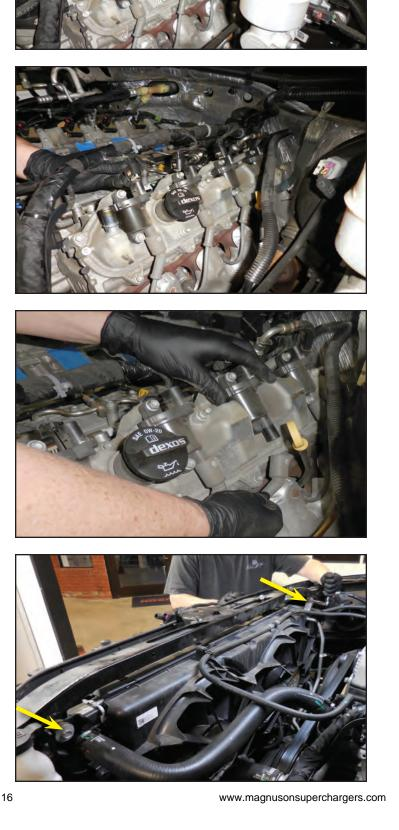
45. Remove the support bracket by unscrewing the two bolts shown with arrows using a 10mm socket wrench. Repeat this process on the passenger side.
