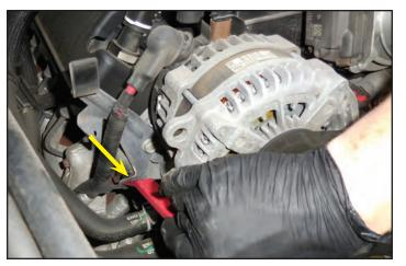
17. **This does not apply to the 2017 or newer Sierra/Silverado.** Remove the bolt securing the bracket in location shown using a 13mm socket wrench.
