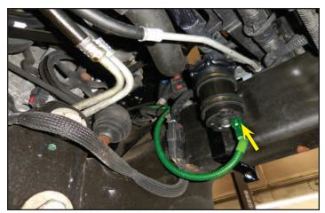
97. Route the intercooler pump ground wire (highlighted in green) above the brake booster housing. Remove the factory nut at the grounding location shown with the arrow using a 10mm socket wrench and place the eyelet from the coolant pump ground wire on the stud. Reinstall the nut to secure the two ground wires.
