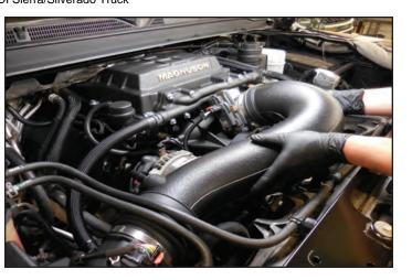
201. Install the 90° fitting of the hose assembly from the last step onto the passenger side valve cover and press the white locking button. Connect the straight fitting from the hose assembly in the last step onto the inlet air tube where shown and press the white locking button. Pull at each connection to make sure the locks are engaged.
