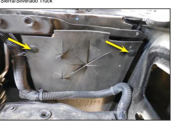
53. Remove the cross-frame support brace center bolt using a 13mm wrench.
