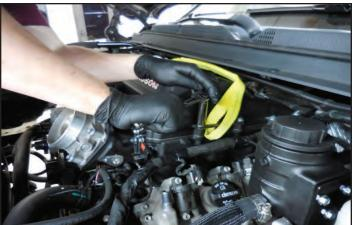
149. Apply Loctite 242 to the 4 lid bolts from the last step. Reinstall the bolts in their original location and **torque them to 18ft-lbs**.
