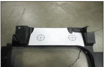
65. Install the two provided grommets at the hole locations. Now re-install the panel back into its original location using the OEM push rivets.
