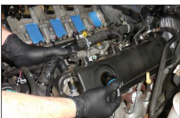
41. Remove the plastic coil cover and reinstall the oil filler cap. Remove the coil cover on the passenger side as well.
