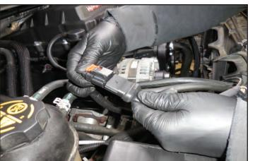
181. Remove the cable tie fastener from the arrow location and cut it free from the wiring.
