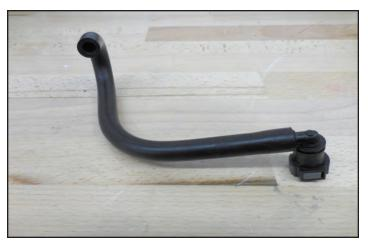
154. Insert the 90° fitting into the hose end and orient as shown.
