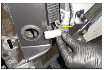
85. Slide the hose from two steps ago through the grommet and over the lower LTR hose barb and secure with the clamp as shown. The short elbow end connects to the LTR shown here.
