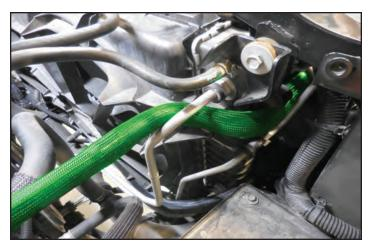
189. Route the hose from the last step under the air box tube as shown highlighted in green.
