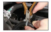
182. Insert the provided cable tie fastener into the location from the last step.
