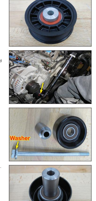
114. Apply Loctite 242 to the supplied bolt as shown below. Install the pulley with the spacer at the backside in the arrow location shown and torque to 25 ft-lbs.
