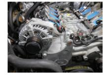
111. Remove the bolt shown with an arrow using a 15mm socket wrench. This will be replaced with a longer bolt to install an idler.
