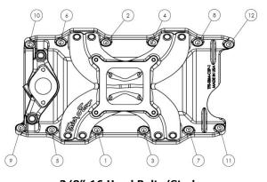
3/8"-16 Head Bolts/Studs Stage 1: 16 ft.-lbs. Stage 2: 22 ft.-lbs. Stage 3: 30 ft.-lbs.
