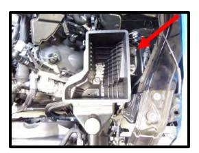
28. Pull the (2) push pins securing the engine harness to the frame on the driver side, this will be reused later to secure the airbox.
