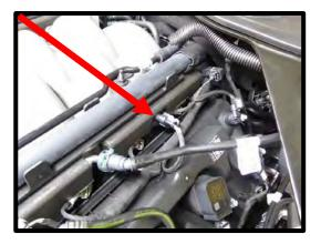
33. Carefully disconnect the factory fuel feed hose from the fuel rail. The fuel system may still have pressure, use protective eyewear and multiple rags to catch any possible fuel leak. To release, press the blue safety latch and pull the fuel fitting away from fuel rail.
