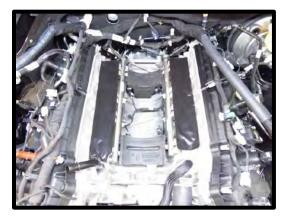
40. Remove the coolant to heater tube overflow hose using a pinch clamp tool. Pull away from heater tube.
