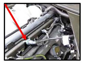
34. Using a 3/8" fuel line removal tool, remove the DI pump fuel feed line from PI fuel rail.
