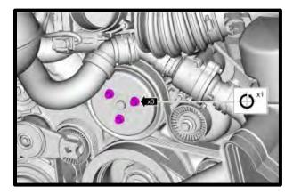
43. Remove the belt from the engine by using a 15mm socket on a ½" breaker bar and rotating the spring-loaded tensioner in a clockwise direction.
