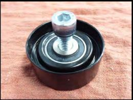
68. Assemble the spring-loaded tensioner by mounting the supplied spacer with the female register to the tensioner. Install the grooved idler pulley (#36326) to the tensioner and (.390") step spacer. Use the supplied step washer to center the bearing and the 10mm x 40mm SHCS (10-Rib uses 10mm x 60mm SHCS) bolt to secure idler to tensioner. Use light amount of anti-seize on threads. Torque to 18 lbs-ft.
