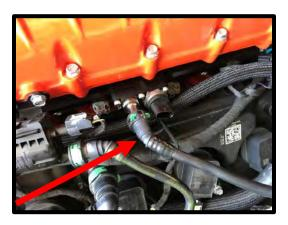
95. Connect the factory fuel PSI sensor connector to sensor, press safety lock until it clicks and locks in place.
