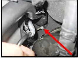
23. Disconnect and remove the positive crankcase ventilation PCV tube from inlet tube and LH cam cover fitting.
