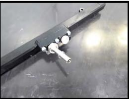
84. Install the supplied (2) #2-906 orings to the (2) inlet/outlet fittings. Install these (2) fittings into rear side of fuel rails. Apply light amount of grease to oring for ease of installation. Using a ¾" wrench (or ¾" deep socket) on both the front and rear fittings, tighten both.
