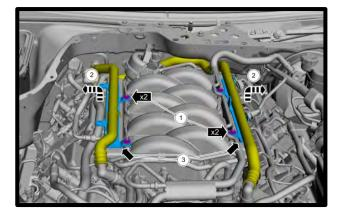
36. Loosen the 4 bolts holding the fuel rails down, these go through to the cylinder head (10mm socket). Fuel rail does not need to be removed.
