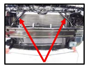
101. Using a panel puller, remove the (1) plastic pin holding the front snorkel to the radiator support. Using a hacksaw, cut the one side off as shown. Once cut, reinstall closeout using original plastic push pin.
