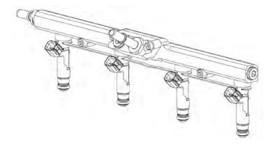
86. Apply generous amount of grease to the injector orings for ease of installation. Install the fuel injectors, rails and lock bracket to the intake manifold, secure with the (4) 6mm x 20mm SHCS using a 5mm allen socket. Torque to 90 lbs-in.
