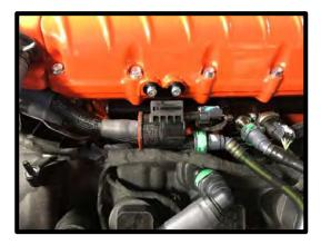
125. Install the supplied ¼" ID bypass actuator to the bypass nipple and ¼" nipple on SC housing. **CAUTION:** Do not open/close bypass actuator by hand. This may damage actuator internally. It only moves properly with equal vacuum/boost at the actuator reference port.
