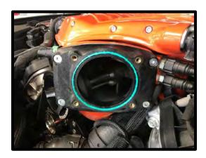
143. Install the stock throttle body using the (4) 6mm x 50mm FHSCS bolts using a 10mm socket.
