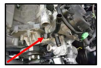
42. Loosen the (3) bolts securing the water pump pulley (while belt is on) using a 10mm socket.
