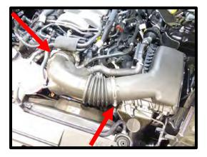
27. Remove the airbox bottom by removing the (1) bolt on the driver side inner fender (10mm socket).
