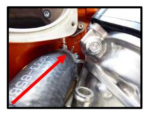
54. Install the supplied ¼" formed hose from the water neck vent line, route towards the overflow tank for later installation. Secure with stock clamp. NOTE: Shown with SC on for routing direction.
