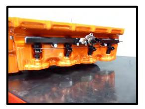
87. Install the supplied fuel cross over line around the back of the supercharger by pressing until they click and lock in place.
