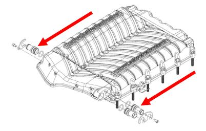
93. Connect the factory passenger side rail fitting to the DI pump factory hose, press until it clicks and locks in place.
