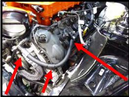
52. Install the factory coolant overflow hose to the new supplied tee fitting on the driver side. Secure using factory pinch clamp.
