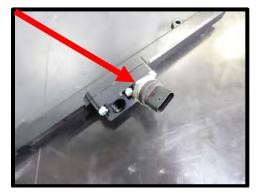
82. Install the supplied (1) #2-906 Viton oring to the (1 of 2) 45mm long 9.49mm inlet fitting. Apply light amount of grease to oring for ease of installation. Install fitting to the fuel inlet block.
