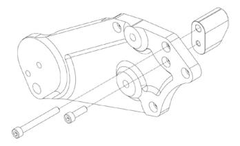
79. Torque the (10) 6mm x 55mm HHFCS manifold bolts in the following pattern using a 10mm socket. First pass: 88 lbs-in. Second pass: 106 lb-in. **NOTE:** For bolt #10, a ¼" socket with 4"-6" extension, 10mm wobble is the best possible tool to get into this tight area.
