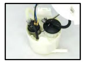
157. (Stage 2 and Up Systems) Reinstall the hat to the assembly in the center/buckets assemblies and connect the electrical connector harness to the hat assembly.
