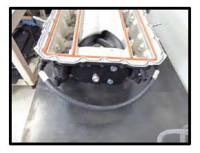
88. Using the supplied 5/16" OD silicone tube, install the (1) 60 1/2" cord around the perimeter receiver groove. Bunch it up so it has no gap at the end. Install the (2) 16" cords in the two middle sections, making sure it bunches up to perimeter cord. There should be no gaps.
