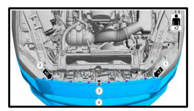
13. If equipped, disconnect the front active shutters electrical connector behind the bumper support. Remove the (6) plastic plush pins securing shutter assembly to front of vehicle as shown. These will not be reused. Wrap the connecter up, cover with electrical tape and secure with zip-tie to factory harness.
