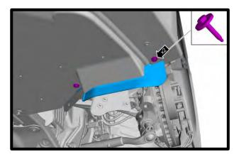
10. Remove the (19) lower close-out panel bolts (7mm socket) and the (2) push pins. Remove the lower close-out panel from vehicle.
