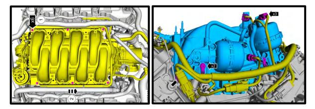
39. Clean the intake manifold to cylinder head surface using carb cleaner or acetone. Install tape over the exposed ports until manifold installation.
