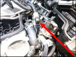
32. Disconnect the fuel psi sensor connector from driver side fuel rail.
