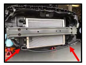
123. Mount the EECPV bracket to SC lid, use the (2) supplied 6mm x 10 HHFCS. Torque to 80 lbs-in using a 10mm socket.
