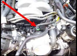
25. Disconnect the MAF connector by pulling back on the safety lock, then squeezing the unlocking tab and pulling back. Using a panel puller tool, remove the wiring harness support tab from the airbox.
