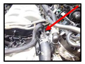
31. Remove the heater hose from both driver and passenger side of block by pulling locking tab back and pulling away. Push to the back of the engine for later use.
