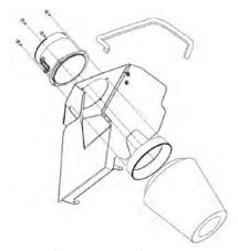
135. Install the factory MAF sensor element into the new MAF housing using the supplied (2) 4mm x 6mm SHCS. Torque to 17 lbs-in. \*\*DO NOT USE STOCK BOLTS\*\*. \*TIP: Verify arrow position for airflow direction.
