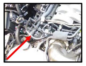
19. Pull apart the rubber shielding securing vacuum lines together.
