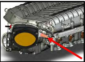
128. Install the supplied 3/8" ID x 5 ½" hose factory EECPV barb fitting and **upper** quick connect fitting on SC inlet. Push until it clicks and locks into place.
