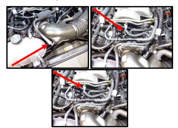
21. Using a pinch clamp tool, remove the brake booster line that connects the brake aspirator rubber line to hard line.
