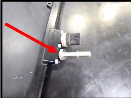
83. Install the supplied (1) #2-906 Viton oring to the (1 of 2) 45mm long 9.49mm outlet fitting. Apply light amount of grease to oring for ease of installation. Install fitting to the fuel inlet block. Install the supplied -6 ORB plug to the extra port.
