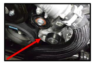
45. Remove the water pump pulley using a 10mm socket (this will be reused).
