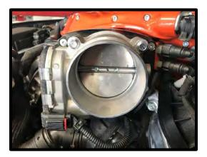
144. (Whipple 132mm Crusher throttle body) Install throttle body to supercharger inlet, use the supplied gasket between TB adapter and SC inlet. Secure with the supplied (3) 6mm x 25mm SHCS and (1) 6mm x 50mm SHCS using a 5mm allen socket. Torque to 88 lbs-in.
