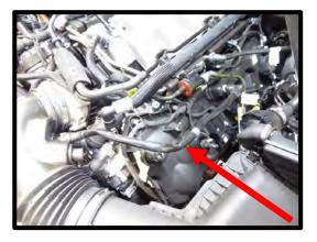
24. Disconnect the green connector from the evaporative emission canister purge valve (EECPV) tube and the electrical connector. Disconnect green connector securing EECPV line to intake manifold. Lift EECPV purge valve from intake manifold for later use.
