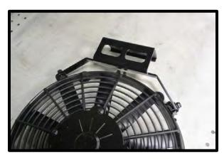
105. (**Dual fan installation**) Carefully set both fan assemblies on top front of the LTR, space these evenly before installing.
