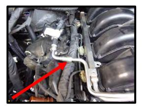
35. Remove the (4) nuts from the top of the intake manifold that secures the (2) heater hose trays and brake aspirator line. Use a 10mm deep well socket. Once bolts are removed, remove tray, brake aspirator and foam material.
