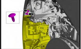
12. Carefully pull the fascia forward, disconnect the fog lamps before pulling away.
