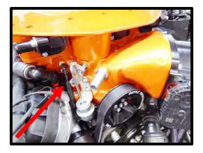
126. Install the (2) supplied 6AN viton oring (#906) to the (2) 6AN to 3/8" quick connect fittings. Install these fittings to the passenger side lower 6AN fittings on the inlet using an 11/16" socket.
