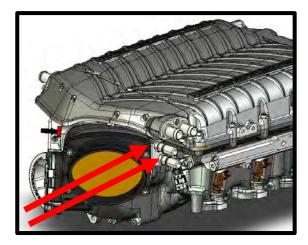
127. Install the supplied 3/8" ID x 24" brake aspirator hose from the brake booster to the **lower** quick connect fitting on the supercharger inlet. Push until it clicks into place. **TIP:** For best routing, nestle in between cam cover and fuel rail, under the wiring and heater hose.
