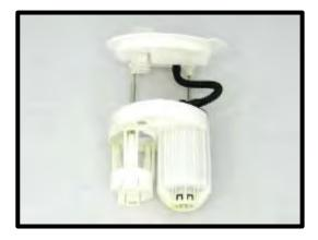
153. (**Stage 2 and Up Systems**) Remove the (3) locating tabs and smooth the pump receptacle to the diameter of the DW400 (46mm).
