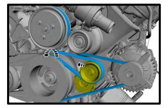
44. Remove the spring-loaded tensioner from the engine using a 13mm socket.
