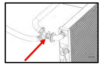
116. Connect the ¾" x 34.5" #3102697 hose to the Y fitting, secure with pinch clamp. Route other end to the RH side of the water cross fitting. Secure with the supplied worm clamp. For max hood clearance, ensure that the hex is not on top.
