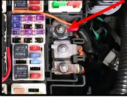
60. Pull the red 10amp fuse from position **#62** (ABS). Install the 10amp red fuse in the unused fuse slot on the fuse tap. Install the supplied fuse tap into position **#62** (ABS). **Note:** 10amp red fuse should be in bottom slot, 5amp should be in top slot. Make sure wire has enough room when fuse cover closes, route around fuses for clean installation.
