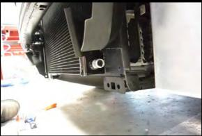
121. **(Standard LTR)** Route the 3/4" ID x 16" hose from IC pump outlet to LTR inlet. This hose has to go up and towards the tank as shown in the image. Failure to do so may cause clearance issues.
