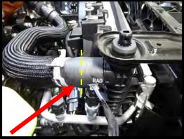
56. Remove the coolant vent hose from the radiator and pull back the plastic sheaving. Shorten this hose end by 1" for additional clearance. Reinstall hose using factory clamp.
