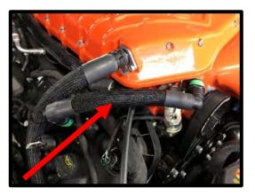
131. Install the supplied 5/8" ID x 21" hose to the driver side valve cover. Push until it clicks and locks into place. The other end will be installed in inlet tube later.
