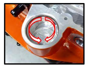
91. Apply generous amount of grease to the (1) #2-230 Viton bypass oring. Install the supercharger lid to the supercharger housing by carefully placing the bypass down. Secure the SC lid using the (17) 6mm x 30mm HHFCS and (3) 6mm x 70mm HHFCS (*marked green*) using the following pattern. Torque to 90 lbs-in using an 8mm socket.
