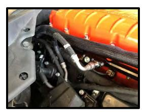
94. Connect the factory fuel inlet line to the driver side fuel fitting, press until it clicks and locks in place.
