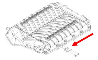
124. Slide the EECPV to bracket by sliding onto bracket. Connect factory plastic quick connect fitting to EECPV until it clicks and locks into place. Connect 2-way electrical connector to EECPV, press locking tab back in place.
