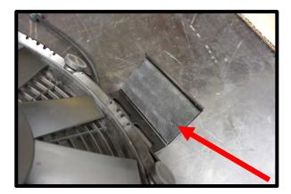
104. (**Dual fan installation**) Install the (4) brackets to the fans by sliding the square tab into the fan notch and the steel channel bracket will slide on the outside. The angled side will face the fan. This slides together easier if the bracket is facing slightly up. Once these are lined up, push until the seat together. Repeat on the other (3) brackets. Leave nyloc nuts loose for now.
