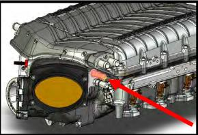
129. Install the (1) supplied 6AN viton oring (#906) to the (1) 6AN to 5/8" quick connect fittings. Install this fitting to the driver side 6AN fittings on the inlet using a 7/8" wrench.
