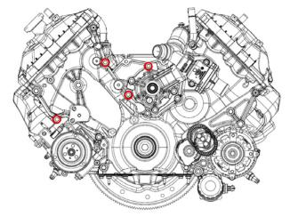
63. Install the (4) support stands to the front idler plate. These are loose fit; therefore, you must tilt backwards during installation or the stands will fall. You can use masking tape to help hold in place during installation if installation becomes difficult. *Each support stand is marked with an identifying number, as well as the idler plate for ease of placement*. TIP: Assemble together with the number facing out for future reference.
