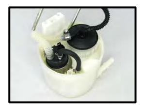
156. (**Stage 2 and Up Systems**) Install the new connector harness supplied with the DW kit, the additional static ground inserts into the slot on the assembly filter, the same as OE.
