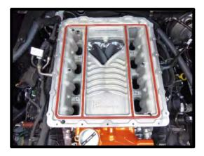
89. Install the supplied pre-formed 20.7" x .103" oring to the top sealing surface of the SC housing. Apply generous amount of grease to help ease the oring into place. **TIP:** To install oring into dove-tail groove, press vertically, vs sliding finger along.
