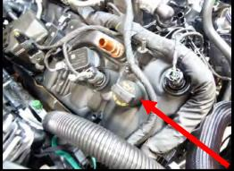
18. Remove the PCV purge line from the intake manifold and RH cam cover. One of these 90deg connectors will be reused.
