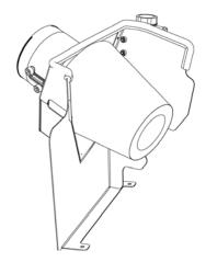
137. Install the intercooler filler neck to the (2) aluminum threaded stands using the (2) 6mm x 45mm BHFCS (4mm allen socket).
