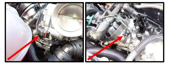
30. Remove the vent hose coming from the thermostat housing fitting by removing pinch clamp. Remove vent line from overflow tank by removing pinch clamp using a pinch clamp tool. This hose will not be reused.
