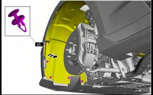
9. Remove the push pins from the (2 per side) push pins securing inner fender well to undertray.
