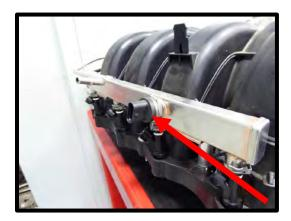
47. (Stock throttle installations) Remove the throttle body from the manifold by removing the (4) bolts using a 10mm socket
