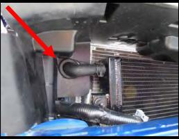
115. Route the supplied 90deg intercooler feed hose #COYO-2006 through the grommet, cut to fit as needed. Install the supplied Y fitting to the end of the hose from the outlet of the LTR, just after the grommet. Secure hose to fitting with pinch clamp.
