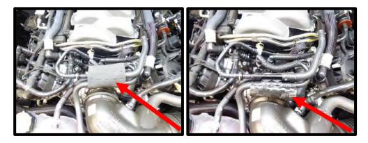
20. Disconnect and remove the brake aspirator lines from the inlet tube and intake manifold.
