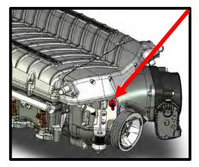
130. Install the supplied 5/8" ID x 8 ½" hose to the passenger side valve cover. Connect other end to the supercharger inlet quick connect fitting. Push until it clicks and locks into place.
