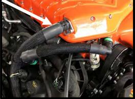
117. Install the supplied preformed ¾" x 48" dual 90deg hose #3102698 to upper Y fitting and secure with pinch clamp. Route up and over the condenser to LH side of vehicle. Leave this end loose until airbox installation. Secure hose to factory holes using zip-tie to prevent hose from sitting on AC Condenser.
