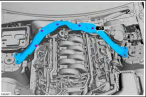
17. Rotate the oil fill tube counter clockwise and remove from engine. Remove the oil fill cap from tube. Reinstall cap into valve cover until it locks in place.
