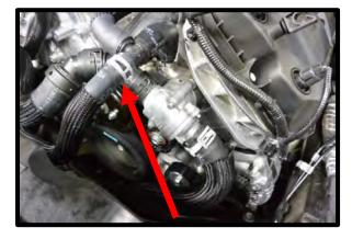
53. Using needle nose pliers, rotate the factory pinch clamp at the water neck towards the driver side for future clearance of the SC. **NOTE:** Image shows clamp with SC installed to illustrate max clearance.
