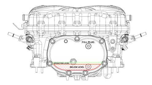
77. Install the supercharger housing (without lid) to the engine. Use the supplied (4) 6mm x 55mm HHFCS on the outer bolt holes and the (6) 6mm 55mm HHFCS bolts with the supplied (6) #2-009 orings on the bolt, under the head. Use **Blue Loctite #243** to the threads of each bolt. Leave hand tight for now.
