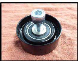
67. Remove the factory plastic smooth idler pulley from the engine. Replace with the supplied steel idler pulley. Use the factory fastener to secure. Torque to 18 lbs-ft with a 13mm socket. **NOTE:** Image shows proper direction of idler assembly.
