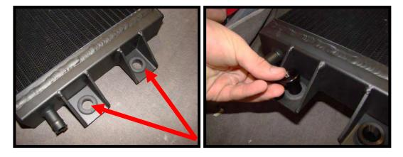
109. Install the LTR brackets to the LTR using the supplied (4) 8mm x 35mm FHSCS bolts through the aluminum heat exchanger spuds (5mm allen socket).
