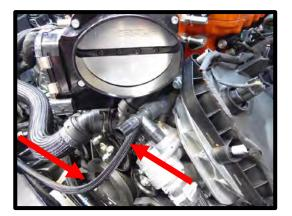
55. Remove the upper radiator hose from radiator. Use a hose cutter, remove 1" from the radiator hose end. Reinstall hose once completed and secure with factory hose clamp. TIP: This is for added clearance for the new belt system.
