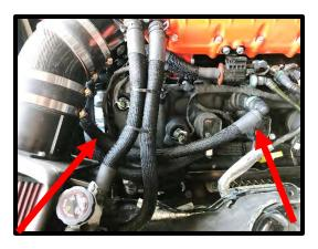
132. Install the supplied ¾" ID molded hose (#COYO-1300) from the IC **OUT** fitting to the airbox area for later installation. Secure end with supplied worm clamp. **TIP: For hood clearance, ensure that the nut of the clamp is not on top**.
