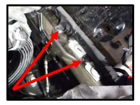
29. Carefully cut the electric tape securing the ETC wires to the throttle body. Disconnect the electronic throttle electrical connector by pushing up on the safety lock and then squeezing the connector and pulling away. Remove the harness support plastic tab from the block ground stud.
