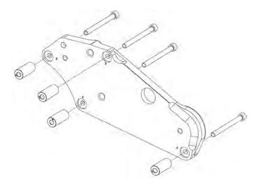
65. Preinstall the supercharger support bracket by installing on the back of the idler plate. Secure with the (1) 8mm x 70mm SHCS and (1) 8mm x 25mm SHCS, leave loose until supercharger assembly.
