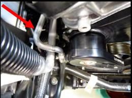
70. Install the spring-loaded tensioner to idler plate, locating the tang into position. Secure with the supplied (1) 10mm x 60mm SHCS. Use light amount of anti-seize on threads. Torque to 25 lbs-ft.
