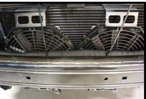
114. With the LTR mounted, mark the centerline of the LTR fitting and horizontally center of the plastic radiator (passenger side) shrouding. Using a 1 ½" hole saw, drill a hole through the plastic shrouding. Install the supplied 1 ½" rubber grommet into this hole. **NOTE:** Install hole and grommet as close to the plastic edge as possible. This gives proper clearance on the opposite side for the Y fitting.
