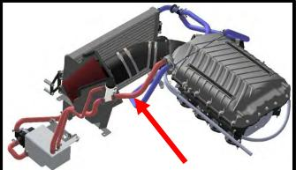
139. Install the supplied 3/8" ID x 31 ½" IC vent line (COYO-1400) and the ¾" ID x 24 ½" IC rubber hose (COYO-1300) to the filler neck. Both use the 90deg on the filler tee. Secure both with supplied pinch clamps. Route both below the airbox, to the IC reservoir. Secure both ends with supplied pinch clamps. Use multiple zip-ties to secure hoses together. Watch for hose kinks!
