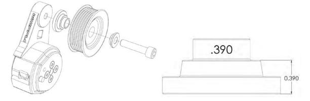
69. Carefully bend the factory AC line down and towards passenger side. Install spring loaded tensioner to plate to check clearance. You should have a minimum of 3/8" of clearance from the tensioner to the AC line.
