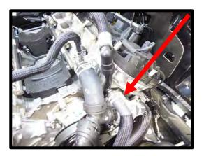
41. Remove the driver side heater tube from engine by removing the (1) bolt using an 8mm socket.
