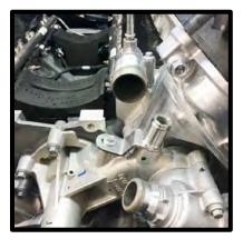
50. Install the supplied tee and 90deg hose to the driver side heater tube you just installed. Secure with the supplied pinch clamp on the 90deg hose to heater tube. **NOTE:** Short end of 90deg goes on heater tube, long end goes on tee fitting.
