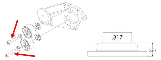
72. Install the (1) #2-109V75 oring to the MAP sensor block off and apply light amount of grease to oring. Install the MAP sensor port with the supplied block off plate, secure using the supplied (1) 6mm x 16mm SHCS. Torque to 70 lbs-in.
