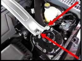
15. Using a flat head screw driver, remove the (2) plastic cups exposing the fasteners below. Using a 10mm socket, remove the (2) bolts securing cover to engine. Lift and remove cover from the engine.
