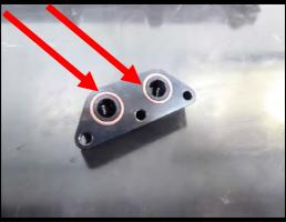
81. Using a 27mm socket, remove the fuel PSI sensor from the factory fuel rail. Install the factory fuel PSI sensor to the adapter using a 27mm socket. Torque to 53 lbs-in, then an additional 25-degree rotation. **NOTE: No sealant on the threads.**
