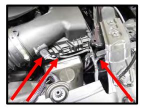
26. Loosen the factory air box lid by pushing the (2) locking tabs back. Loosen both hose clamps on the inlet tube (7mm nut driver). Remove tube, airbox lid and filter element from vehicle.
