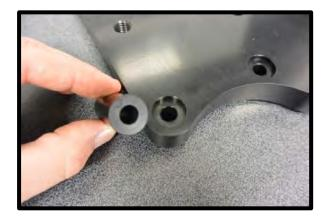
64. Use the supplied (4) 8mm x 90mm SHCS to secure the idler plate to the front of the passenger side of engine, install hand tight. Using a 6mm allen, torque to 22 lbs-ft.
