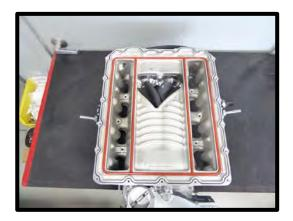
90. Install the (1) #2-230 internal bypass oring to the lid bypass passage. Use generous amount of grease to secure oring in place.
