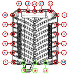
92. Install the supplied (3) intercooler cross-over inlet/outlet fittings and mounting fork to cross-over. Apply light amount of grease to orings for proper installation. Use the supplied (2) 6mm x 10mm HHFCS to secure mounting fork. Torque to 85 lbs-in using a 10mm socket.
