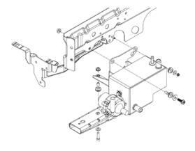
120. **(Standard LTR)** Using a hacksaw, notch the plastic shrouding next the heat exchanger inlet fitting. Use the supplied <sup>3</sup>/<sub>4</sub>" ID x 20" hose with 90deg end for test fitting (from pump outlet to LTR inlet).
