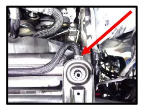
57. (Complete kits) Connect the supplied 3-way to 2-way air charge temperature pigtail at the rear of the passenger side cylinder head to the 3-way IMRC connector (Yellow, Orange, Green wires). Route to the RH side of the engine for later installation. NOTE: This will not work on competition or non-Whipple calibration systems. For competition-based systems, you will be required to supply your own method of monitoring post intercooler temperature.
