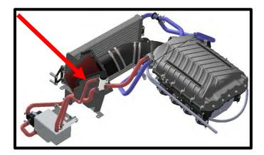
140. Install the previously routed hose from the Y fitting, to the LH core inlet fitting. Secure with worm clamp. **TIP: For hood clearance, ensure that the nut of the clamp is not on top**. Secure inlet and outlet lines with zip-ties for clean installation.
