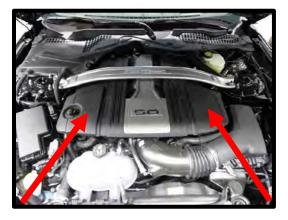
16. Remove the upper cowling for K-brace access. Remove the (7) push pin retainers and (2) tabs on the cowling. Lift up the cowl trim panel and remove the (4) nuts and (5) bolts from the K-Brace using a 13mm socket, remove from vehicle for later installation.
