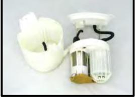
152. (**Stage 2 and Up Systems**) Carefully cut the larger pump outlet hose (3/8" ID) from the assembly filter and remove the OE pump.
