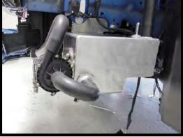
122. **(HD LTR)** Use the supplied ¾" coupler and (2) pinch clamps to couple the ¾" x 20" hose to the ¾" x XX" extension. Route the 180deg end to the LTR inlet. Secure using pinch clamp.
