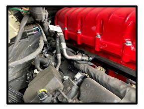
67. Connect the factory fuel inlet line to the driver side fuel fitting, press until it clicks and locks in place. Connect factory fuel psi sensor connector to sensor, press safety lock until it clicks into place.
