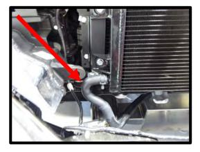
92. Connect the ¾" ID molded/formed (33") hose (#18F150-HS009A) from the LTR driver side bottom fitting that you previously installed, to the IC pump outlet barb. Secure with supplied pinch clamp. **NOTE: Ensure that this hose cannot kink or rub anything overtime.**
