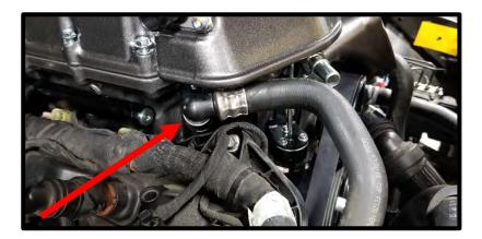
75. Connect factory heater hoses to previously installed plastic water fitting (bank 2).
