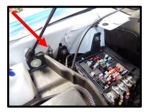
110. Pull the red 10amp fuse from position #F17 (ABS). Install the 10amp red fuse in the unused fuse slot on the fuse tap. Install the supplied fuse tap into position #F17 (ABS). **Note:** 10amp red fuse should be in bottom slot, 5amp should be in top slot. Make sure wire has enough room when fuse cover closes, route around fuses for clean installation.
