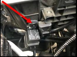
108. Using a 10mm socket, remove the nut on the power stud, located on the positive battery connector. Install the IC pump relay power eyelet (red wire) to the power stud on the battery positive (+) stud. Use a 10mm socket to secure stock and IC power wire.
