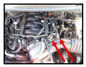
13. Remove the driver side valve cover PCV line quick connect fittings from the inlet tube by squeezing the connector and pulling away. Remove from valve cover by squeezing the connector and pulling away.
