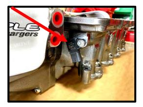
57. Install the supplied (8) manifold orings into the Whipple intake manifold.
