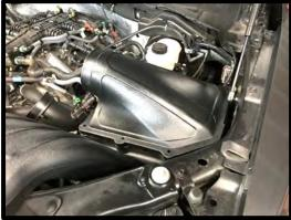
103. Install the (1) supplied 13/16" to ½" rubber grommet into the supercharger inlet tube. Install the supplied ½" to 15.82mm quick connect fitting.
