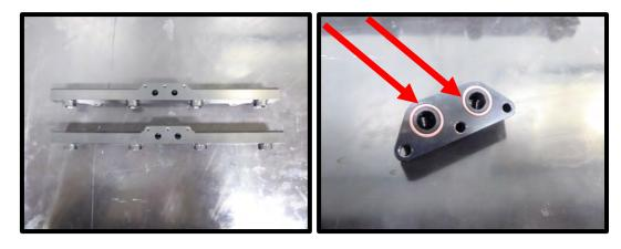
44. Using a 27mm socket, remove the fuel PSI sensor from the factory fuel rail. This will be reused at a later step. Install the factory fuel PSI sensor to the adapter using a 27mm socket. Torque to 53 lbs-in, then an additional 25-degree rotation. **NOTE: No sealant on the threads.**
