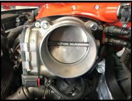
97. (Stage 2 Whipple 132mm Crusher throttle body) Install throttle body to supercharger inlet, use the supplied gasket between TB adapter and SC inlet. Secure with the supplied (3) 6mm x 25mm SHCS and (1) 6mm x 50mm SHCS using a 5mm allen socket. Torque to 88 lbs-in.
