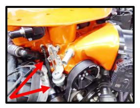
53. Install the (3) supplied 6AN viton orings (#906) to the (1) 6 ORB to 9.89mm and the (2) 6 ORB to 15.82mm quick connect fittings supplied. Bank 2 side, install (1) 15.82mm fitting to the lower port using a 7/8" deep socket and the 9.89mm fitting in the top port using a 11/16" deep socket. Bank 1 side, install (1) 15.82mm fitting to the lower port using a 7/8" deep socket. Install the supplied 6AN plug with oring to lower port, bank 1 using a 6mm allen.
