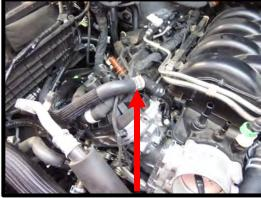
22. Disconnect the driver side heater tube quick connect fitting by squeezing and lifting away. Remove the heater tube overflow hose using a pinch clamp tool. Using an 8mm socket on the 1 factory bolt, remove the heater tube. Install the supplied oring to the shorter heater tube and install to factory location, secure with stock bolt, torque to 89 lbs-in. Reconnect both factory hoses.
