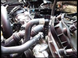
23. Carefully remove the factory fuel line by releasing the blue safety lock, then squeezing the connector and pulling back. The fuel system may still have pressure, use protective eyewear and multiple rags to catch any possible fuel leak. Remove the fuel PSI sensor electrical connector from the driver side fuel rail by releasing the white locking tab and squeezing connector, then pulling away
