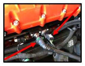
68. Slide the EECPV to previously installed bracket. Connect factory plastic quick connect fitting to EECPV until it clicks and locks into place. Connect 2-way electrical connector to EECPV, press locking tab back in place.
