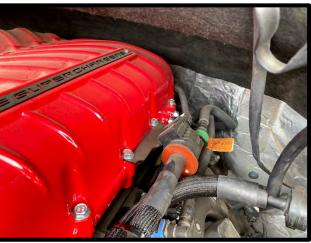
66. Connect the factory passenger side rail fitting to the DI pump factory hose, press until it clicks and locks in place. NOTE: THIS FUEL LINE HAS A CHECK VALVE, DO NOT FLIP ORIENTATION FROM STOCK DIRECTION. THE 90-DEG END ALWAYS CONNECTS TO FUEL FEED SUPPLY FROM FUEL RAIL! 30-DEGREE ALWAYS CONNECTS TO PUMP!
