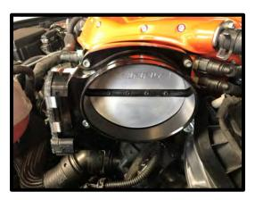
98. Connect the electronic throttle extension to the electric motor. Press until it clicks and locks into place. Press the safety lock until it clicks and locks into place. **NOTE: Secure harness to the intercooler line with a zip-tie to ensure proper clearance from the belt system.**
