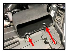
102. Install the supplied panel filter to the airbox lower. Install the upper airbox to the top of the filter. Secure the top to bottom using the supplied (6) 6mm x 16mm BHCS. Torque to 50 in-lbs. \*Caution: Over torqueing can result in pulling an insert out of plastic box.
