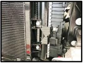
87. Reinstall new horn bracket and horns to factory location, using factory nut. Torque to 106 lbs-in. Zip-tie wire to factory harness for clean installation.
