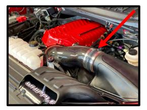
105. (Stock throttle body installations) Install the supplied 5" ID x 2 1/4" silicone hose over air inlet tube and airbox lid. Install the supplied reducer silicone hose over air inlet tube and stock throttle body. Connect the other end to the stock throttle body. Secure all ends with the supplied hose clamps (2) #80, (1) #64 and (1) #56 on throttle body.
