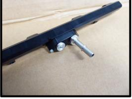
47. Install the supplied (2) #2-906 orings to the (2) inlet/outlet fittings. Install these (2) fittings into rear side of fuel rails. Apply light amount of grease to oring for ease of installation. Using a ¾" wrench (or ¾" deep socket) on both the front and rear fittings, tighten both.
