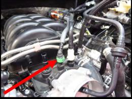
18. Remove the second brake booster quick connect line from intake manifold by squeezing locking tab and pulling away.
