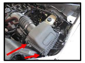
15. Using a 13mm socket, remove the (1) factory fastener securing airbox to the fender.
