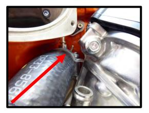
37. Remove stock oring from factory bank 2 heater tube, install on supplied heater tube. Install the supplied plastic heater tube into bank 2 heater port. Secure with supplied stepped bracket and factory bolt.
