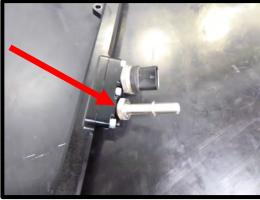
46. Install the supplied (1) #2-906 Viton oring to the (1 of 2) 45mm long 9.49mm outlet fitting. Apply light amount of grease to oring for ease of installation. Install fitting to the fuel inlet block. Install the supplied -6 ORB plug to the extra port.
