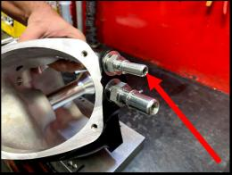
70. Install the supplied 1/2" ID x 14" with 90deg quick connect fitting brake aspirator hose (#HSF150-HS012) from the brake booster to the **lower** quick connect fitting on the supercharger inlet. Push until it clicks into place. **TIP:** For best routing, nestle in between cam cover and fuel rail, under the wiring and heater hose.
