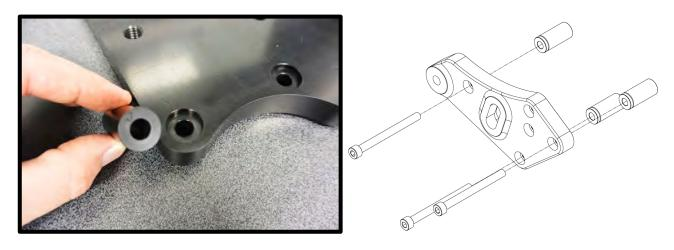
42. Use the supplied (3) 8mm x 90mm SHCS to secure the idler plate to the engine. Using a 6mm allen, torque to 22 lbs-ft
