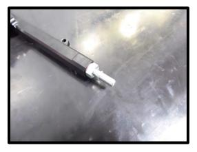
48. Install the supplied (1 per injector port) .515" injector shims to be installed to the injector port of the SC housing, to hold the injector up to its proper position. Install the fuel injectors to the fuel rail, apply generous amount of grease to oring for easy installation.
