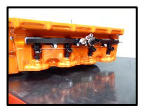
51. Install the supplied 3/8" fuel cross over line around the back of the supercharger by pressing until they click and lock in place.
