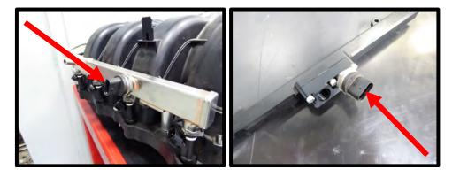
45. Install the supplied (1) #2-906 Viton oring to the (1 of 2) 45mm long 9.49mm inlet fitting. Apply light amount of grease to oring for ease of installation. Install fitting to the fuel inlet block.
