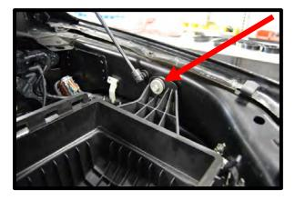
16. Remove first brake booster quick connect line from intake manifold by squeezing locking tab and pulling away.
