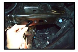
90. Install the IC reservoir to the (2) nut plates using the (4) 8mm x 25mm flanged hex headed bolt. Start (1) on each side to align holes to bushing. If off, you can use screwdriver to align the nut plate and bushing before installing the final (2) bolts. Torque to 15 lb-ft using a 13mm socket.
