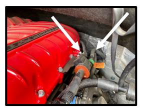
69. Install the supplied 3/8" ID x 12" with 55deg quick connect fitting hose (#18F150-HS011) to the EECPV barb fitting and **upper** quick connect fitting on SC inlet. Push until it clicks and locks into place.
