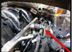
24. Using a 3/8" fuel line removal tool, remove the feed line from the factory port injection system to the direct injection mechanical pump. Slide removal tool between the lines, securing the DI side until it releases. NOTE: THIS FUEL LINE HAS A CHECK VALVE, DO NOT FLIP ORIENTATION. DO NOT REMOVE FROM DI PUMP TO ELIMINATE CONFUSION. 90-DEG END ALWAYS CONNECTS TO FUEL FEED SUPPLY!
