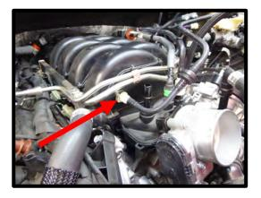
17. Disconnect the EVAP solenoid electrical connector by squeezing locking tab and pulling away. Disconnect the EVAP solenoid quick connect fitting hose from the EVAP solenoid and from the intake manifold by releasing locking tab and pulling away.
