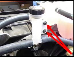
100. Install the ¾" ID rubber hose (#18F150-HS006) from the Bank 2 (OUTLET) IC fitting to the IC filler neck. Secure both ends with supplied pinch clamps. NOTE: NEVER SWITCH THE INTERCOOLER ROUTING, BANK 2 IS ALWAYS THE OUTLET!
