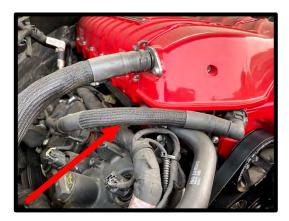
72. Plug the (8) fuel injector electrical connectors to the new fuel injectors until they click and lock in place.
