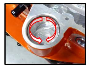
65. Apply generous amount of grease to the (1) #2-230 Viton bypass oring. Install the supercharger lid to the supercharger housing by carefully placing the bypass down. Secure the SC lid using the (17) 6mm x 30mm HHFCS and (3) 6mm x 70mm HHFCS (*marked green*) using the following pattern. Slide the EECPV bracket under bolts 3 and 5 from image (bank 2). Torque to 90 lbs-in using an 8mm socket.
