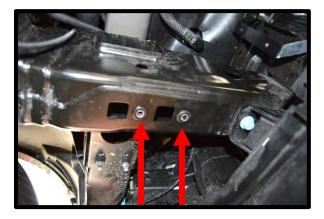
89. Install the supplied steel nut plates (2), (1) per side up through square opening with nuts facing up.
