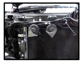
88. Install the supplied (4) rubber grommets and steel bushing into the (4) holes located on the driver and passenger side frame.
