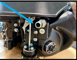
54. Using the supplied 5/16" OD silicone tube, install the (1) 80 1/2" cord. Start as shown with green arrow, go in a clockwise motion, to the front, then around the perimeter. End at yellow arrow position. Bunch it up so it has no gap at the end as any gap will be an air leak of un-intercooled air. Install the (1) 6.5" cord in the front section shown with the blue arrow.
