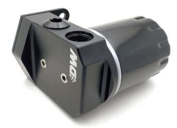
DW Spin On filters are compatible with pump gas, race gas, and ethanol. DW recommends a maximum service interval of 12 months or 12,000 miles. Shorter service intervals are recommended with harsher conditions and corrosive fuels. The DW SOF features dual -10AN O-Ring ports for plumbing flexability.
