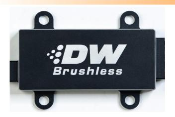
The DW C1 Brushless Pump Controller is included with the DW440 LPH in-tank fuel pump kits. This controller accepts an 8-22v DC input and creates a digital signal to allow effecient and precise speed and torque control of the DW440 pump. The controller is available in 2 configurations: C102 (dual speed), and C103 (pwm controlled).
