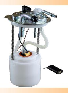
The DW400 05-19 GM SUV Module is a complete plug-n-play replacement for the OE unit. The module incorporates the DW400 pump which is over 60% more than the OE module. This module also integrates seamlessly with the OE wiring harness and level sender. The module includes a return plumbing kit with 8AN feed and 6AN return lines, a DWR1000 regulator, and a fuel pressure gauge. The module also utilizes a venturi fed surge bucket for consistent fueling at low tank levels and high G conditions.
