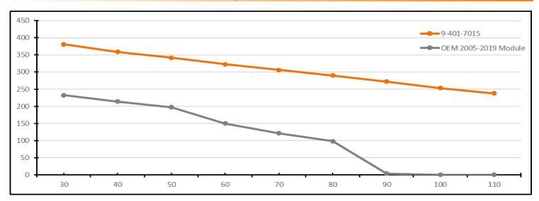
Note: On some Installations, the clocking tab will need to be removed to install module in tank Module Testing Notes: All testing performed by DeatschWerks at 13.5v on calibrated equipment. In-module flow rates are lower than pump alone due to parasitic losses of venturi system, check valves and plumbing.
