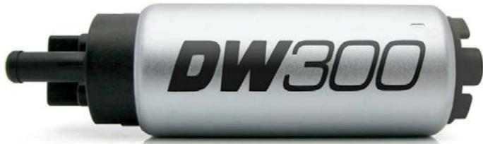
The DW300 is our flagship standard fitment in-tank pump. The DW300 flows 340lph at 40psi and is a popular choice for e85 applications or wherever the highest flowing standard fitment in-tank pump is needed. Quiet operation and pulse width modulation compatibility are delivered via the turbine impeller and computer balanced armature. E85 compatibility is built in via the carbon commutators and a fully encapsulated armature. All DW fuel pumps are backed by a 3-yr no fault warranty.
