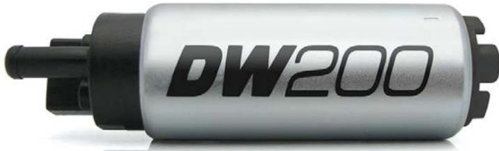
The DW200 flows 255lph at 40psi and is a popular choice for many high performance applications which can be fitted with a standard fitment pump. The DW200 features a quiet and reliable turbine impeller which is compatible with pulse width modulated pump drivers. The pump also features an encapsulated armature for compatability with ethanol based fuels. All DW fuel pumps are backed by a 3-yr no fault warranty.
