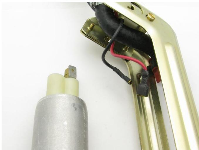
4 – remove the hose and remove the front lip from the base of the assembly
