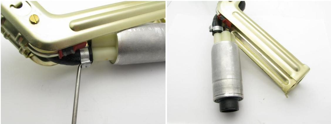
3 – disconnect the electrical connectors and remove the pump from the assembly
