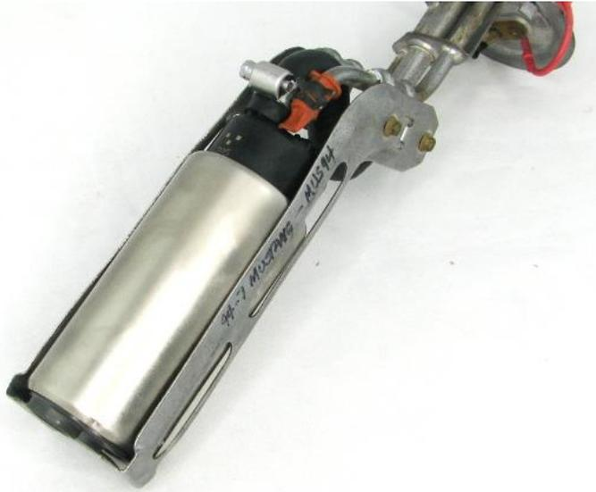
7 – install the fuel sock and wire in the electrical connector (blue is positive, the extra negative lead can be clipped or mounted to the assembly as an additional ground)
