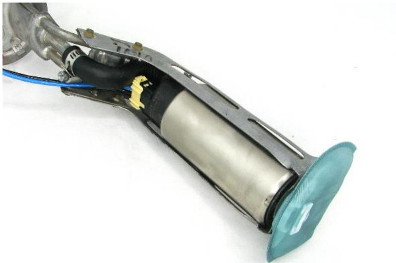
8 – reinstall the assembly into the fuel tank and attach a length of hose to the outlet of the pump assembly allowing it to drain into a fuel safe container and prime the fuel pump assembly
