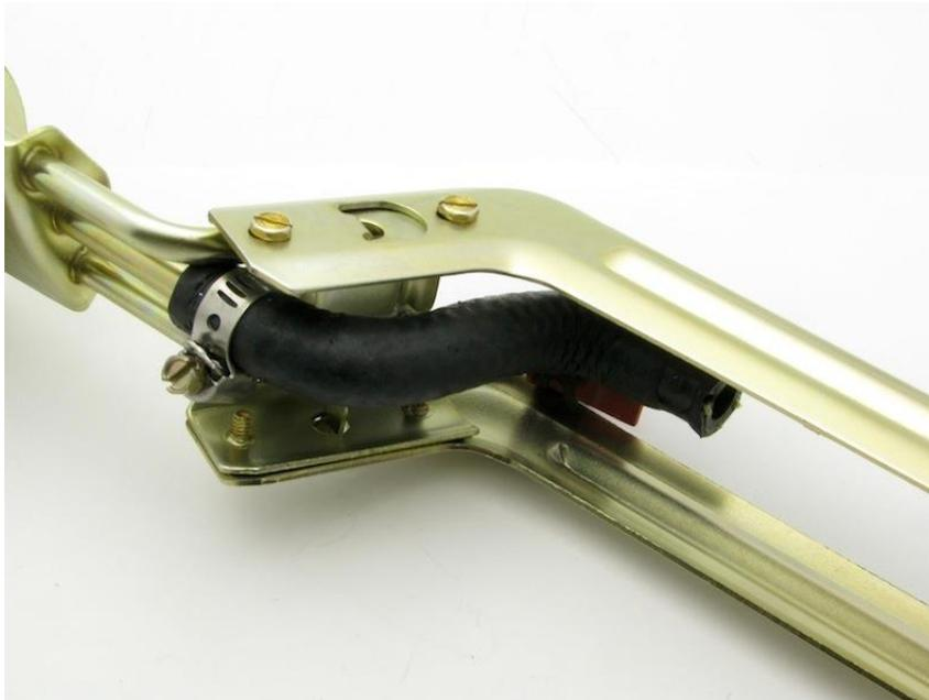
6 – insert DW400 into the hose and install the pump by pushing it into the assembly
