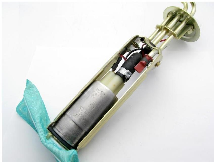
1 – remove the fuel sock from the base of the pump
