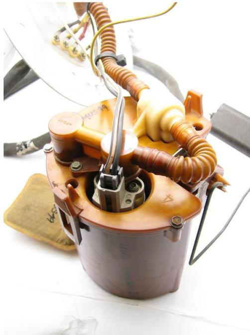
1 – remove the 3 screws holding the cap to the bucket and separate the bucket from the cap
