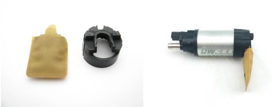
3 – remove the OE sock from the bucket and install the new sock supplied in the kit
