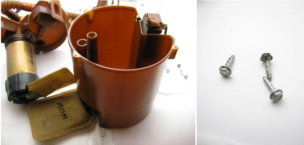
2 – remove the OE sock and isolator from the OE pump and install on the DW300m
