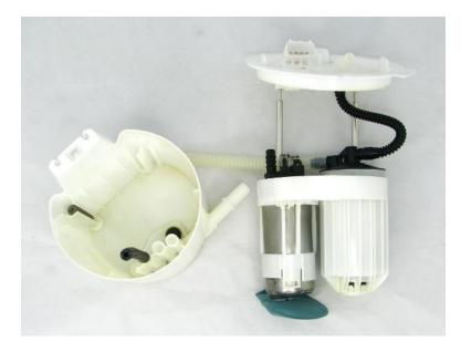
6 – install assembly center section into the assembly bucket and connect the 3/8" tube to the outlet of the pump, then tighten the hose clamps. Slide the larger permanent clamp (13/32") onto the hose and crimp it in place (over the barbs) with a pair of side-cutters. Slide the smaller permanent clamp (11/32") on the hose and install the free end on the smaller venturi outlet on the pump. Crimp the clamp in place under the barb
