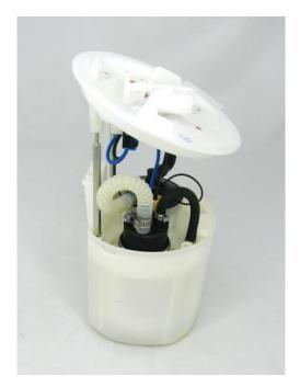
9 – reinstall the assembly into the fuel tank and attach a length of hose to the outlet of the pump assembly allowing it to drain into a fuel safe container and prime the fuel pump assembly
