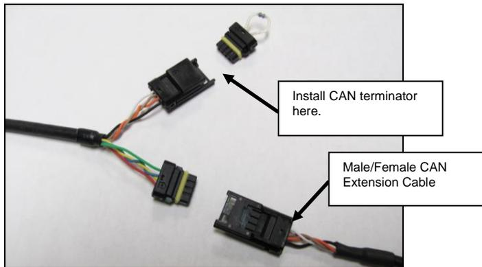
Holley EFI main harnesses use two types of CAN connectors. Earlier harnesses use a 2 pin metripak connector. The kit includes an adapter to go from this to the 4’ extension harness (note the white power and black ground wires are NOT needed for the Pro Dash, but need to be connected if other CAN devices require it for their power supply). Later harnesses plug directly into the 4’ extension harness.
