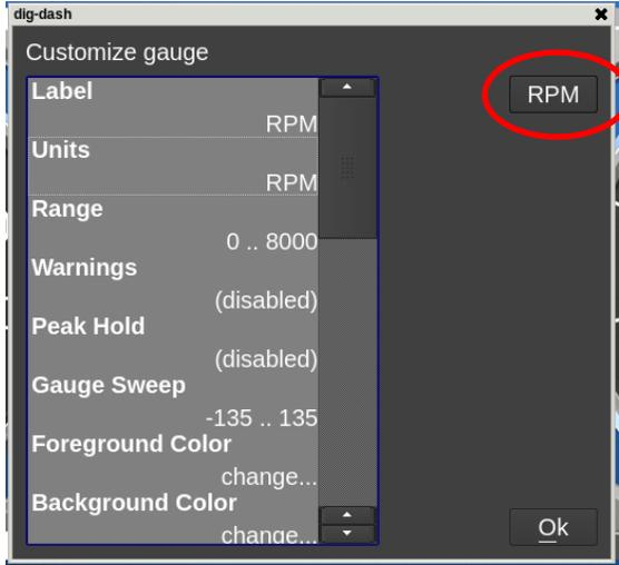
**NOTE:** Only the gauge value being displayed will be updated, the user **MUST** manually change Labels, Units, Range, Warnings etc. with proper values as these will **NOT** be updated automatically! Refer to the 'Customizing Your Layout' Section of the user manual for instructions on gauge customization.
