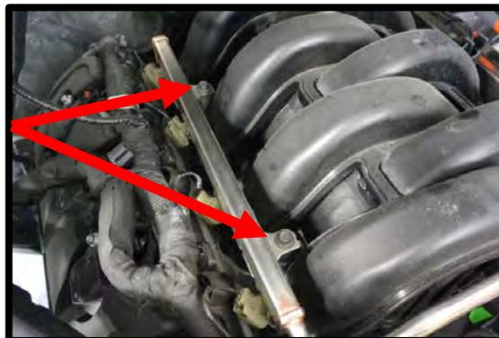
29. Loosen the (8) manifold to cylinder head bolts using an 8mm socket.
