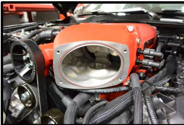
107. **(Stock throttle body)** Install throttle body adapter to supercharger inlet using the supplied (4) 6mm x 14mm FHCS (4mm allen socket). Torque to 88 lbs-in. Install stock TB oring to adapter. Install stock TB to throttle adapter using the supplied (4) 6mm x 50mm FHSCS. Torque to 88 lbs-in.
