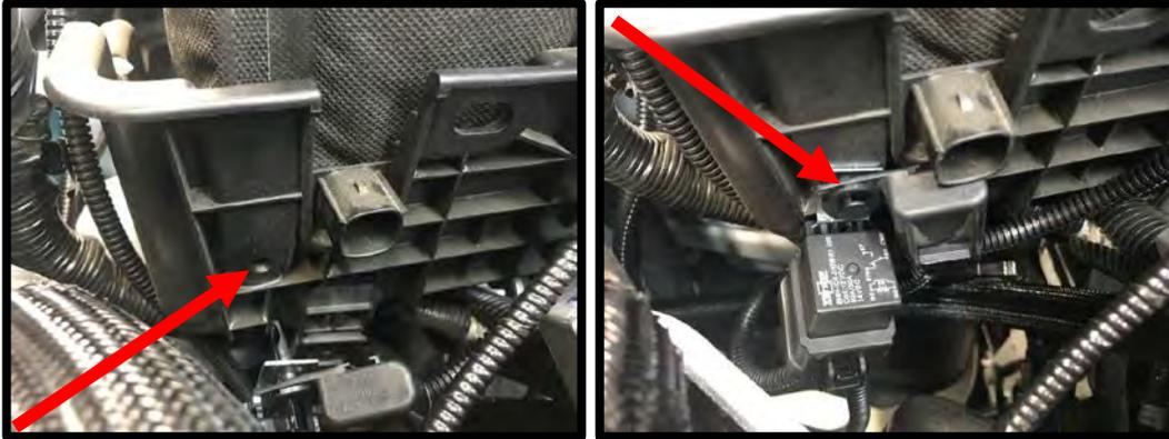
117. Using a 10mm socket, remove the nut on the power stud, located on the positive battery connector. Install the IC pump relay power eyelet (red wire) to the power stud on the battery positive (+) stud. Use a 10mm socket to secure stock and IC power wire.
