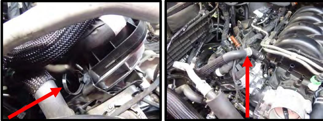
22. Install the supplied driver side heater tube to passenger side of block. Install the supplied oring to the tube and apply light amount of grease to oring surface. Install tube into block and secure with the factory bolt using an 8mm socket. Torque to 89 lbs-in.
