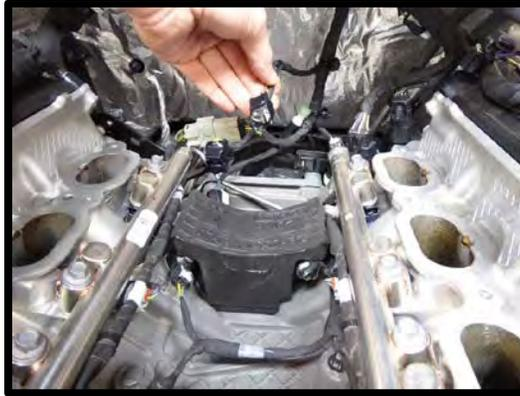
64. Install the (1) supplied manifold top oring (.103" x 51.25") into the oring groove. Use silicone/grease in receiver groove to help oring stay in place.
