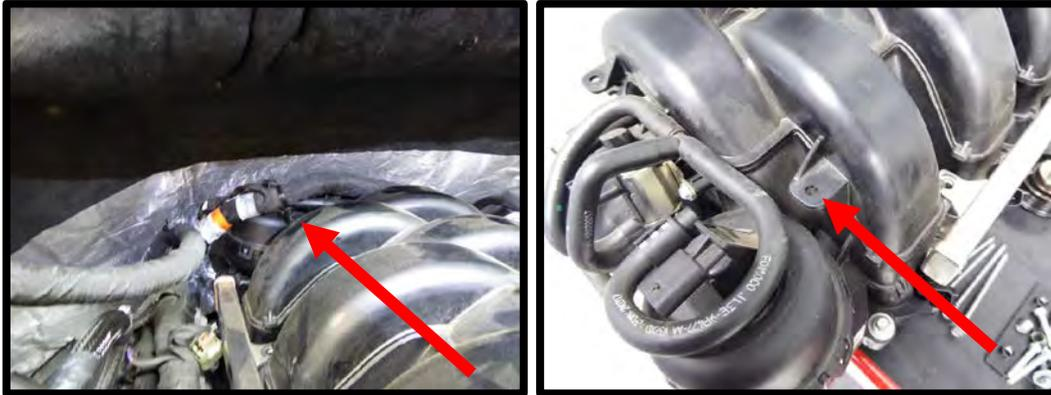
31. Remove the intake manifold from the engine. To do so, remove the (3) wire harness push pin supports from the back of the intake manifold, disconnect the (3) IMRC connectors by pushing on the locking tab and pulling, disconnect the 4-way MAP sensor connector and disconnect the 12-way DI injector harness by releasing the locking tab and pulling apart.
