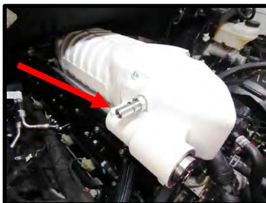
71. Install the supplied #117 Nitrile orings (2) to the aluminum intercooler fitting. Apply light amount of grease to each surface. Install fitting into lower intercooler passage by carefully sliding in, be cautious of the oring and ensure there is no debris during installation.
