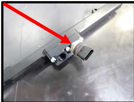
44. Install the supplied (1) -6 oring to the (1 of 2) 45mm long 9.49mm inlet fitting. Apply light amount of grease to oring for ease of installation. Install fitting to the fuel inlet block.
