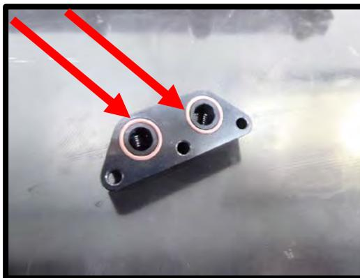
43. Using a 27mm socket, remove the fuel PSI sensor from the factory fuel rail. Install the factory fuel PSI sensor to the adapter using a 27mm socket. Torque to 53 lbs-in, then an additional 25 degree rotation. \*No sealant on the threads.
