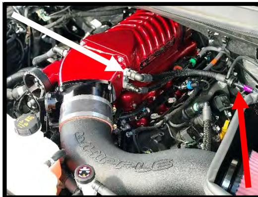
106. Install the supplied throttle body oring to the supercharger inlet. Apply light amount of grease to help hold in place.
