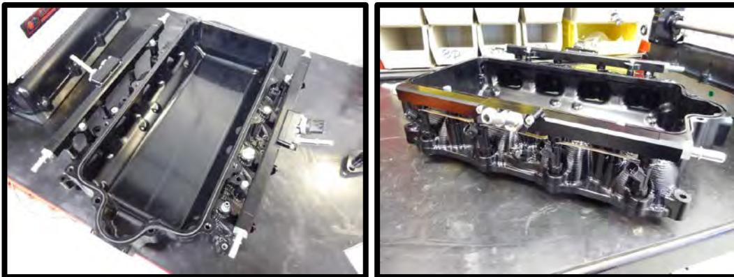
49. Install the rear pre-made cross-over fuel line. Press until the click and lock into position.
