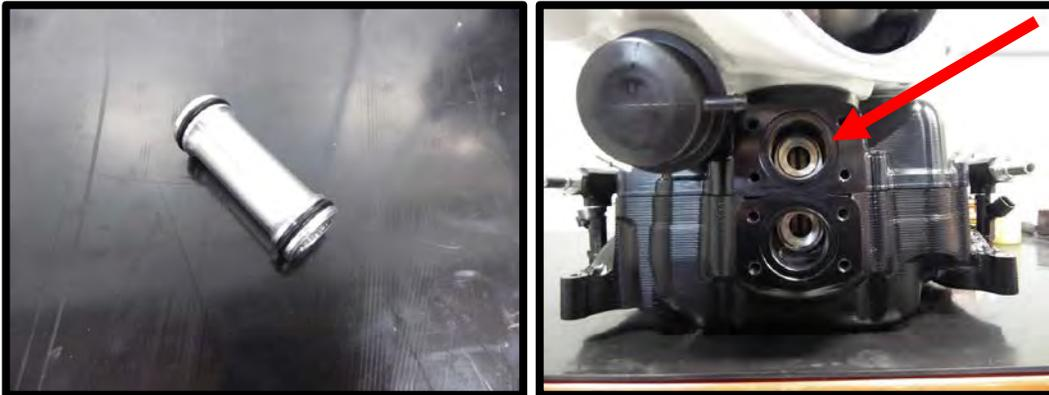
67. Install the supplied #126 Viton oring to the manifold top intercooler passage location. Apply light amount of grease to oring to help secure in place. Install the supplied intercooler hose connect fitting to upper intercooler passage. Apply light amount of Blue Loctite #243 to threads of the supplied (2 of 4) 6mm x 10mm FHSCS.
