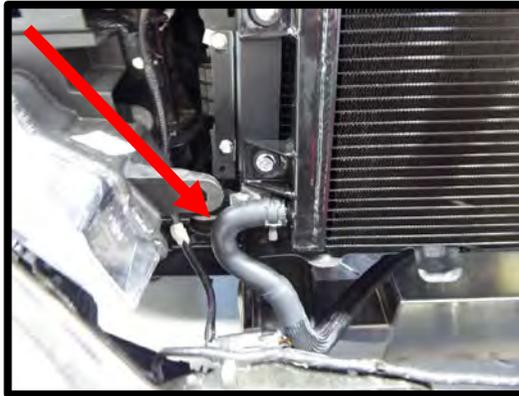
99. Connect the  $\frac{3}{4}$ " ID molded/formed (33") hose (#18F150-HS009A) from the LTR driver side bottom fitting that you previously installed, to the IC pump outlet barb. Secure with supplied pinch clamp. **NOTE: Ensure that this hose cannot kink or rub anything overtime.**
