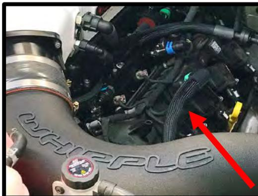
116. Locate the stock hole in the battery box. Use the supplied plastic push pin to secure the intercooler relay and fuse holder to the battery box. Route the power wire to the main power stud at the battery side. Route the ground wire around the front of the battery box, then back towards the fuse box. Zip-tie each wire for a clean installation.
