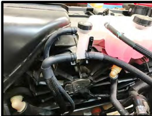
101. Connect the 3/4" ID hose (#18F150-HS007) and the 3/8" ID hose (#18F150-HS008) hose coming from the IC filler neck to the 3/4" and 3/8" barb fitting on the IC reservoir. Secure with supplied pinch clamp. **NOTE: Ensure that this hose cannot kink or rub anything overtime.**
