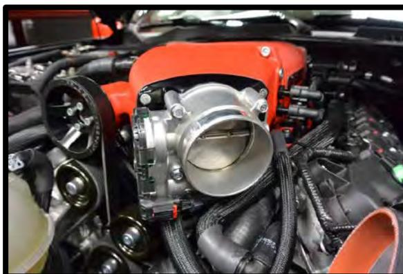
108. **(Whipple 132mm Crusher throttle body)** Install throttle body to supercharger inlet using the supplied (3) 6mm x 25mm SHCS and (1) 6mm x 50mm SHCS using a 5mm allen socket. Torque to 88 lbs-in.
