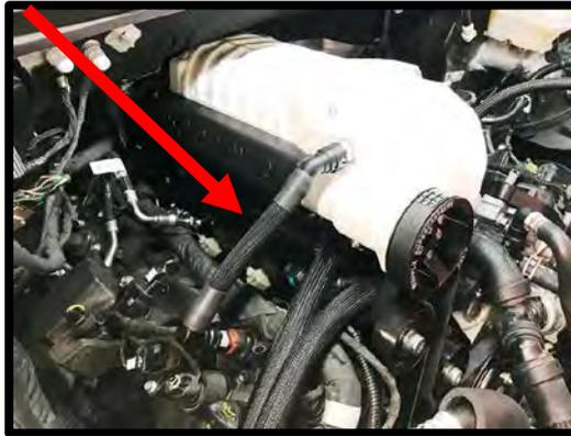
76. Install the supplied 3/8" x 8 1/2" EVAP hose (#18F150-HS002) to the EVAP solenoid and bottom inlet fitting.
