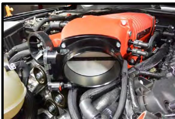
109. Connect the electronic throttle extension to the electric motor. Press until it clicks and locks into place. Press the safety lock until it clicks and locks into place. Secure harness to the intercooler line with a zip-tie to ensure proper clearance from the belt system.
