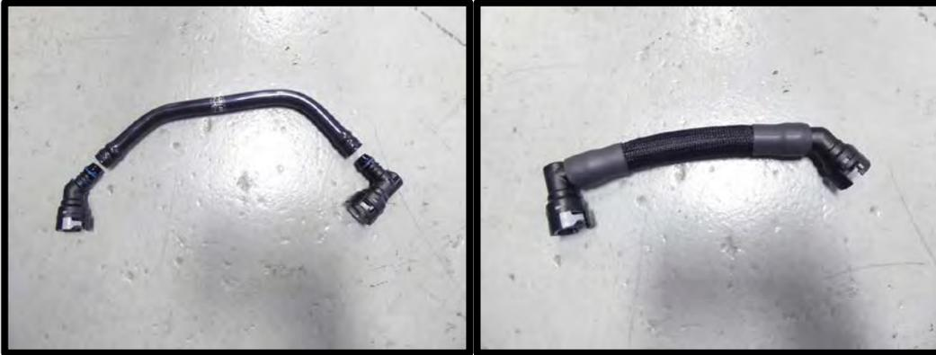
75. Install the new PCV hose to the PCV fitting (passenger side valve cover) to the SC inlet (passenger side).
