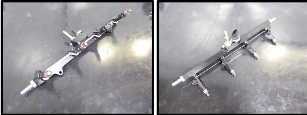
48. Mount fuel rails to intake manifold using the (4) 32mm long spacers between the manifold and fuel rail boss and the (4) 6mm x 50mm SHCS, apply light amount of blue Loctite #243 to threads. Torque to 90 in-lbs using a 5mm allen socket.
