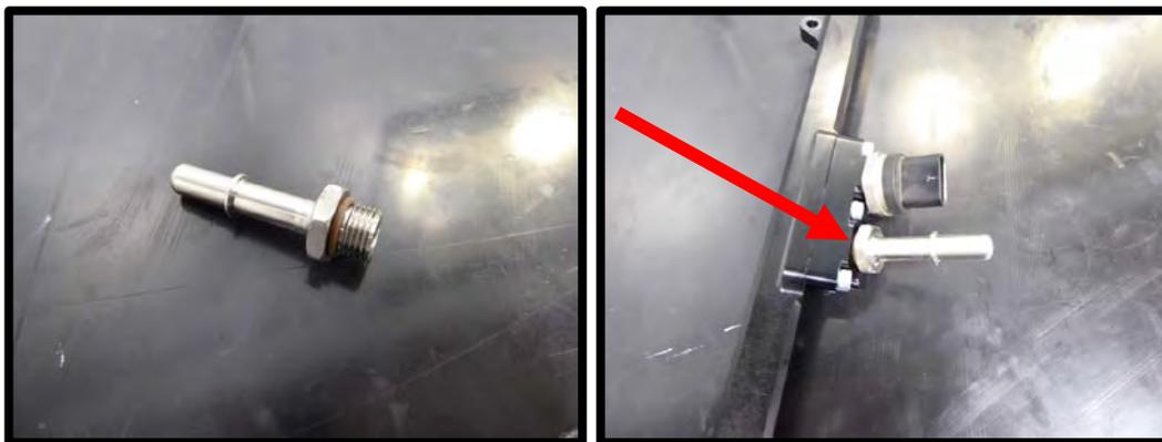
45. Install the supplied (1) -6 oring to the (1 of 2) 45mm long 9.49mm outlet fitting. Apply light amount of grease to oring for ease of installation. Install fitting to the fuel inlet block. Install the supplied -6 ORB plug to the extra port.
