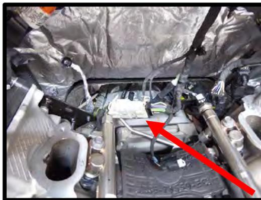
33. Clean the intake manifold to cylinder head surface using carb cleaner or acetone. Install tape over the exposed ports until manifold installation.
