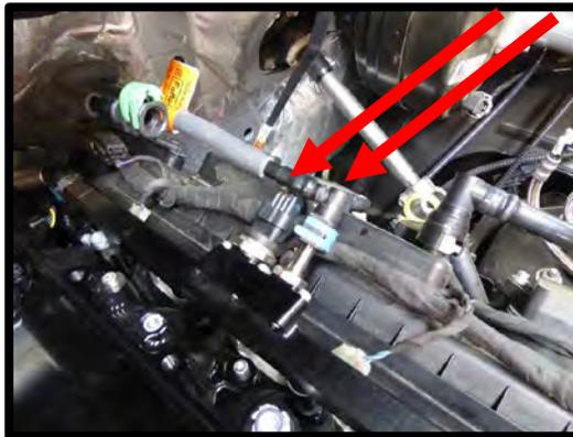
59. Plug the (8) fuel injector electrical connectors to the new fuel injectors until they click and lock in place.
