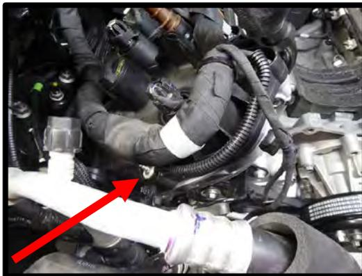
40. **(Complete kits) Gap the supplied spark plugs to .028" (out of box is .050")**. Install the gapped NGK LTR7IX spark plugs. Apply light amount of anti-seize to threads. Torque spark plugs to 124 lbs-in. Reinstall the coils on plugs and torque bolts to 53 lbs-in.
