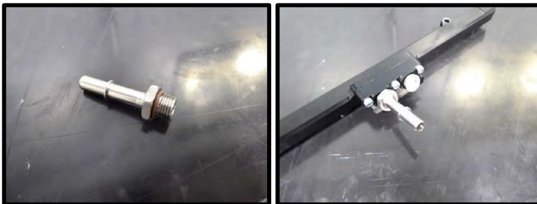
46. Install the supplied -6 orings to the (4) inlet/outlet fittings. Install these (4) fittings into each side of the fuel rails. Apply light amount of grease to oring for ease of installation. Using a 3/4" wrench (or 3/4" deep socket) on both the front and rear fittings, tighten both.
