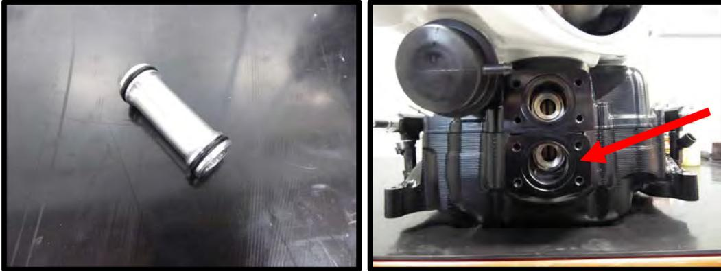
72. Install the supplied #126 oring to the manifold bottom intercooler passage location. Apply light amount of grease to oring to help secure in place. Install the supplied intercooler hose connect fitting to lower intercooler passage. Apply light amount of blue Loctite #243 to threads of the supplied (2 of 4) 6mm x 10mm FHSCS.
