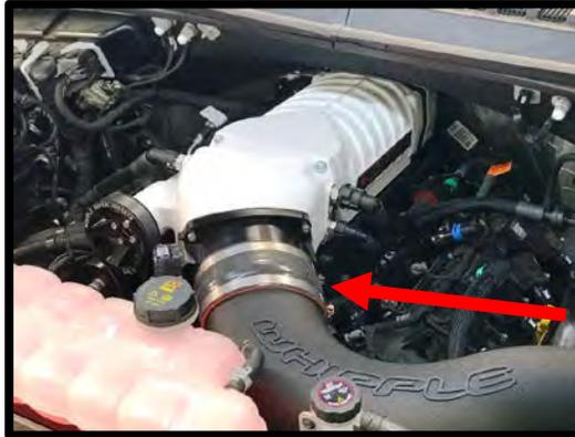
114. (**Stock throttle body installations**) Install the supplied reducer silicone hose over air inlet tube. Connect the other end to the stock throttle body. Secure all ends with the supplied hose clamps.
