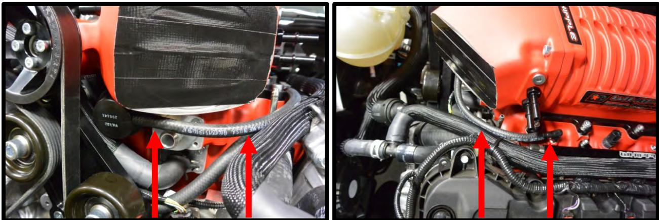
74. Using a razor blade, carefully cut the 90deg and 45 deg quick connect fittings from the factory PCV line. Install these fittings into the supplied 1/2" x 7" hose (#18F150-HS004). Install the 3/4" x 8" sleeving and heat shrink to the 1/2" x 7" hose. Shrink sleeving and heat shrink, using the heat shrink material to cover the cut ends of the hose.
