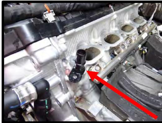
23. Disconnect the driver side heater tube quick connect fitting by squeezing and lifting away. Remove the heater tube overflow hose using a pinch clamp tool. Using an 8mm socket on the 1 factory bolt, remove the heater tube. Install the supplied oring to the shorter heater tube and install to factory location, secure with stock bolt, torque to 89 lbs-in. Reconnect both factory hoses.
