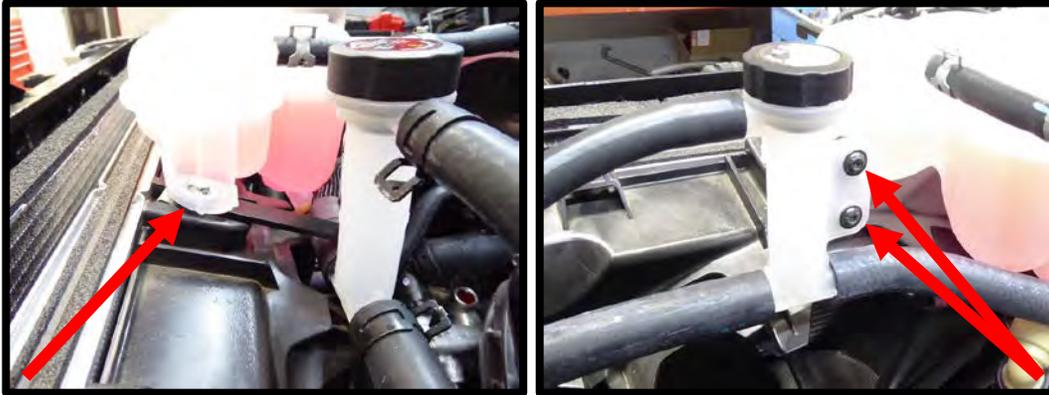
104. Install the 3/4" ID rubber hose (#18F150-HS006) from the top IC fitting (outlet) to the IC filler neck. Secure both ends with supplied pinch clamps.
