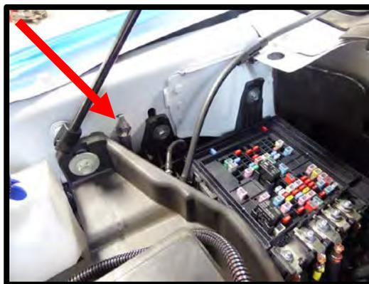
119. Pull the red 10amp fuse from position #F17 (ABS). Install the 10amp red fuse in the unused fuse slot on the fuse tap. Install the supplied fuse tap into position #F17 (ABS). **Note:** 10amp red fuse should be in bottom slot, 5amp should be in top slot. Make sure wire has enough room when fuse cover closes, route around fuses for clean installation.
