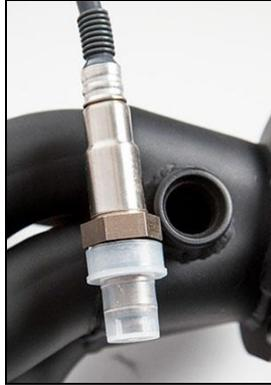
**Clamp-On Oxygen Sensor Bung**
