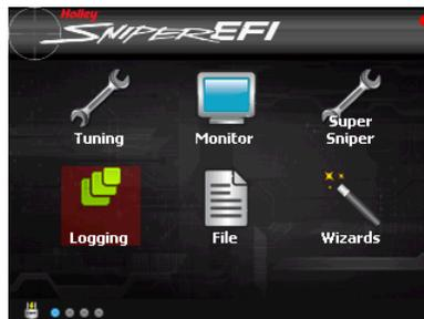
2. To turn on Data Logging press "Start Log" from the Logging Menu
