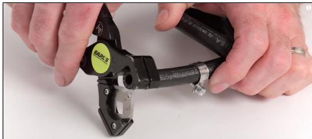
2. Install the fitting, by sliding the fitting into the hose. Make sure the hose seats flush with the fitting (see below).
