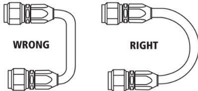
Keep the bend radius of the hose as large as possible to avoid collapsing of the hose and restriction of flow. Follow catalog specs on minimum bend radii.
