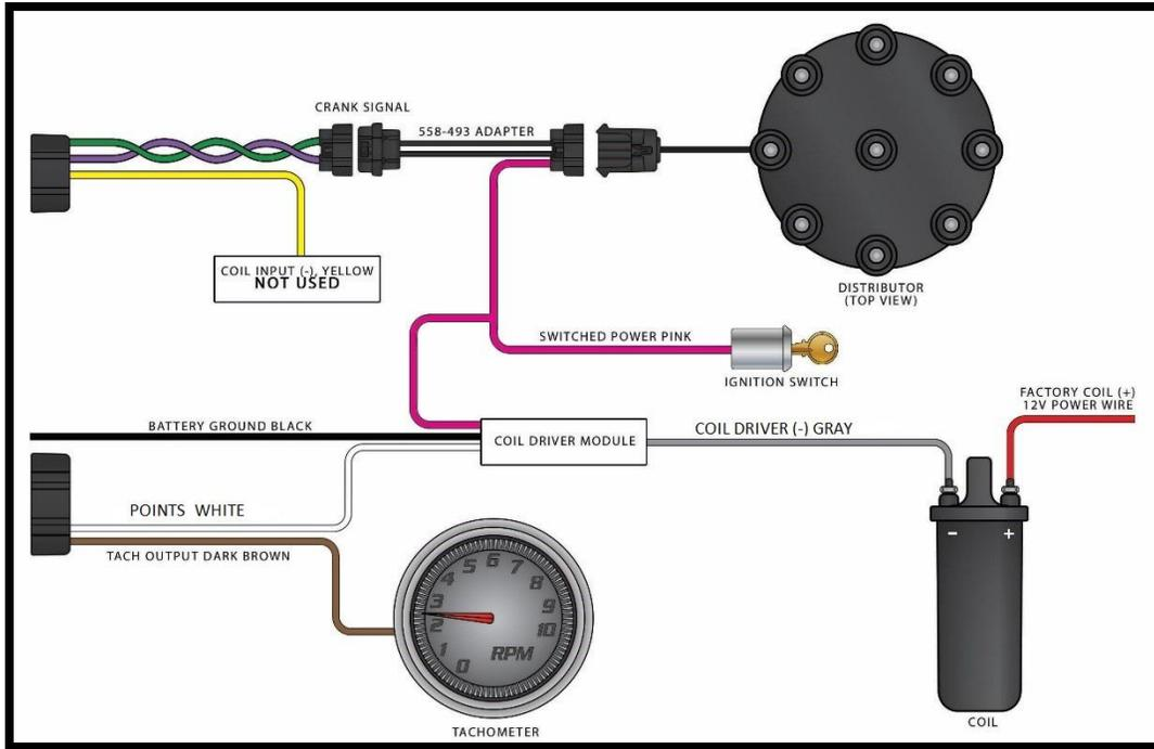
**WIRING W/ Holley Dual Sync Distributor and CAPACITIVE DISCHARGE BOX (Such as MSD 6AL)**
