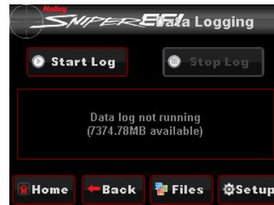
3. To turn off Data Logging press "Stop Log" from the Logging Menu or turn the ignition off.
