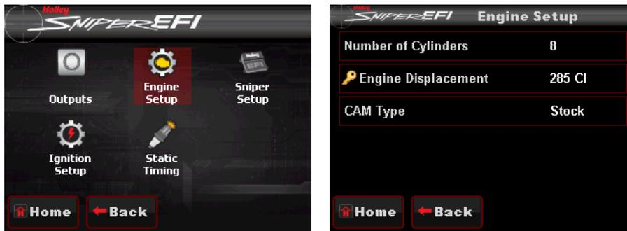
**Number of Cylinders:** Adjust the number of cylinders of the engine
