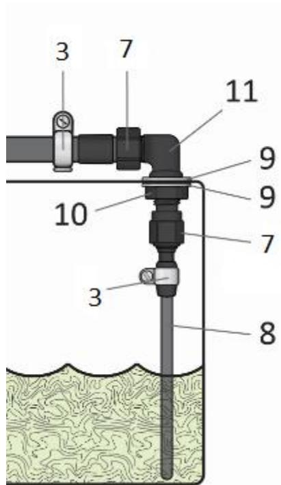
1. Drill a 9/16" hole and debur. Remove all metal shavings and particles from tank.
