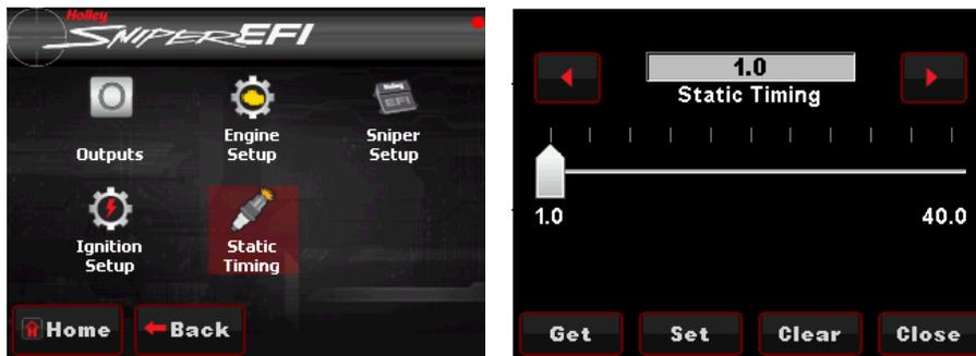
**Get Icon:** If static timing has been set and user has navigated to another screen in the handheld, press the "Get" icon to view what the static timing has been set to.
