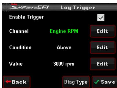
This example will start a log as soon as the engine RPM Exceeds 3000 RPM.
