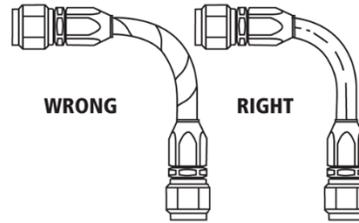
Do not twist during installation. This can be determined by the printed layline on the hose. Pressure applied to a twisted hose can cause hose failure or loosening of connections.
