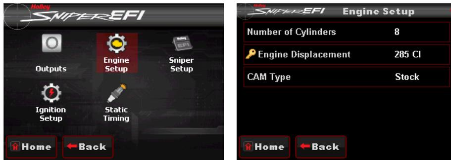
**Number of Cylinders:** Adjust the number of cylinders of the engine
