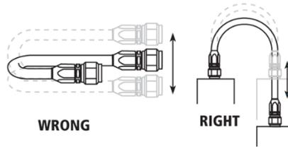
Make sure relative motion of the machine components produces bending rather than twisting of the hose. Hose should be routed so that the flex is in the same plane as the equipment movement.
