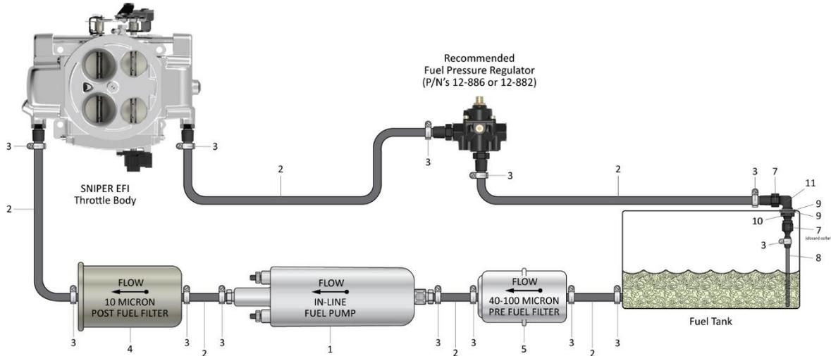
2. Mount the electric fuel pump as close to the fuel tank outlet as possible with the bracket provided. Mounting the fuel pump in this manner will insure that the pump will prime easily to ensure faster starts.
