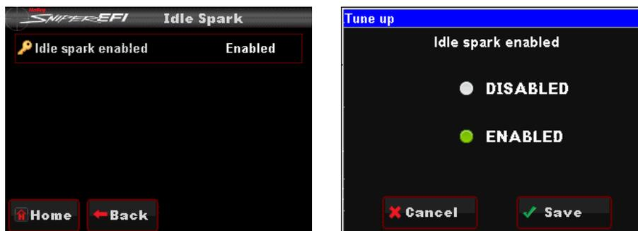
**NOTE:** This feature should be disabled when checking base timing with a timing light and not using the Static Timing option. If not disabled rev the engine to approximately 2000 RPM when syncing timing.
