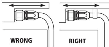
Install hose runs to avoid rubbing or abrasion. Use Earl's Hose Clamps to support long runs of hose or to keep away from moving parts. It is important that the clamps not allow the hose to move. This movement will cause abrasion and temperature hose failure.
