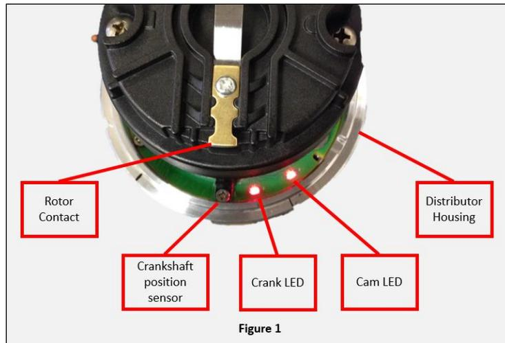
**NOTE:** All adjustments will be made by rotating the distributor housing only. **DO NOT ROTATE THE CRANKSHAFT** as it should remain at 50 degrees BTDC.
