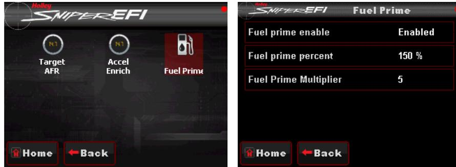
**NOTE:** This only injects fuel once at key-on, and will not do it again until the engine has run. This fuel prime occurs 2 ½ seconds after key-on. If you quickly turn the ignition key without waiting for 2 ½ seconds, the prime will not occur and it may take longer for the engine to start.
