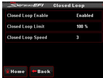
**Closed Loop Enable/Disable:** This menu enables or disables closed loop operation. There is typically no reason to turn off closed loop operation unless you suspect an oxygen sensor problem and want to disable the sensor. **Note:** Self-Tuning requires closed loop operation to function.
