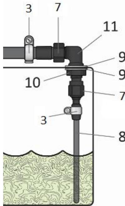
1. Drill a 9/16" hole and debur. Remove all metal shavings and particles from tank.
