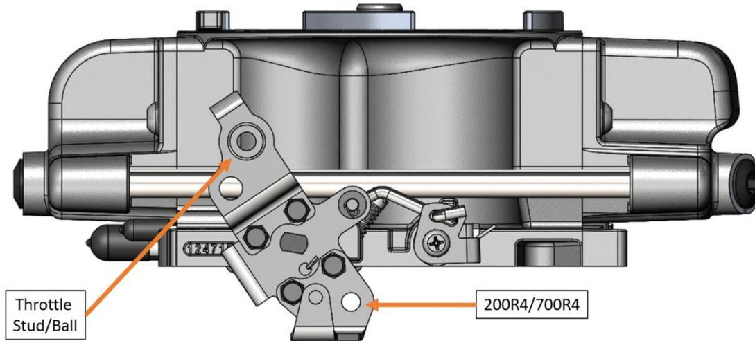
3. Reconnect the throttle and if applicable transmission kick-down linkage. Be sure to check for any binding conditions and correct before proceeding. Poorly routed throttle cables & linkages can cause throttle pedal issues.
