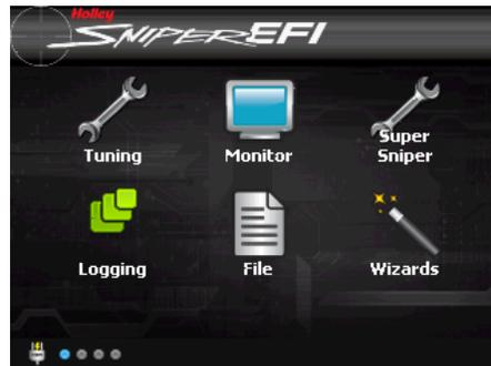
The Home screen contains icons which will navigate to different functional features of the 3.5” Touch Screen. These features will be discussed in detail throughout the main manual. The 3.5” Touch Screen will not display sensor parameters until a base calibration has been put in the unit using the Wizard.
