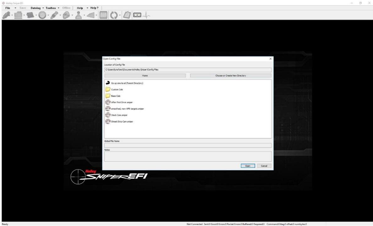
3. Calibration can be viewed and Modified using the Sniper Software. It can be saved directly to the SD card or to the Config Files folder. If saving to the Config Files Folder a copy of the tune will also need to be placed on the SD Card to Transfer it to the Sniper EFI via the Handheld.
