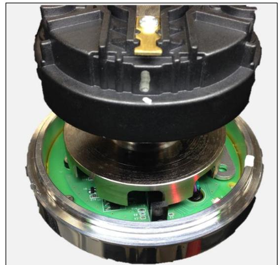
Turn the housing **clockwise** until the Crank LED comes back **ON** (**Figure 7**). Stop at this point. This will position the distributor close to where it needs to be. Install and snug the distributor clamp down at this point.
