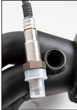
**Clamp-On Oxygen Sensor Bung**
