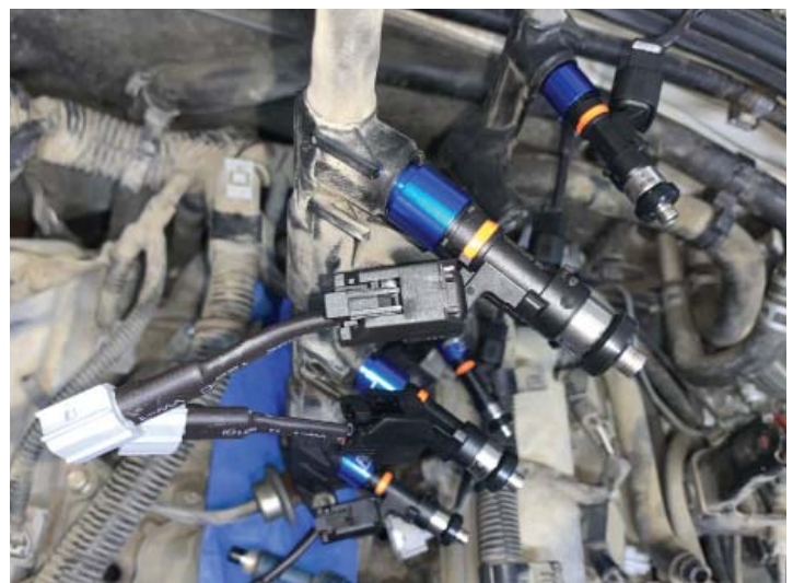
New Fuel Injector
