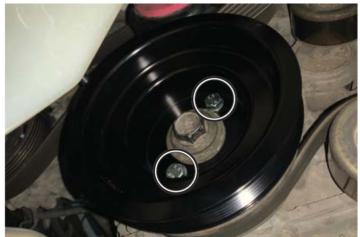
Crank Pulley Installed
