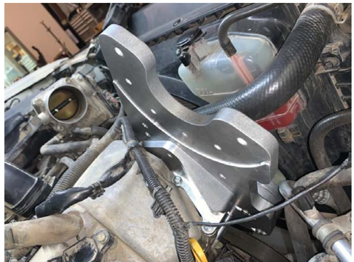
ProCharger Bracket Assembly
