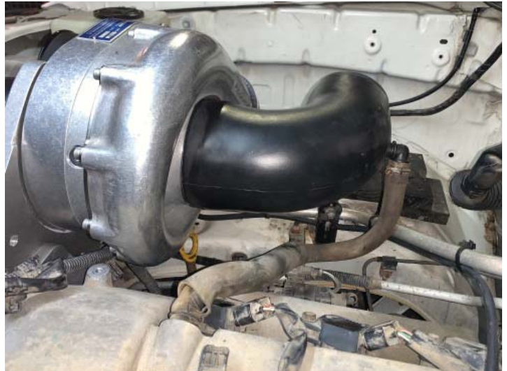
Connect PCV Line to Inlet
