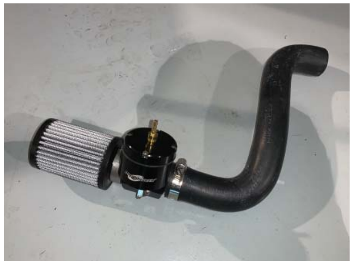
Surge Valve Assembled
