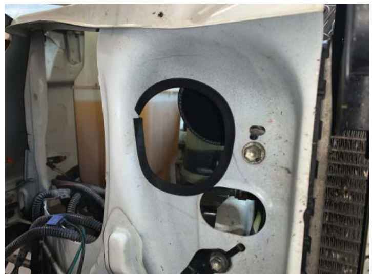
Rubber Trim Installed
