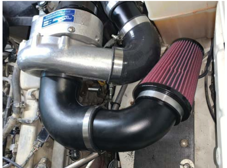
Air Filter Installed
