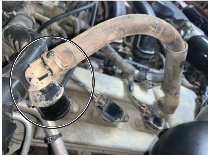
Remove PCV Line Fitting
