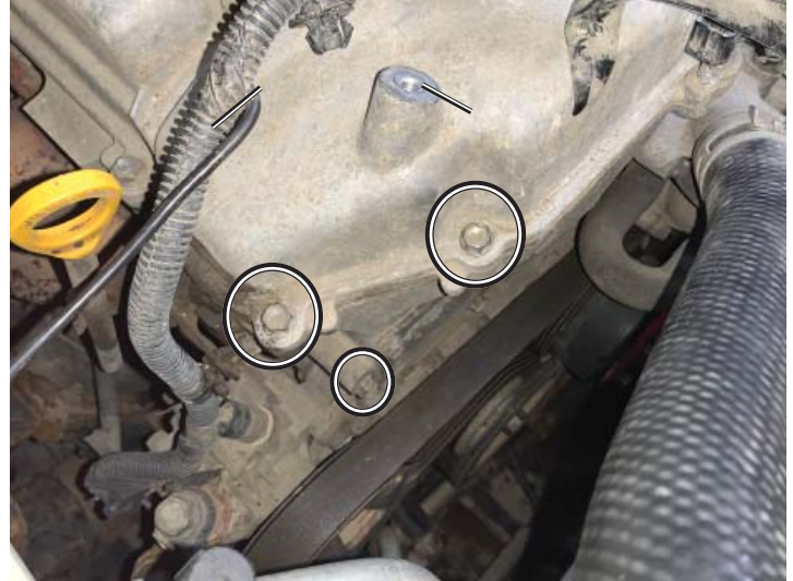
Bracket Mounting Holes
