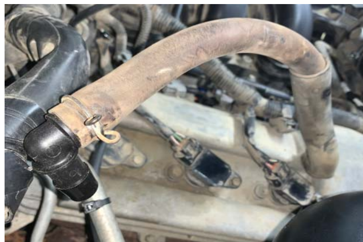
Install New PCV Line Fitting
