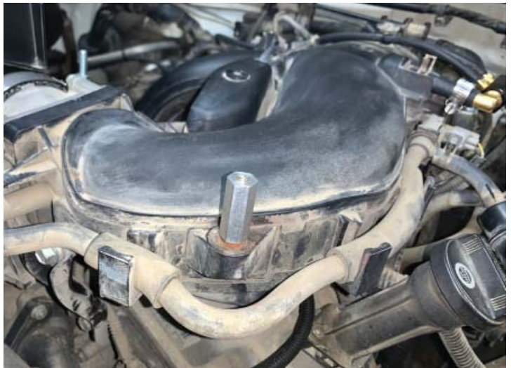
Engine Cover Spacer
