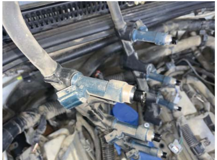
Factory Fuel Injector
