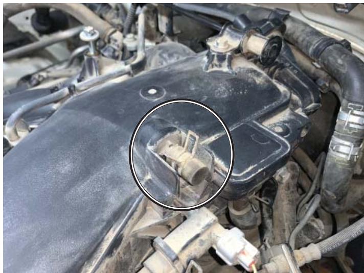
Remove Factory Vacuum Cap
