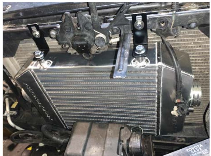
Upper Intercooler Brackets
