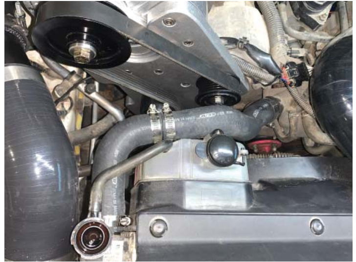
Upper Radiator Hose Installed
