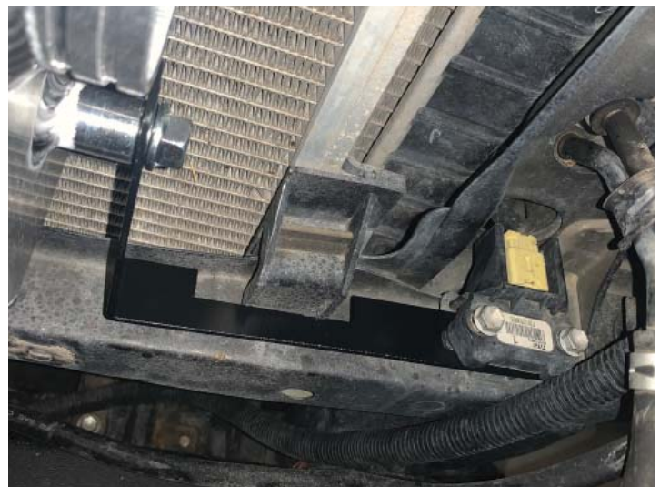
Driver's Lower Intercooler Bracket
