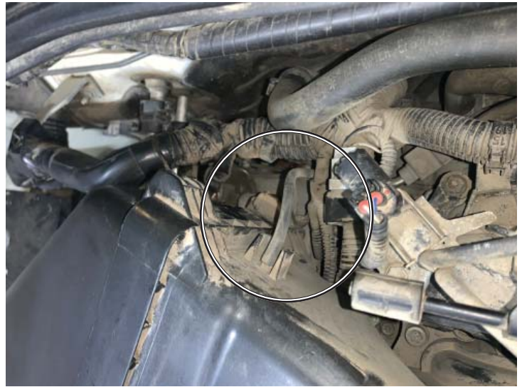
Fuel Pressure Regulator Vacuum Hose
