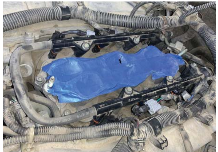
Fuel Injectors Installed
