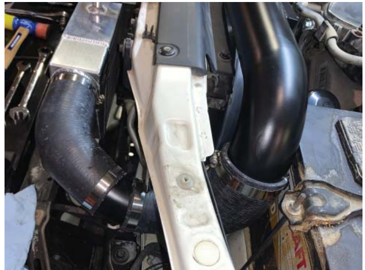
Rubber Reducer Installed
