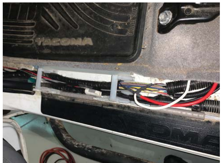
Factory Wire Loom
