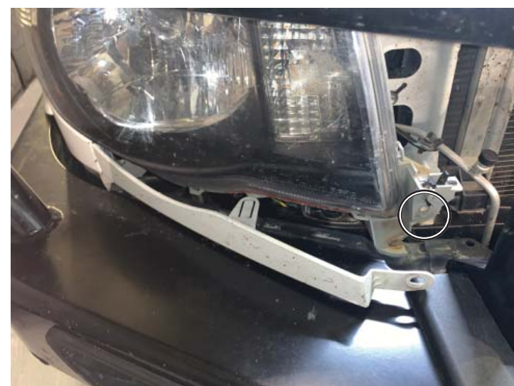
Lower Headlight Moulding
