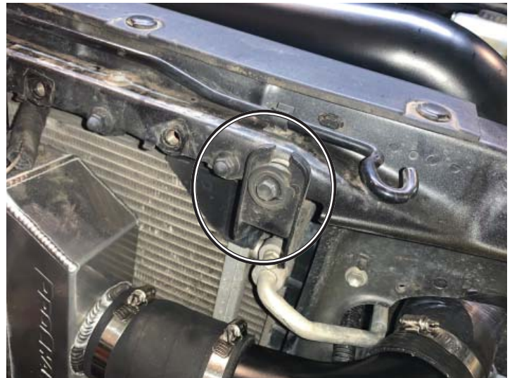
Radiator Bracket Bolt
