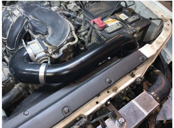
Throttle Body Connection
