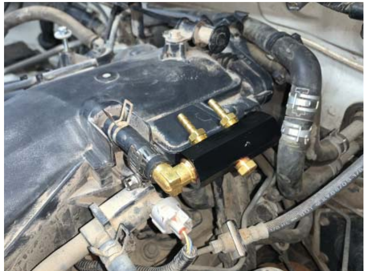
Vacuum Manifold Installed
