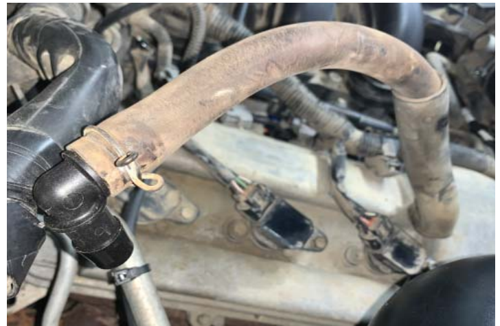
Install New PCV Line Fitting
