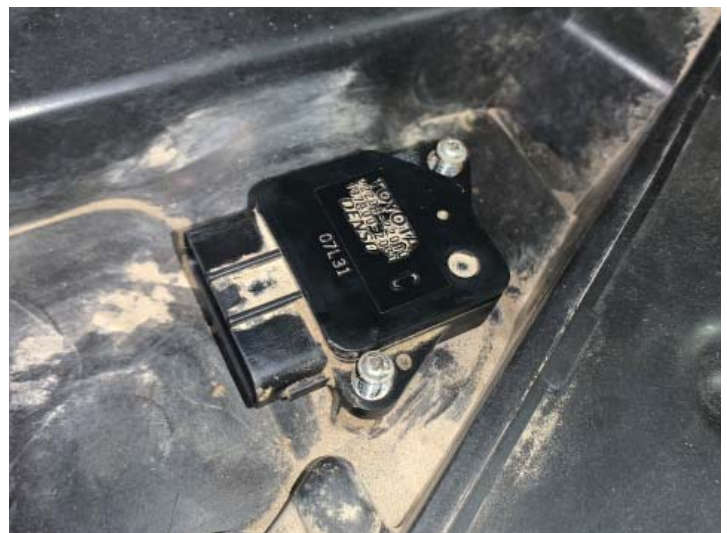
Remove MAF Sensor
