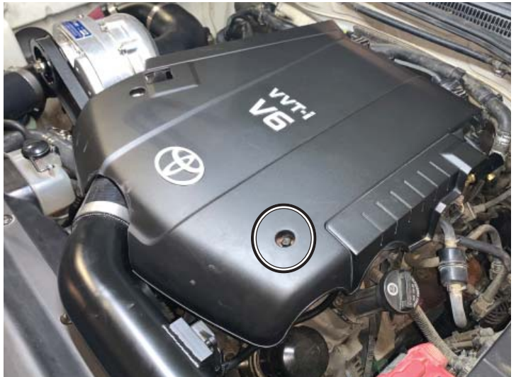
Engine Cover Installed
