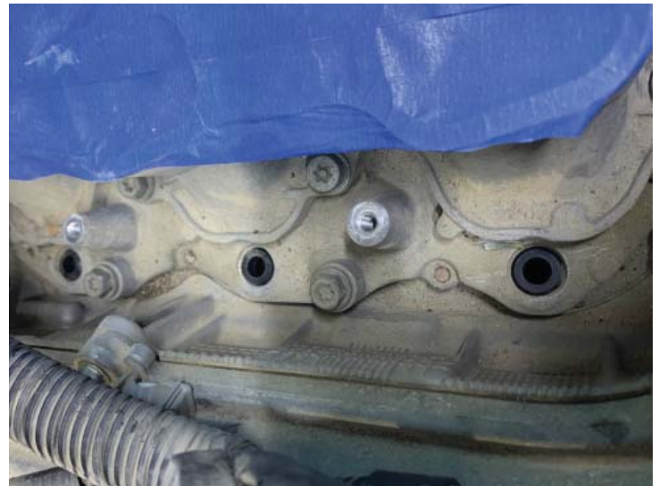
Injector Port Seal
