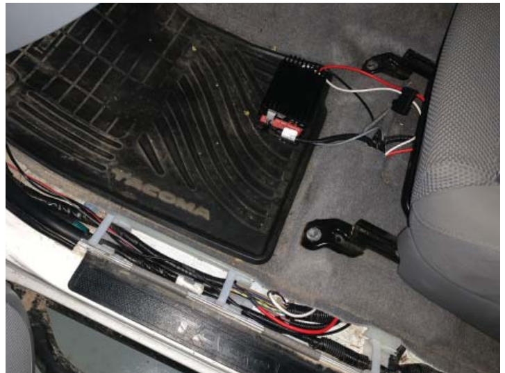
Run Wires Under Carpet
