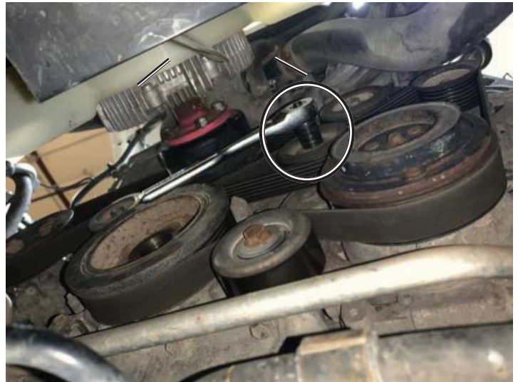
Loosen Factory Belt
