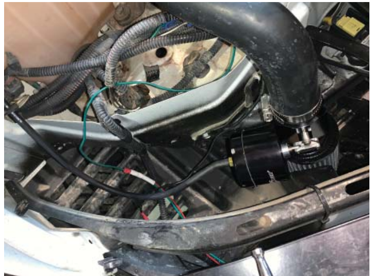
Surge Valve Installed
