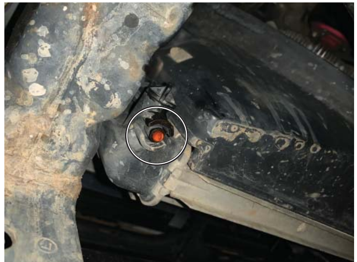
Radiator Drain Cock
