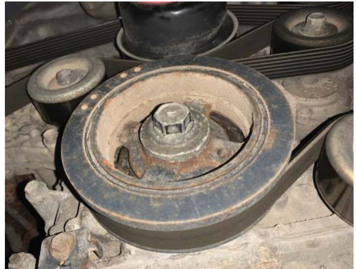
Factory Crank Bolt
