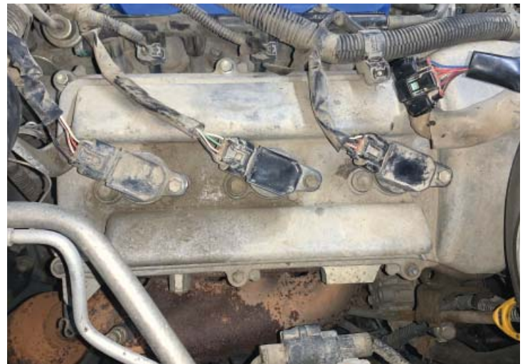
Spark Plug Coils
