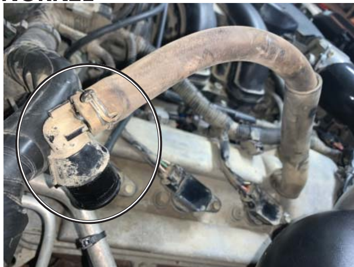
Remove PCV Line Fitting
