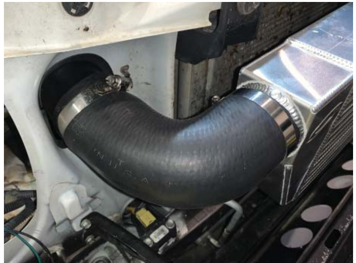
W/O Winch Intercooler Inlet
