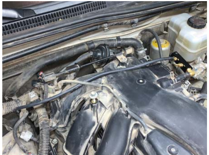
Pressure Regulator Vacuum Line
