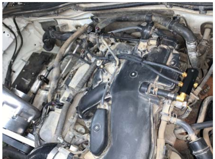
Surge Valve Vacuum Line
