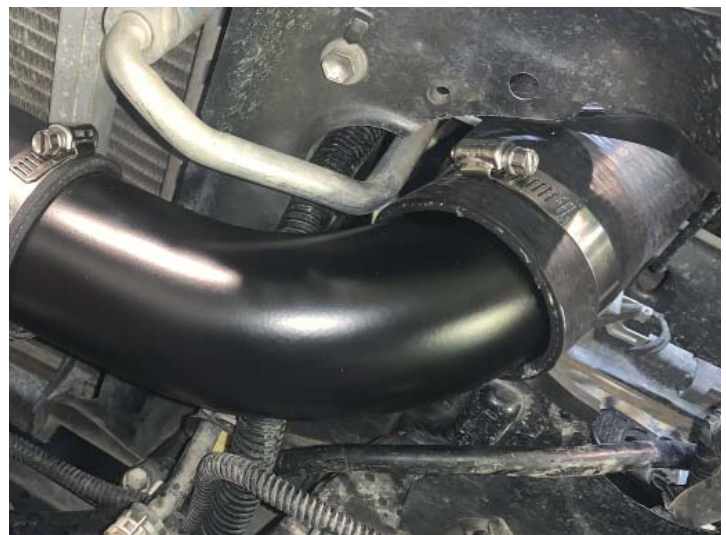
Rubber Reducer Installed
