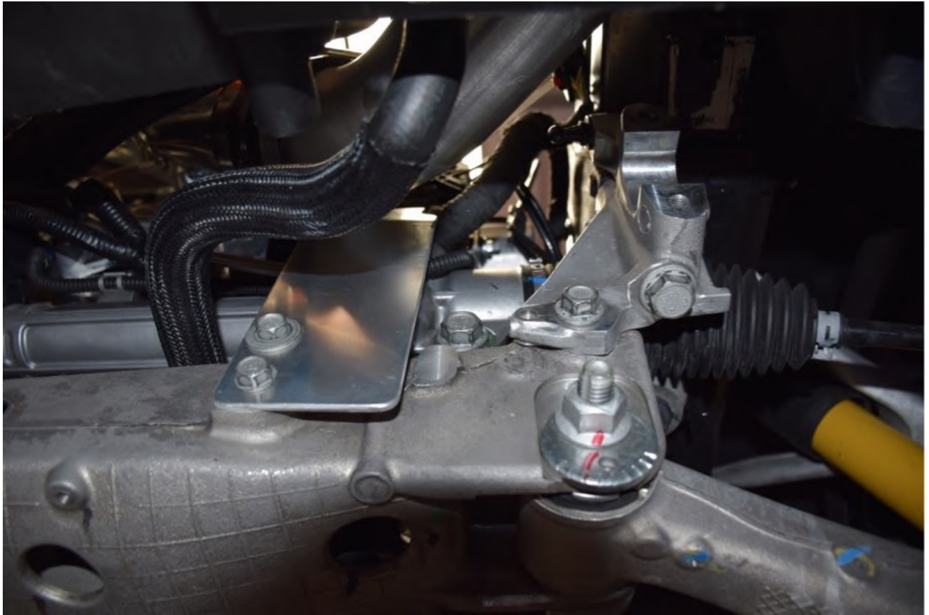
(TNEW ABS BRACKET ATTACHED TO SUBFRAME)
