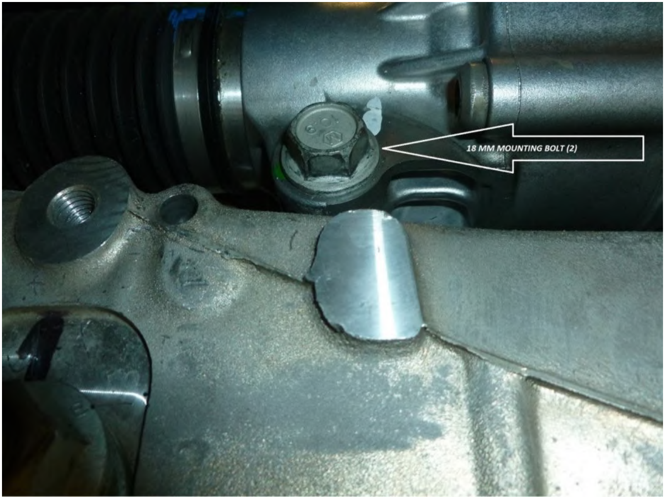
LEFT SIDE STEERING RACK MOUNTING BOLT
