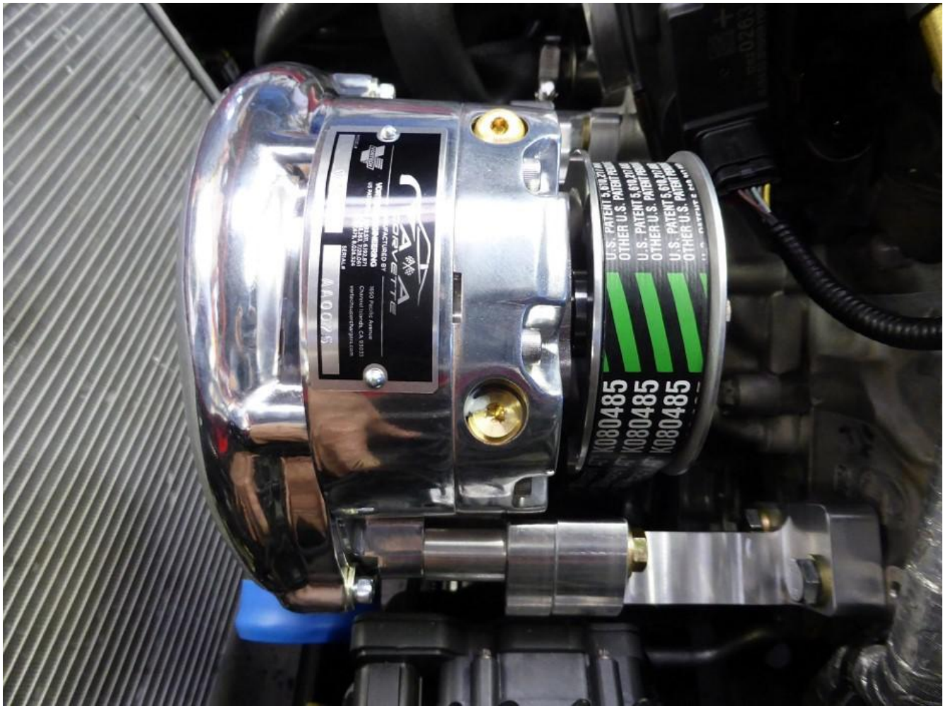
(SIDE VIEW OF SUPERCHARGER BRACKET INSTALLED)
