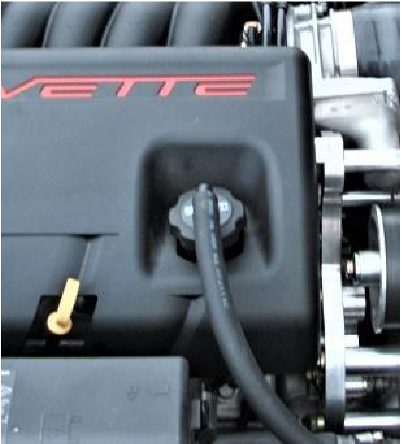
OIL CAP VENT HOSE INSTALLED ON STANDARD C6
