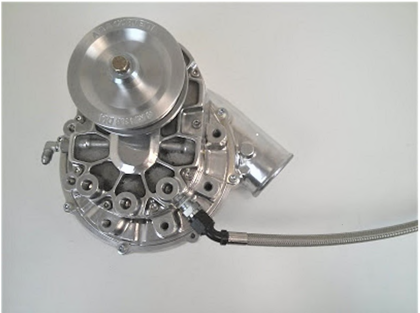
STAINLESS A-N OIL DRAIN LINE INSTALLED (NOT USED ON SELF-CONTAINED V3)
