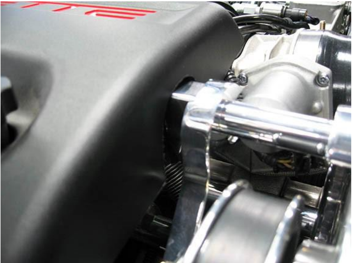
(TRIMMED PASSENGER SIDE COIL COVER INSTALLED)
