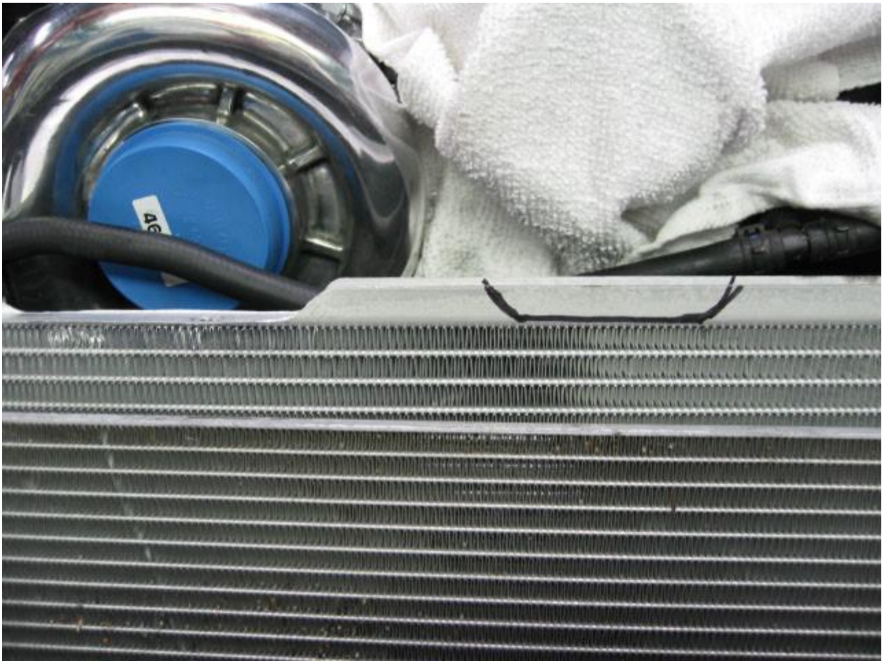
(RADIATOR MARKED FOR TRIMMING)
