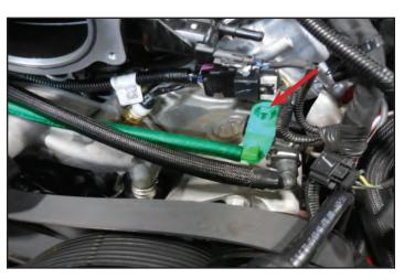
128. Install the provided cable tie with the "tree" mount on it (shown with the yellow arrow) to the electrical connection from the last step and install the "tree" into the threaded hole shown with the red arrow. Also at this time reconnect the wiring plug to this connection.
