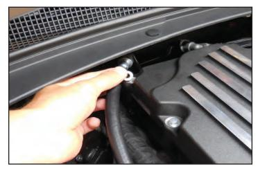
115. Install a provided Adel clamp at the corner lid location and secure with an M6x30mm bolt.
