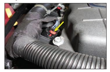
30. Remove the supercharger belt by rotating the tensioner shown with the arrow in a counter-clockwise direction using a short 15mm socket and a serpentine belt wrench. This belt will not be reused.
