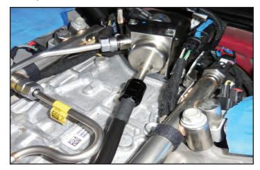
62. Tighten the fuel line securely with wrenches.
