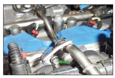
56. Place rags in the manifold valley under the fuel line. Repeat the process of removing the safety clip and disconnect the fuel line using the provided plastic fuel line tool. Remove this fuel line. It will be replaced with a provided fuel line in the next step.
