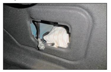
6. Place a rag over the rear hatch latch to prevent locking.
