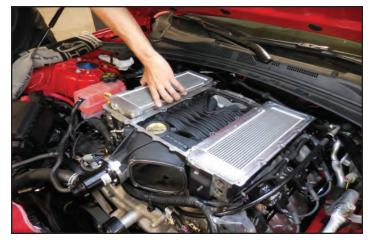
106. Gather the coolant manifolds shown that were removed earlier. Relube all the O-rings with the provided Lubriplate grease prior to reinstalling the coolant manifolds.
