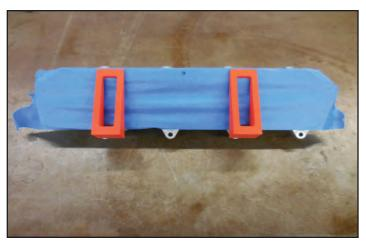
76. Ensure that the wedges sit flat against the bottom of the valve covers, and that they contact the band saw table and guide fence as shown here.
