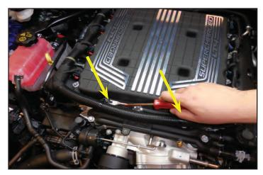
28. Remove the four cable tie connections shown with arrows using a pry tool.
