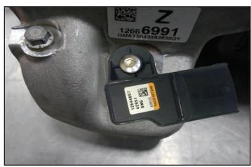
87. Remove the bolt from the location shown here on the new supercharger. This is where the MAP sensor from the previous step will be installed. Apply a light coat of supplied Lubriplate grease to the bore shown with an arrow.
