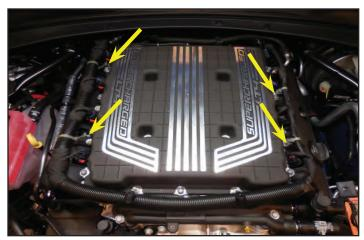
29. Disconnect the 8 coil connections by first pulling back on the red tab, and then unplugging them. You can see one of these connections here shown with an arrow.
