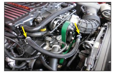
157. Remove the bypass solenoid from the OEM supercharger. Install the two provided rubber caps shown with arrows.
