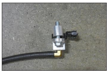
127. Install the MAP sensor bracket assembly at the bolt location that was removed earlier using the supplied M8x45mm bolt and spacer from the last step. Route the hose under the inlet as shown here highlighted in green. Reattach the anchor for the electrical connection to the bracket that was removed earlier using a supplied cable tie.
