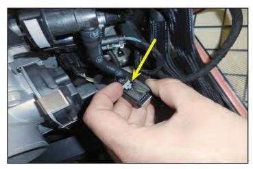
16. Disconnect the brake booster hose connection shown with an arrow. There is a gray release button that must be pressed first prior to removal.
