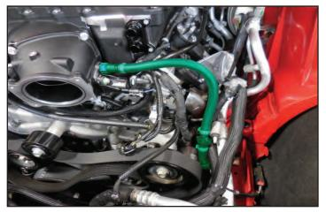
133. Place the EVAP solenoid in the location shown with the yellow arrow. Use the original bolt to secure the EVAP solenoid, and torque it in place to 108 in-lbs. Reinstall the EVAP hose (highlighted in green) and the electrical connection to the EVAP solenoid. Press in on the locating tab once the electrical plug is in place. Ensure that the electrical connection is secure.
