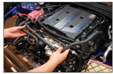
27. Remove the two cable tie connections from the front of the supercharger using a pry tool. The second connection is hidden behind the hand in this photo.
