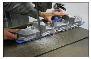
78. Once you have cut the upper coil pack mounts flush you will need to remove any sharp edges. Also thoroughly clean all the debris from the covers once you have removed the sharp edges.
