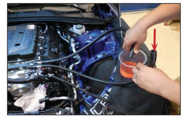
41. Seal the two connections on the supercharger side as well with plastic bags and rubber bands or plugs. Remove the front MAP sensor shown at the arrow location. This sensor will be installed in a new location in a later step using this OEM fastener.
