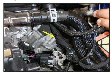
34. Here you can see a pry bar being used to remove the cable tie connection shown in the last step.
