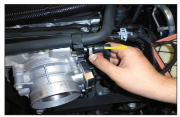
17. Pull up on the connection shown with the hose assembly to release it from the PCV air fitting.
