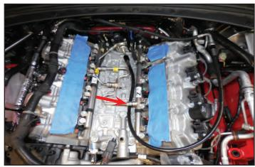
59. Remove the securing slotted nut from the female hose end.
