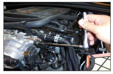
21. Unplug the MAP sensor by first releasing the locking tab, and then pull it loose.
