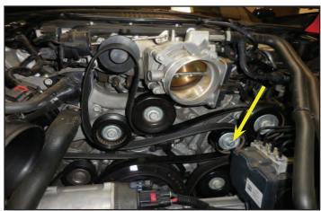
31. Here you can see the serpentine belt wrench attached to the tensioner. Rotate it counterclockwise to release the belt tension and pull the belt off the pulleys. The belt will not be reused.
