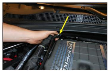
23. Disconnect the opposite side of the EVAP hose that was shown in the last photo and remove this hose from the vehicle. It will not be reused.
