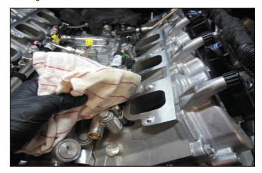
98. Have someone help you support the supercharger from the opposite side while installing. Carefully place the supercharger on the inlets for the heads. Leave enough space at the back to allow the installation of the rear MAP sensor connection.
