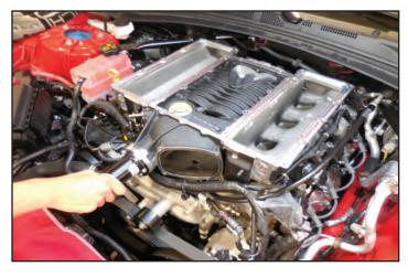
104. Locate the six M5x12mm button head bolts that held the charge air coolers in place. Apply the provided Loctite 242 on the ends of each bolt.
