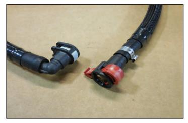
113. Connect the straight fitting from the last step to the hardline at the back of the supercharger. Secure the end by closing the red plastic clamp.
