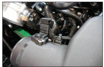
149. Secure the intercooler lines at the green highlighted location shown with an arrow with a provided cable tie. Do not crush the hose.
