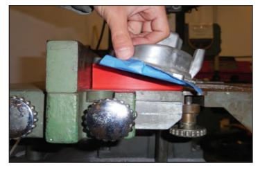
77. Cut each of the top coil pack mounts flush with the valve cover. You will have to stop the saw to reposition the wedges for each cut.
