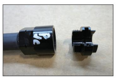
60. Slide the slotted nut that was removed in the last step over the flange on the male fuel fitting as shown with the arrow.
