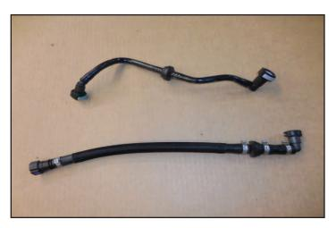
132. Install the provided brake booster hose assembly in the location shown. This hose has been highlighted in green for clarity.
