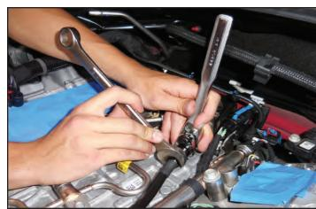
63. Connect the male fuel line connector to the female connector on the supply line. Ensure that it is fully engaged by pulling on it to verify that it is secure.
