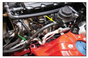
146. Use a belt tensioning wrench, or other suitable socket and wrench to provide slack in the belt to install it according to the routing diagram given at the back of this manual. Rotate the supercharger tensioner counterclockwise to provide slack at the yellow arrow location. It is easiest to install the last portion of the belt at the smooth idler shown with the blue arrow.
