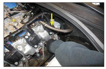
69. Once you have removed all the coil packs you can remove the valve covers. These will be modified in the next steps.
