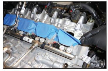
97. Wipe down the intake port outer sealing surfaces with a rag coated with Tri-flow. Pull the coil harnesses to the sides to make clearance for supercharger installation. Ensure that there are no tools or other items left in the valley area before you install the supercharger.
