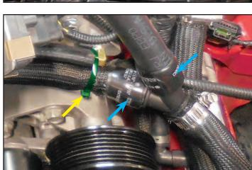
139. Cut the hose going to the OEM intercooler radiator (highlighted in green) to fit at the "Y" connector. Secure it with the provided worm gear clamp shown at the yellow arrow location.
