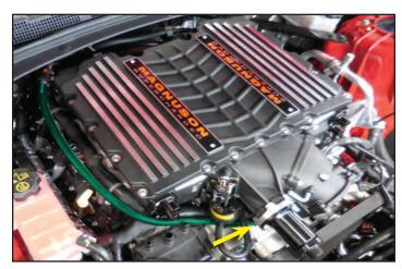
120. Here is a front view of the EVAP hose that was shown in the last step. Again the 90° fitting will be connected later.
