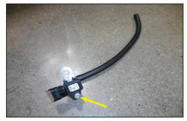
126. Install the supplied M8x45mm bolt and spacer shown to the front MAP sensor mounting bracket assembly from the last step.
