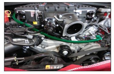
121. Apply Loctite 242 to the provided three M6x25mm bolts and both sides of the provided stud.
