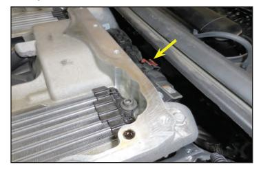
46. Remove the 10 bolts shown with arrows holding the supercharger housing in place. These bolts will not be reused.
