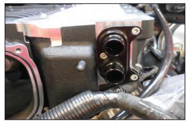
109. Apply Loctite 242 to the 19 M6x20mm bolts that were removed from the lid and 4 more M6x30mm bolts that were provided and reinstall the lid. The four M6x30mm bolts are for the center locations on the lid.
