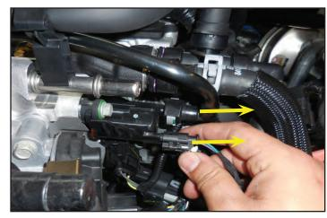
19. Here is a close-up of the electrical connection on the EVAP solenoid with the locking tab.
