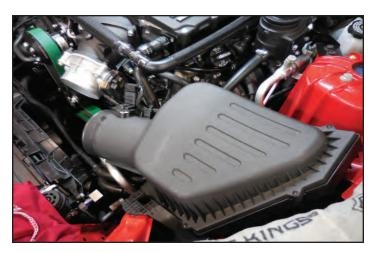
148. Plug in the MAF connector at the airbox lid.
