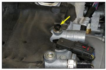
51. Apply blue tape over the ports to prevent anything from entering the engine. Remove the insulation from the manifold valley shown with an arrow. This insulation will not be reused.
