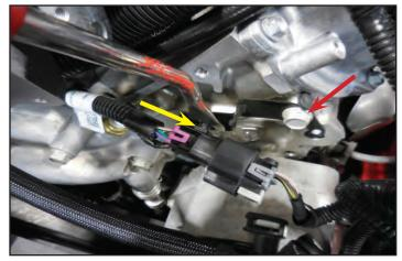
125. Gather the following supplied front MAP sensor bracket assembly and 5/16" diameter hose. Press the 20"x5/16" hose on the brass barb. This assembly will allow you to reroute the front MAP sensor into a new location. Remove the MAP sensor from the front of the OEM supercharger and install it to the adaptor using the OEM bolt in the location shown with an arrow.
