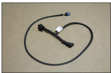
95. Pre-install the IAT sensor wire to the supercharger prior to installation. Be careful with the wire assembly while you are installing the supercharger.
