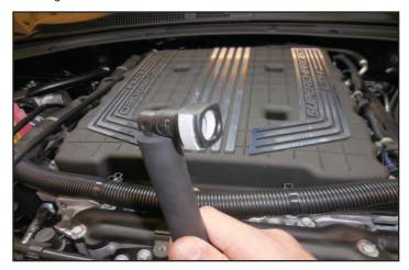
10. Pull out on the red locking mechanism from the MAF sensor connector. Then remove the connector. You can see the locking mechanism in this photo.
