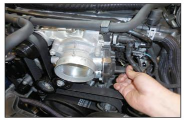
15. Here is a photo of the connection from the last step shown from the underside so you can see the locking tab.
