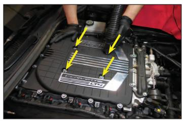
44. Remove all 20 bolts holding the lid in place. Then remove the lid.
