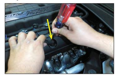
26. Now you can remove the PCV hose assembly shown. The smaller hose will be replaced with a provided one in a future step. The larger hose will be reused.
