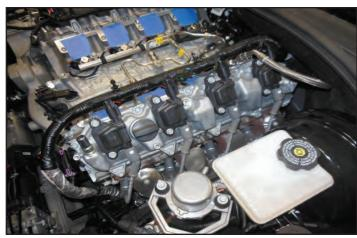
68. Disconnect the spark plug wires from all the coils. Disconnect the electrical connector on top of the coils. Remove the two screws securing the coils using a 10 mm socket. Set the coils aside for reinstallation later.
