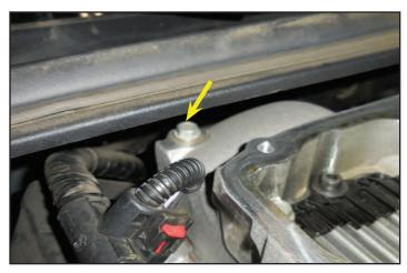
48. Here is the other hidden bolt on the left rear of the supercharger.
