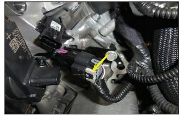
33. Use a pry bar to remove the cable tie connection shown with the arrow.
