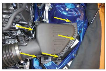
8. Loosen the two hose clamps for the intake duct using an 8mm nut driver or standard screwdriver. Also at this time remove the PCV hose shown at the green arrow location by pressing inwards on the gray buttons and pulling it out.
