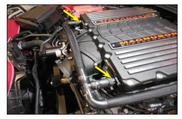
142. Gather the provided reservoir and install it to the provided bracket using the 3 bolts that came attached to the reservoir.
