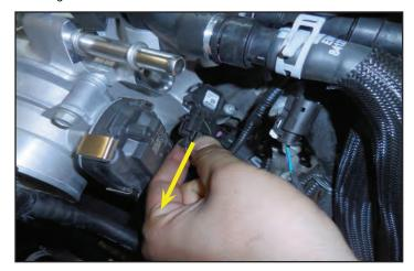
22. Disconnect the EVAP hose shown at the right rear of the OEM supercharger.
