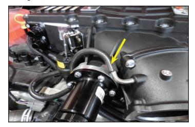
130. Unplug the other end of the brake booster hose assembly shown here highlighted in green at the arrow location. You can see a better image of this hose assembly in the next step.
