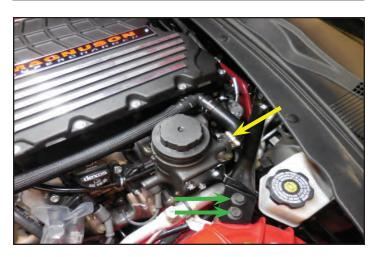
144. Cut a 9" hose section from the material that was left over after cutting the 4"x36" 90° hose. This will be used to connect the reservoir output to the OEM intercooler pump inlet along with the 3/4" hose mender, shrink clamp, and two worm gear clamps. These items will be used in the next step. Connect one end of the 9" hose to the 3/4" hose mender and secure with the shrink clamp. Again make sure the connection is tight after heating the clamp by pulling on it.
