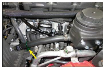
151. Install the provided rubber air duct. Use the two provided hose clamps to tighten the air duct in place. Ensure that the duct lines up with the notches in the air box and the throttle body shown with the blue arrows.
