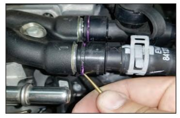
37. Here is one of the two clips that was removed in the last step. These will not be used again.
