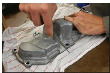
79. Remove the masking tape. Clean out the debris using a solvent cleaning tank. Ensure that the covers are thoroughly clean and dry before installing them on the heads. Re-install the gaskets on both valve covers.
