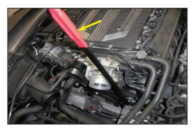
32. Remove the connection shown with the arrow by first releasing the white tab, and then unplugging the connector.
