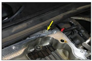
49. At this point you will need some help to remove the supercharger from the engine. Have at least one other person on the opposite side of the engine bay while you lift it up. Carefully clean up the surface around the intake ports. Use isopropyl alcohol to clean the surface around the ports. Make sure nothing enters the intake ports.
