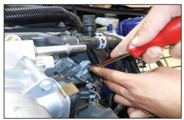
35. Place a cup under the intercooler connections as shown to collect the coolant that will be drained in the next few steps.
