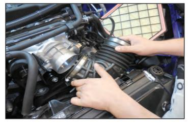
13. Remove the lower part of the airbox by pulling up on it. It has three barbed pins that connect to rubber grommets.
