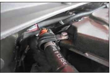
116. Torque the 23 bolts lid bolts to 106in-lbs following the order for the lid given at the back of this manual.
