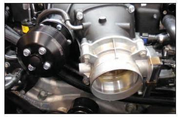
135. Plug in the electronic throttle control and ensure that the lock is engaged.
