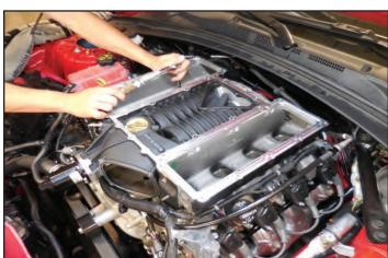
103. Ensure that the supercharger pulley still spins freely after full torque is applied.
