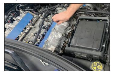
70. Remove the gaskets from the two valve covers.
