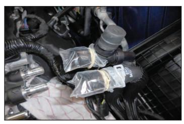
40. In order to drain more coolant from the supercharger you can install some hoses at the connections you just unplugged. Then place one hose in the drain cup while you pressurize the other hose. This should clear the majority of coolant out of the supercharger.
