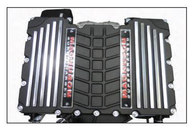
92. Remove the 3 bolts holding the coolant manifold assembly at the front of the supercharger and pull the spigot out. Repeat this process on the other coolant manifold assembly.
