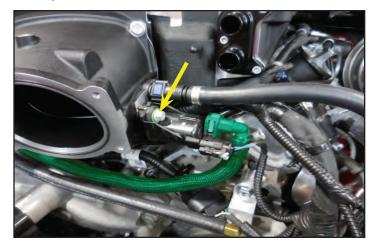
134. Install the throttle body using the OEM bolts and torque them to 108 in-lbs. Install the pulley with the provided M6x16mm bolts and torque them to 108 in-lbs.
