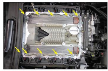
47. Two of the bolts from the last step are hidden below the cowl. This is on the right rear of the supercharger.
