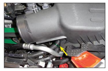
150. Secure the intercooler lines at the green highlighted location shown with an arrow with a provided cable tie with. Do not crush the hose.
