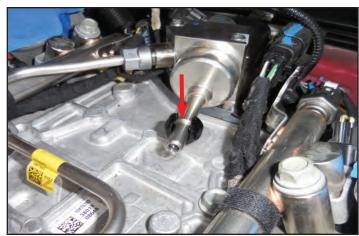
61. Hand tighten the slotted nut onto the female fuel line. You may have to bend the hose slightly with your hands at the end to thread the nut.
