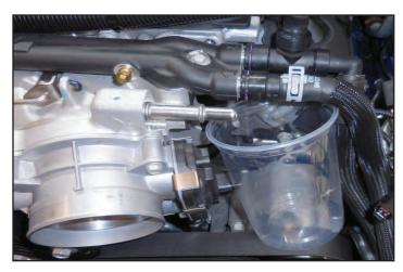
36. Use a pick or other appropriate tool to remove the two clips that secure the connections for the intercooler hoses.
