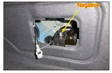
5. Place a rag, or other appropriate insulator over the negative terminal to prevent accidental connection.
