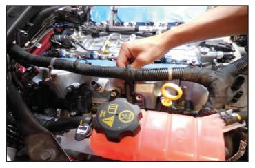
85. Use a provided Adel clamp to secure the fuel line at the arrow location.
