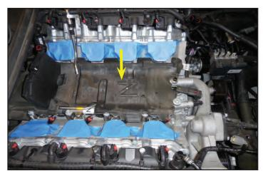
52. Vacuum out the manifold valley to remove any debris.
