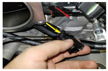
129. Install the opposite end of the hose from the last step to the air tube shown with the arrow. This hose will wrap around the supercharger inlet. Ensure that the hose does not interfere with the belt line.
