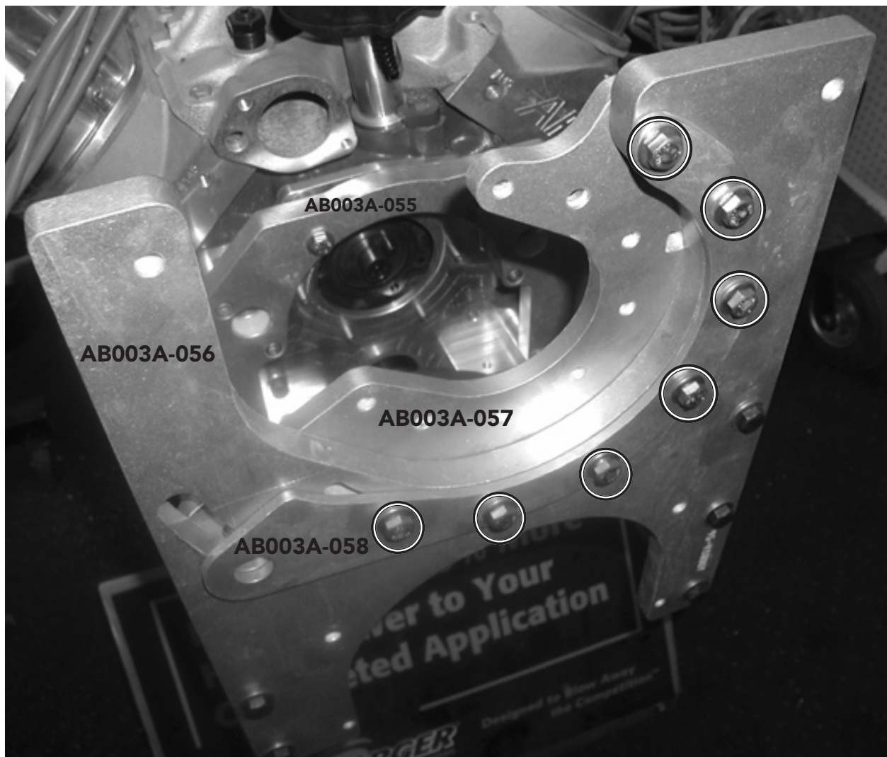
Swivel Plate & Washer Plate Installed
